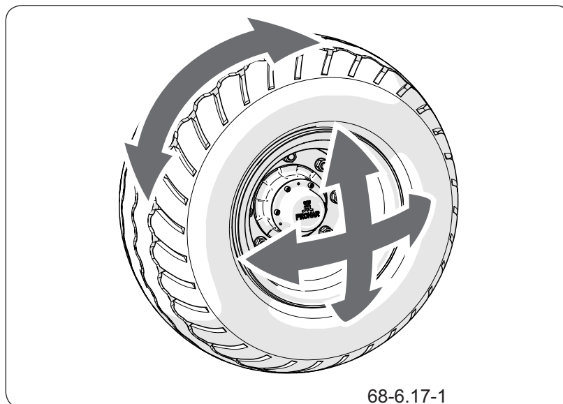
Figure 6.6 Check wheel half axle bearings looseness
