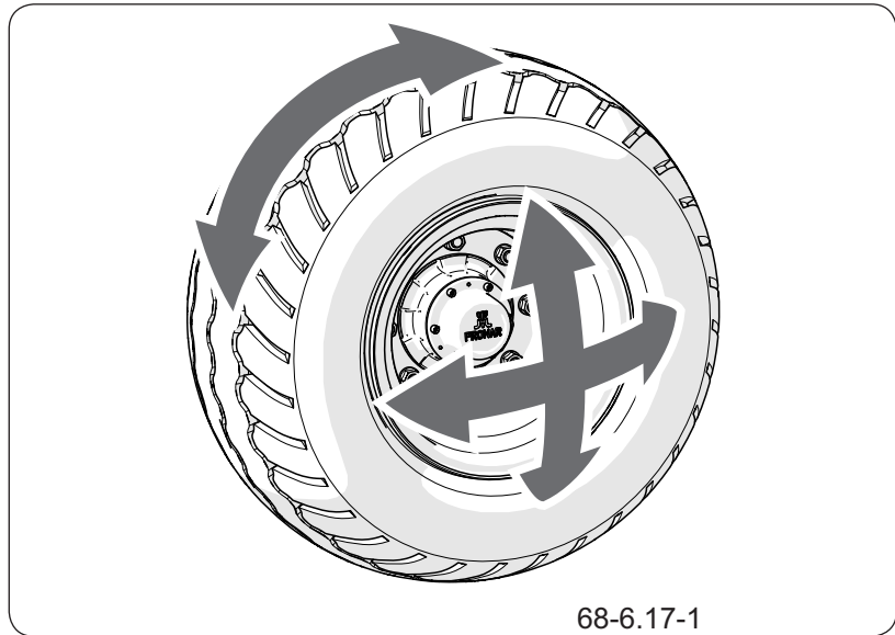
Figure 6.6 Check wheel half axle bearings looseness
