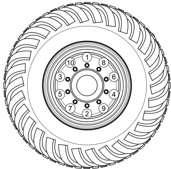
FIGURE 5.4 Sequence of undoing and tightening nuts
