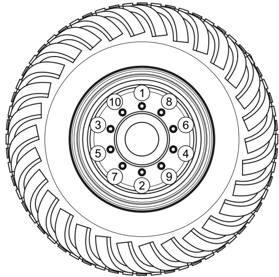
FIGURE 5.4 Sequence of undoing and tightening nuts
