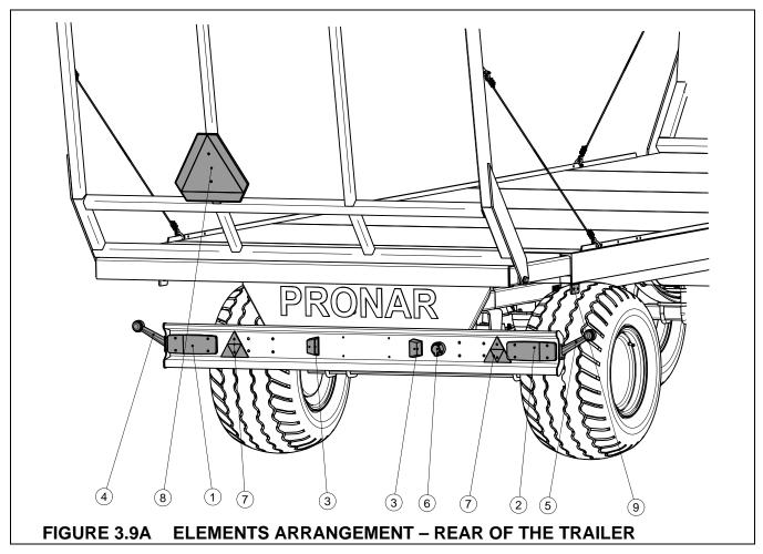
(1) left rear complex lamp, (2) right rear complex lamp, (3) registration plate illumination lamp, (4) left rear contour lamp, (5) right rear contour lamp, (6) rear socket, (7) warning reflective triangle, (8) "Low Speed Vehicle" plate, (9) orange side contour lamp
