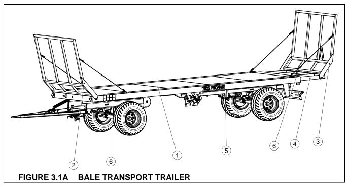
(1) frame – load platform, (2) front ladder, (3) rear ladder, (4) extendable frame, (5) parking brake mechanism, (6) protective steel cable
