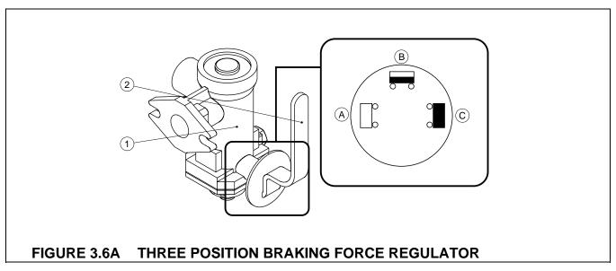
(1) braking force regulator, (2) lever, (a) "no load" (b) "half load, (c) "full load"
