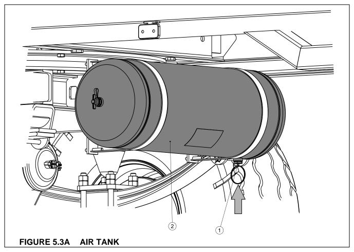
(1) drain valve, (2) air tank
