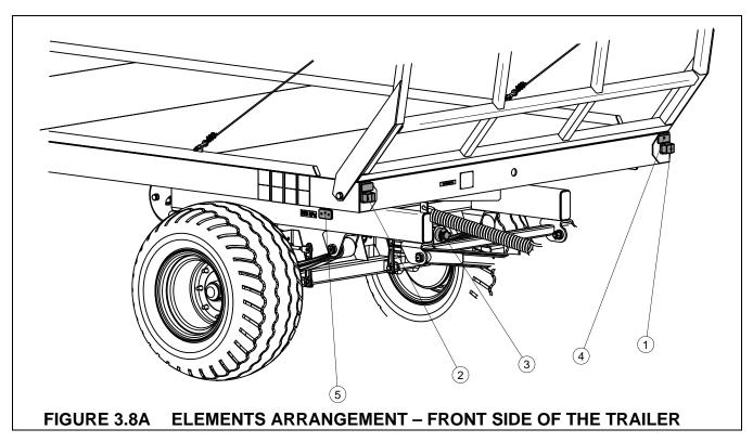
(1) front left head lamp, (2) front right head lamp, (3) front socket, (4) white reflective lamp, (5) orange contour lamp
