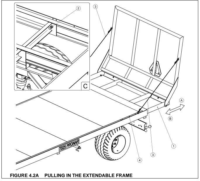
(1) extendable frame, (2) locking bolts, (3) steel cable, (4) steel cable fixing holes
