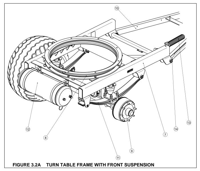
(7) Turn-table frame, (8) turn- table, (9) traction axle, (10) shaft, (11) parabolic spring, (12) air tank, (13) spring, (14) shaft pivot
