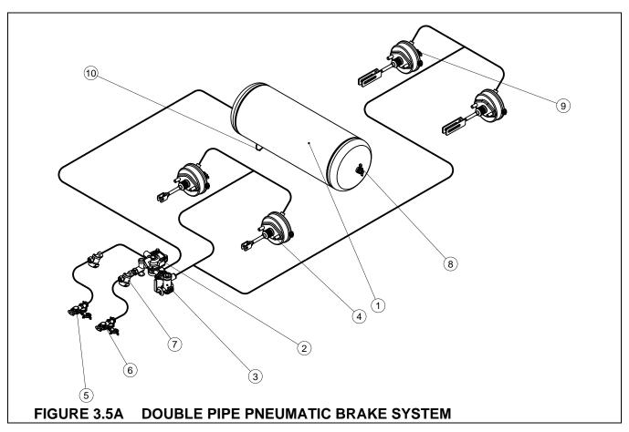
(1) air tank, (2) control valve, (3) braking force regulator, (4) pneumatic actuator, (5) red pipe connection, (6) yellow pipe connection, (7) air filter, (8) air tank control connection (9) actuator control connection, (10) drain valve
