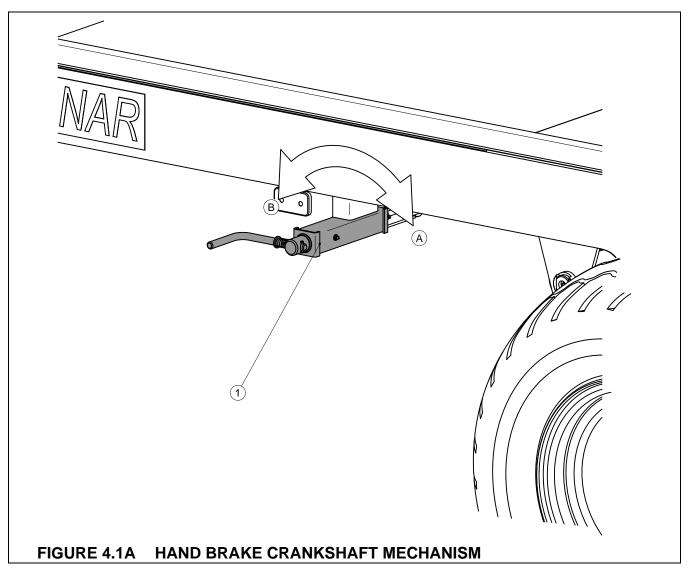
(1) crankshaft mechanism, (A), (B) turning direction of the mechanism
