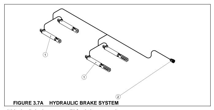
(1) hydraulic brake actuator, (2) feed pipe connection
