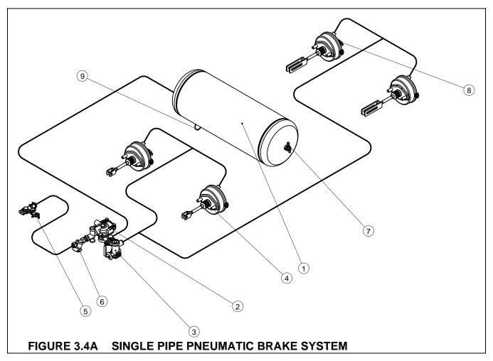
(1) air tank, (2) control valve, (3) braking force regulator, (4) pneumatic actuator, (5) connection, (6) air filter, (7) air tank control connection, (8) actuator control connection, (9) drain valve
