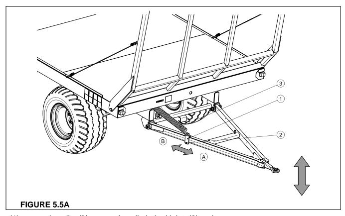
(1) connection clip, (2) connection clip bolted joint, (3) spring
