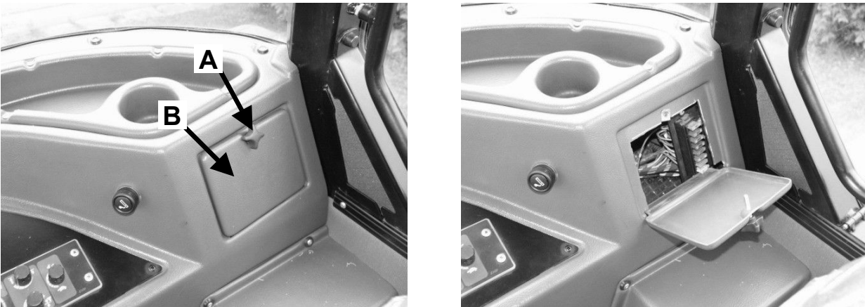
Fig. E-54 Location of fuse set FB3 on the right wheelarch. A- screw; B- cover
