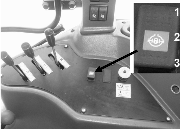
Fig. D-16 Controlling of the rear axle differential gear lock (at the switches panel on the right side of the seat)
