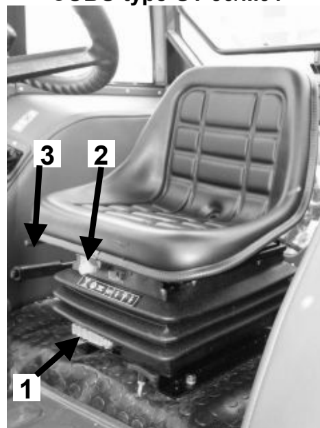
Fig. C-22 Operator seat 1-shock absorption adjustment knob (depending on operator's weight); 2-vertical adjustment; 3- horizontal adjustment.
