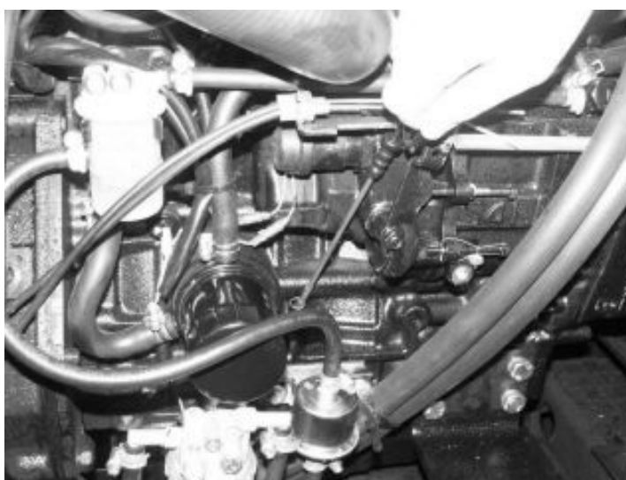
Fig. E-5 Engine oil dipstick, situated on the right side of the tractor. Oil level should stand between notches L and H.
