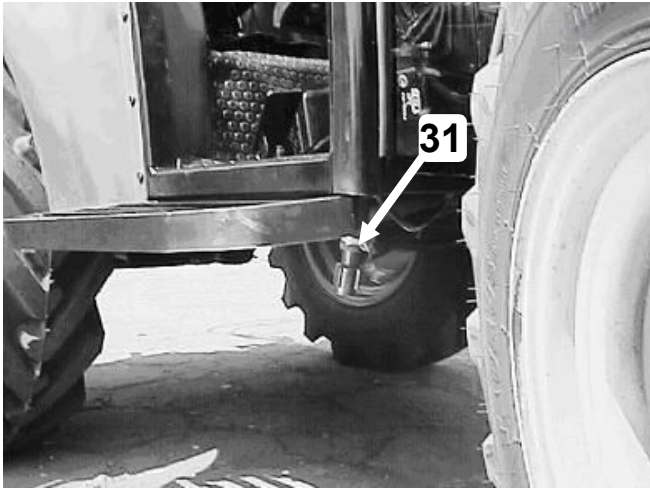
Fig. E-25 Cab heater drain plug (31)- 2 pcs on both sides of the cab
