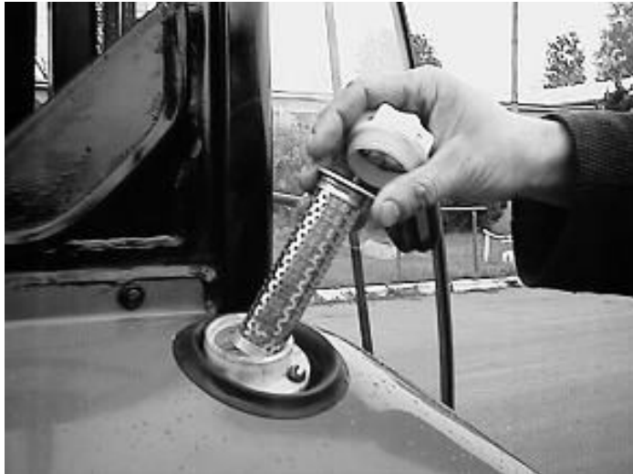
Fig. E-18 Filling plug of the hydraulic & steering system + filling filter.
