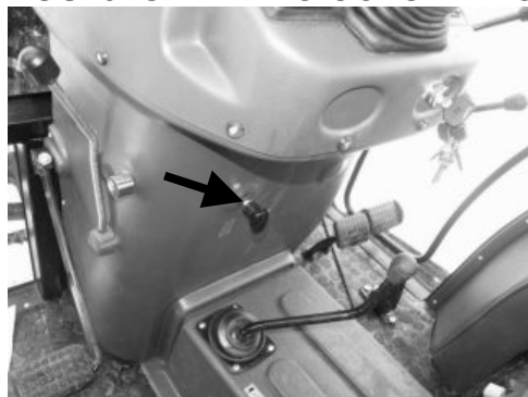
Fig. C-15 Steering column position clutch cable.
