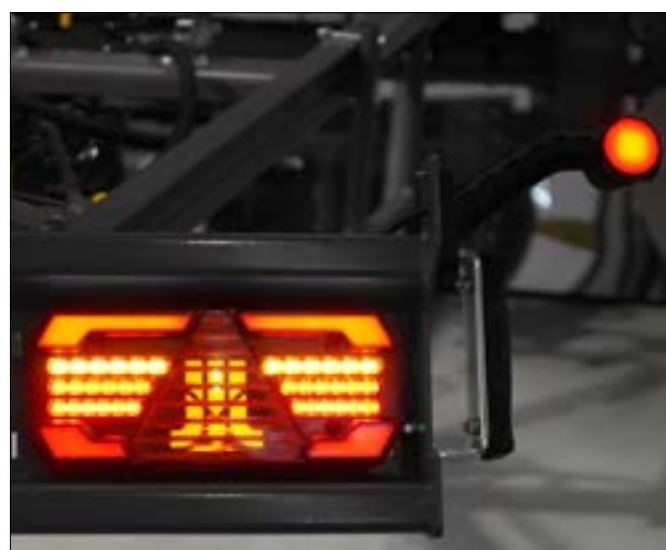
Installation d'éclairage 12V LED (standard)
