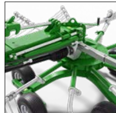
● hydraulic adjustment raking width
