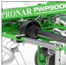
● spring shock absorber, stabilizing the machine
