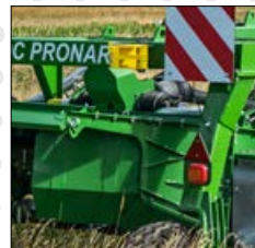
metal swath guides (PDC300C)
