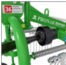
● active suspension with stabilizers shock-absorbing (optional)
