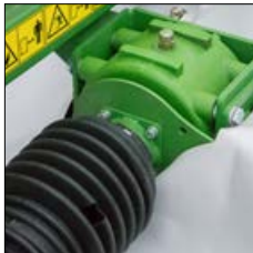
• drive - 3 angular gearboxes
