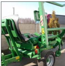
● loading system - side bale grab
