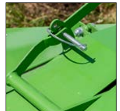
4-stage regulation for conditioner pressure
