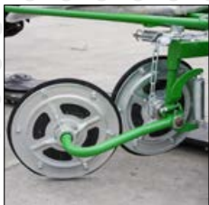
● double galvanized swath guides (PDT260 - option)
