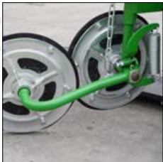
• double galvanized swath guides
