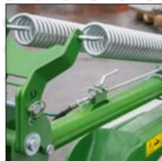
● 3 stage mechanical relief adjustment
