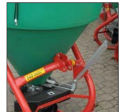
• dose adjustment lever and sowing direction
