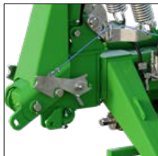
bump stop for lifting over swaths
