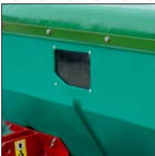
● inspection holes in twin-chamber tank
