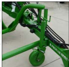
● drawbar support with foldable steel wheel
