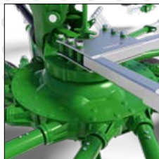
● carousel gearbox - greased
