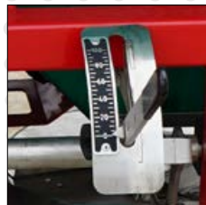
● dose adjustment lever and sowing direction
