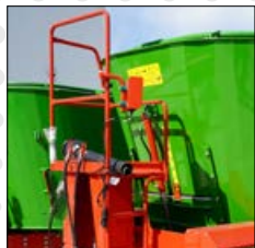
● platform with steps and a protective barrier
