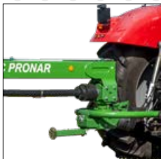
● adapted to the 540 and 1000 rpm drive
