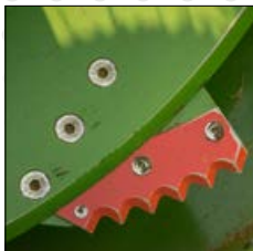
● cutting knife (possibility to set in 2 positions)
