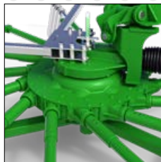
• carousel gearbox - greased
