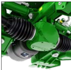
• drive - 3 angular gearboxes
