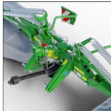
• central suspension bilateral terrain copying range +18°-16°
