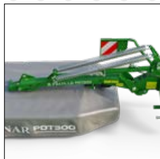
● central suspension large terrain copying range +18°/-16°
