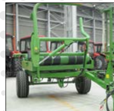
● loading system - front bale grab
