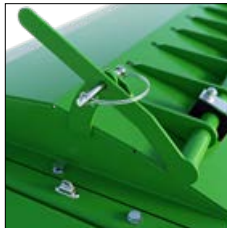
4-stage regulation for conditioner pressure
