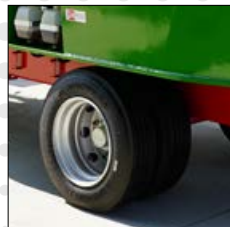
● reinforced axle on double tires
