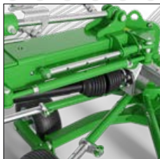
• mechanical adjustment of the raking width
