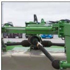
● central drawbar allows mowing to the right or left side of the tractor
