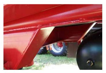
The lower frame is welded from closed steel sections made of high quality construction steel
