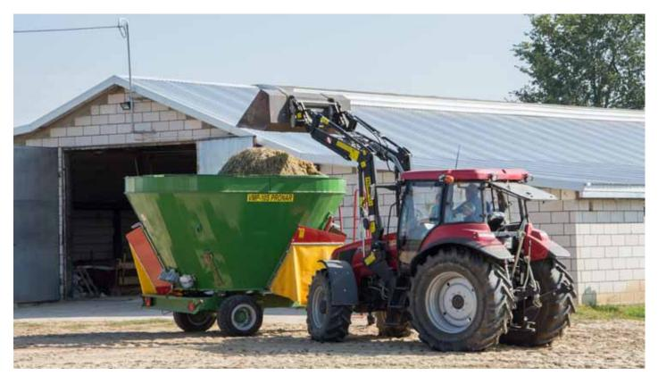
One of features PRONAR mixed feeders have is segmental construction. It allows the farmer to adapt capacity of the machine (even up to 12m<sup>3</sup>) to the size of his herd by
