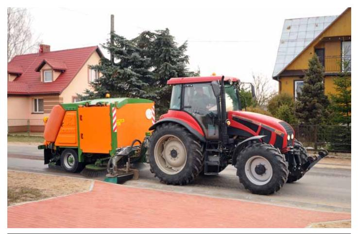
by Pronar's British dealer. The grasscovered surface was cleaned it 95% and suffered no damage after the first pass with minimal pressure set. The surface was thoroughly cleaned and otherwise left intact. Another test positively verified effectiveness of new brushes in gathering up large amounts of wet leaves, a task traditional suction sweepers have trouble dealing with.
