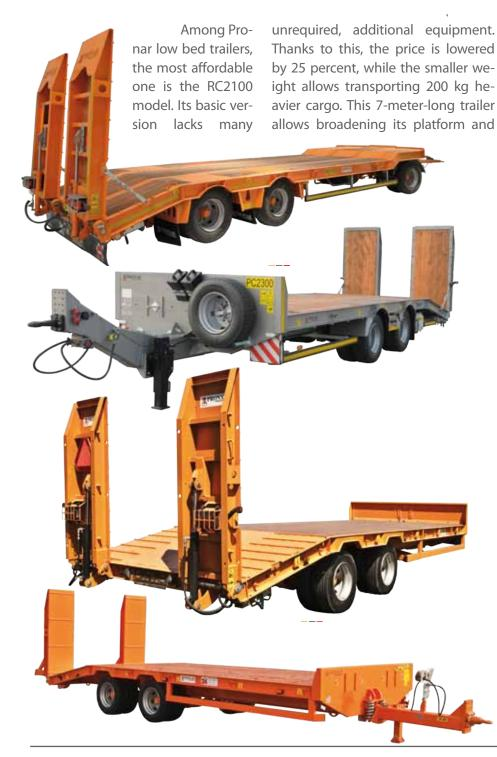
ramps by 25cm on each side to make the load width reach 3040mm. This allows transport of machines and cargo of non-standard dimensions. 1,9-meter-long ramps facilitate loading of vehicles, extend the load surface and secure the cargo.
