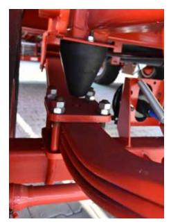
The suspension is based on parabolic springs with three leafs, narrowing towards the end. Thanks to this design they do not require any lubrication.
