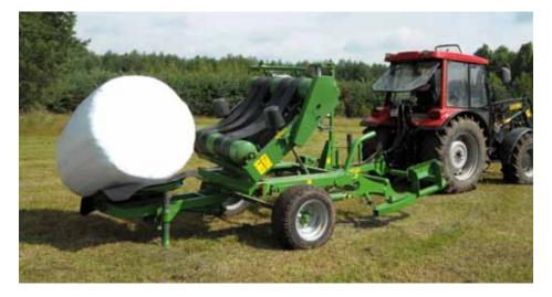
PRONAR Z245 is loaded from the side using a loading arm, while PRONAR Z245/1 is loaded from the front. Each machine counts the rotations of the turntable with a wrapping counter inside the tractor's cab. Depending on the width of the foil, it is recommended to use 24 (for 500 mm foil) or 16 (750 mm) rotations. The wrapped bale is grabbed by the adjustable unloading mechanism and set on the side of the wrapper with the flat side down or is rolled down behind the machine (depending on the model).
