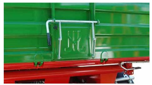
The chute is closed with two tension rods which make it easier to open and lock it.
