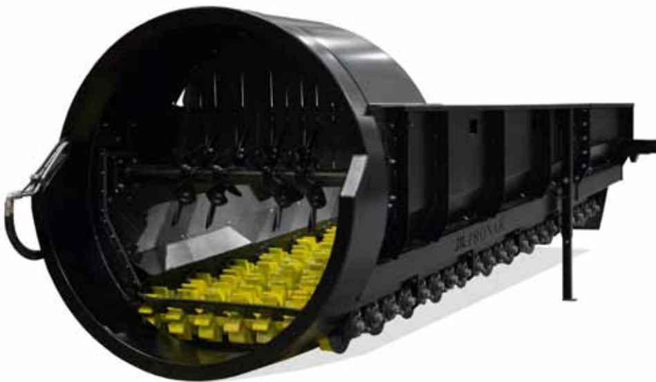
The shaft spreading the material on the star screen
