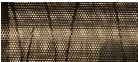
Thanks to the mesh band surrounding the drum, it is possible to make a screen with a perforation of less than 10 mm
