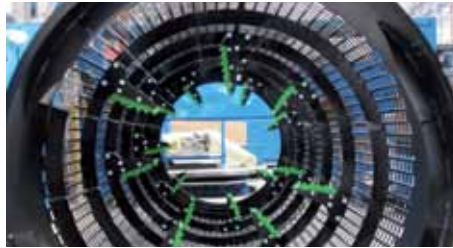
Blades to tear up bags can be mounted in all trommel screens
