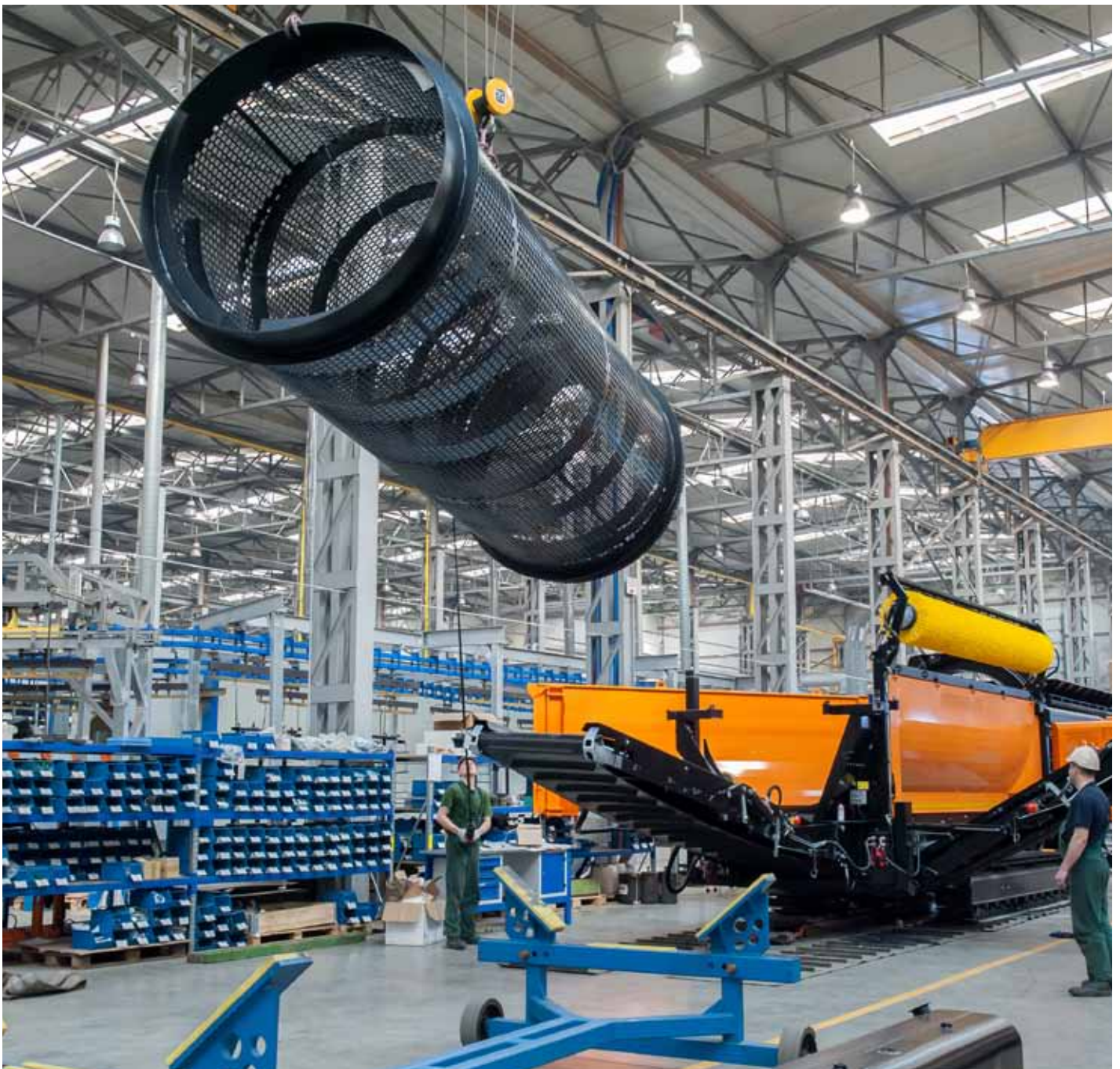
↑ One of the most important element of trommel screen is a steel drum.
