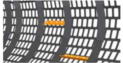
Threshold bars mounted in the trommel screen help to clean the material more effectively
