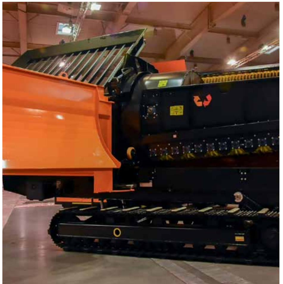
↑ Star screen mounted in the machine
