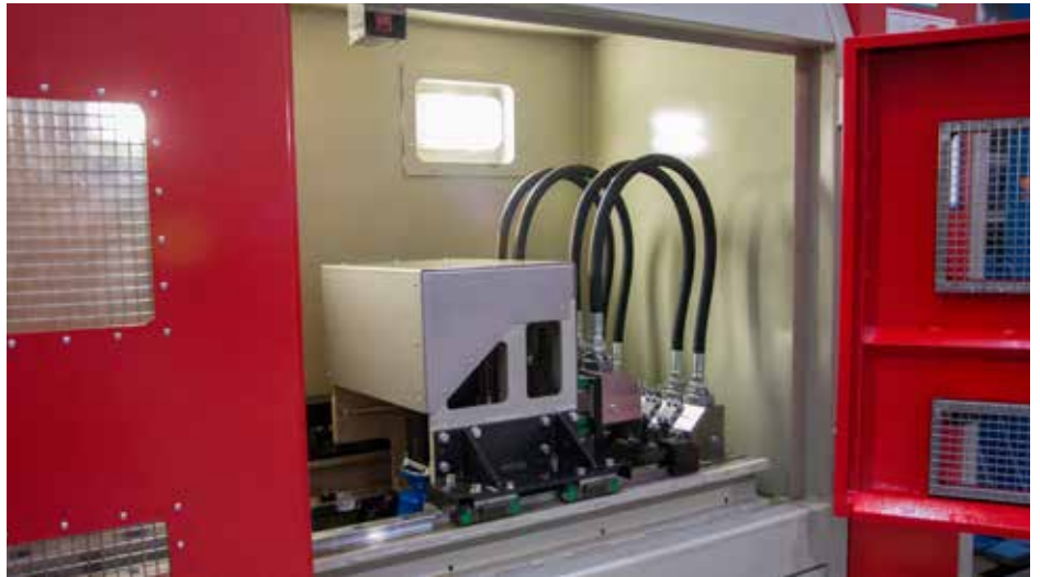
The UV chamber enables the simulation of changing weather conditions, e.g. temperature, UV radiation and humidity
