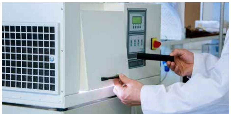
The UV chamber enables the simulation of changing weather conditions, e.g. temperature, UV radiation and humidity
