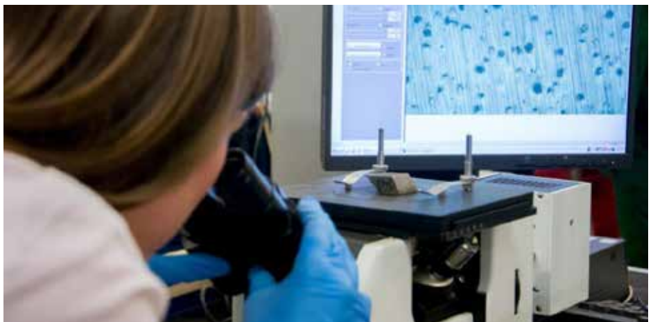
The metallographic testing station allows for testing the micro-structure of metals and their alloys, e.g. analysis of grain size, inclusions, porosity, cracks and other material flaws
