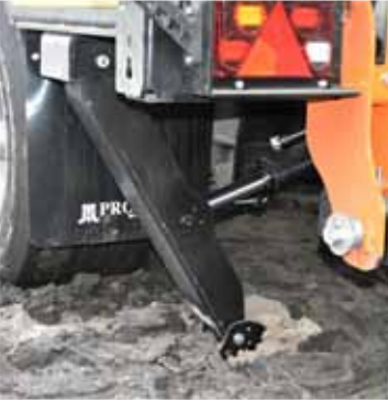
Hydraulic support legs improve machine stability during operation
