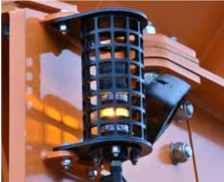
Machine operating mode status indicator - for status check and security warnings
