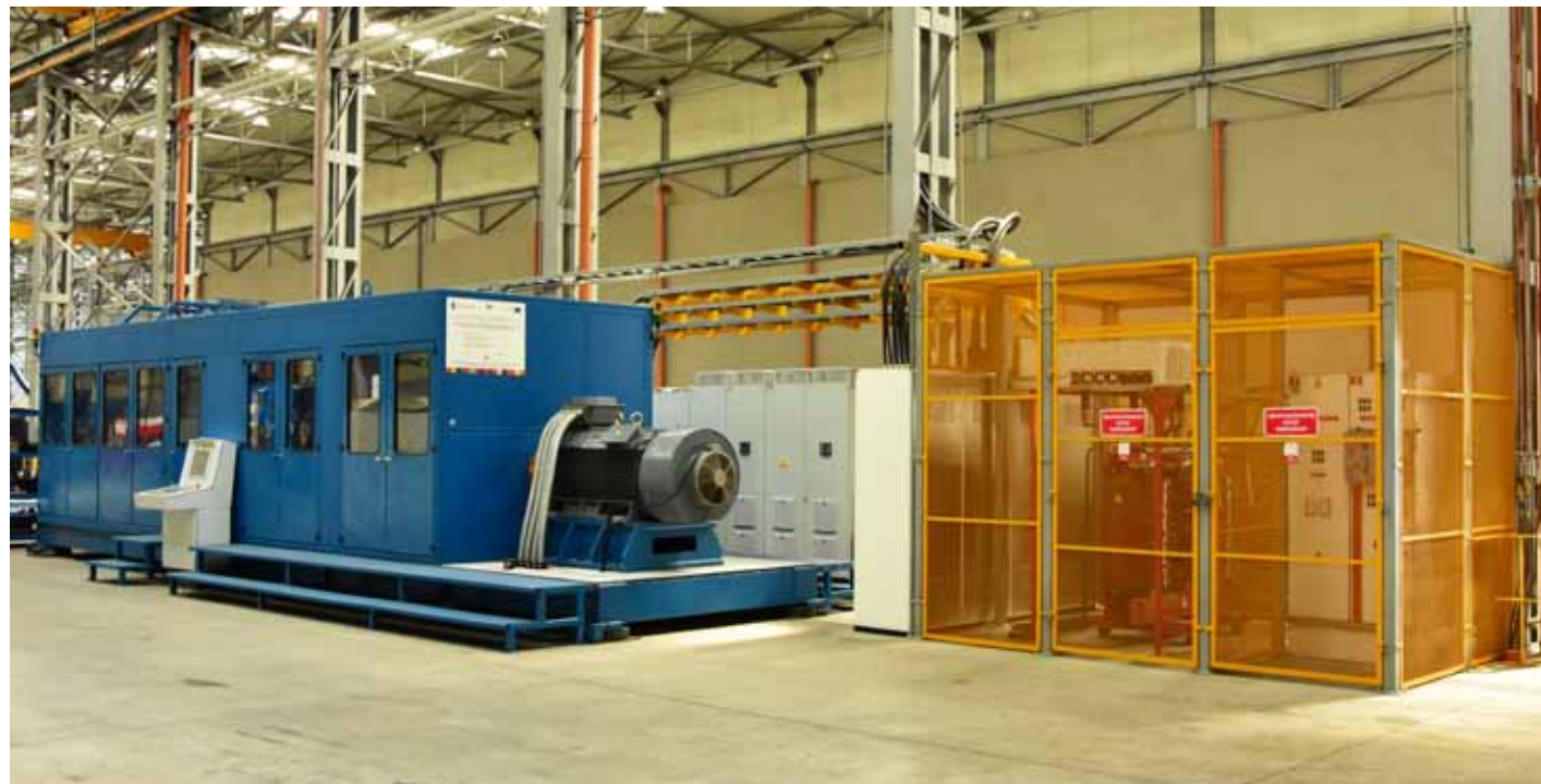
Using their own experience as well as research conducted together with external institutions, Pronar's engineers have designed a special stand for axle tests
