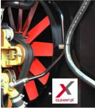
Engine cleanfix system - automatically cleans the engine radiator ensuring uninterrupted overheating issues id dusty conditions
