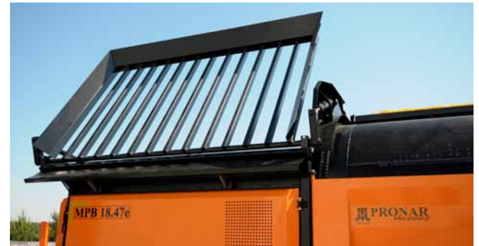
Hopper grate. This helps stop bigger pieces of debris entering the work area when screening materials with larger dimensions. The grate is not necessary when screening lighter materials (chips, etc).
