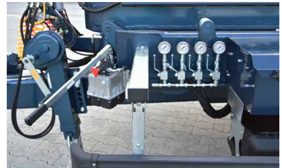
All hydraulic cylinders are controlled by a hydraulic distributor, which is in standard equipment of the trailer
