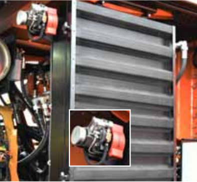
Hydraulic oil radiator cleanfix system for optimal and uninterrupted operations
