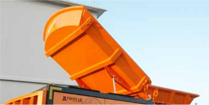
Thanks to remote control a hydraulically raised chute increases machine output and operator's work comfort
