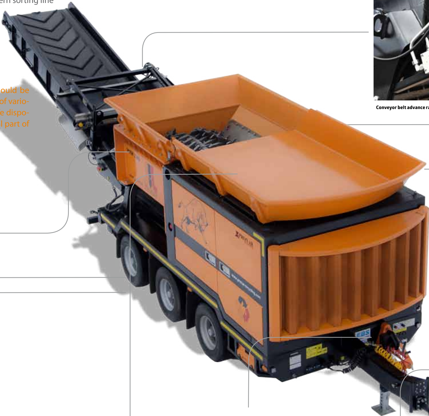
Thanks to remote control a hydraulically raised chute increases machine output and operator's work comfort
