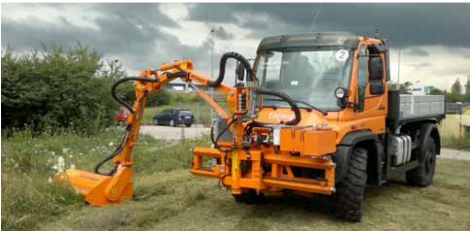
WWP500U hydraulic arms are designed for use with MB Unimog vehicles
