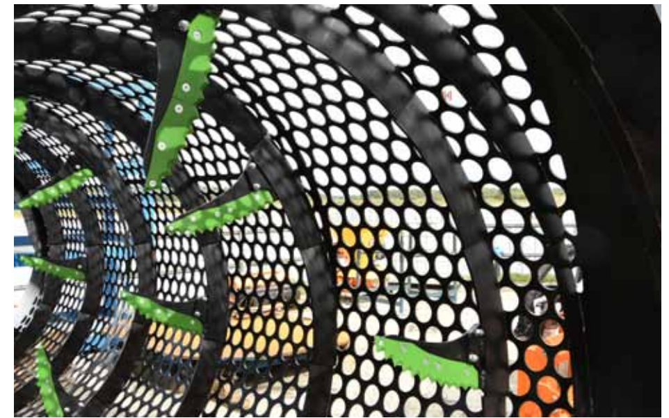
Trommel for screening municipal waste. The blades facilitate separation of plastic bags.
