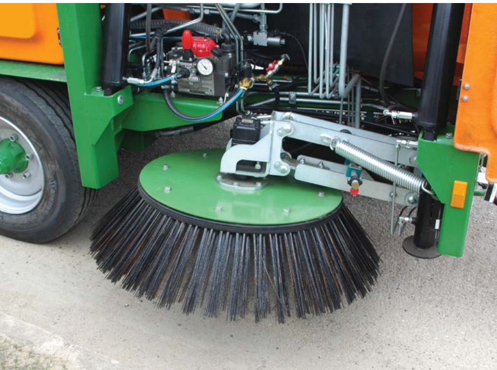
Disc brushes furnished with regulating mechanism, which is facilitated with their slope angle indicators during sweeping
