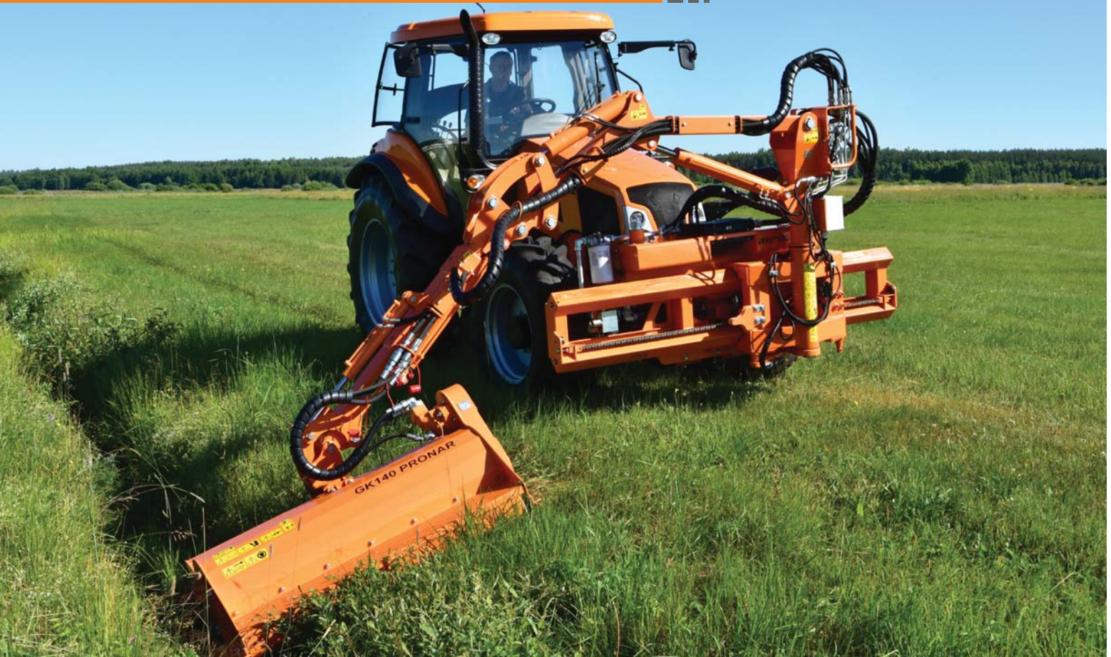
Multifunctional extension arm PRONAR WWP500 with PRONAR GK140 head mounted on a PRONAR 5340 tractor
