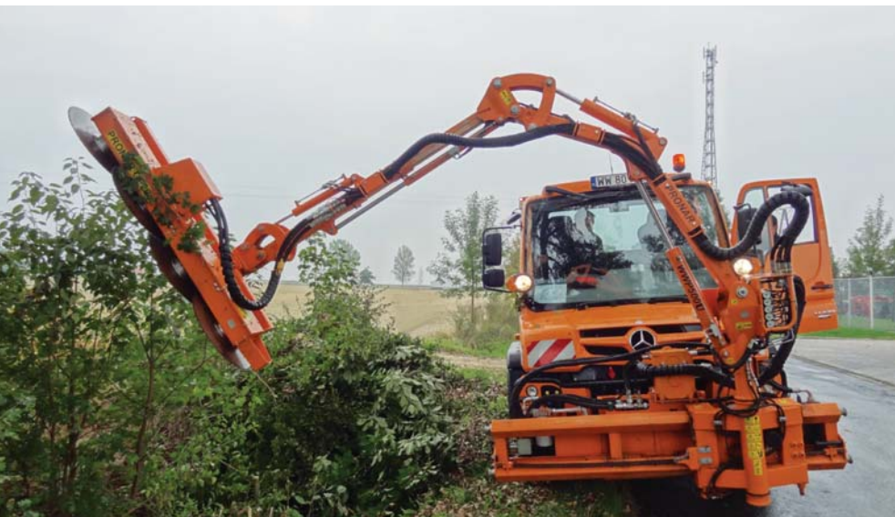
PRONAR WWP500U with the branch cutting saw PRONAR GP200 mounted on Unimog 500
