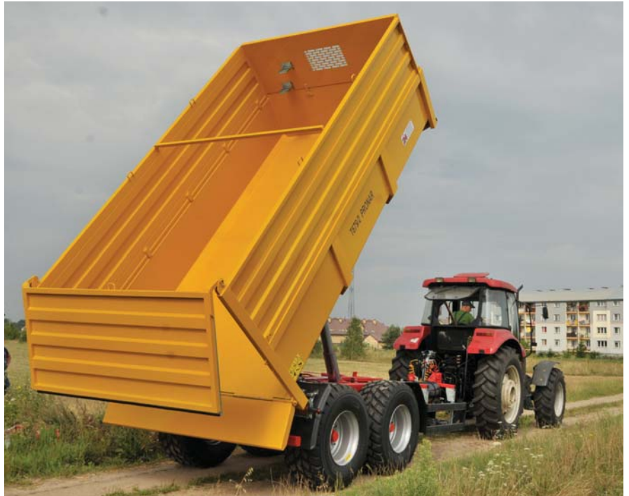
Additional superstructure increases the capacity of the trailer
