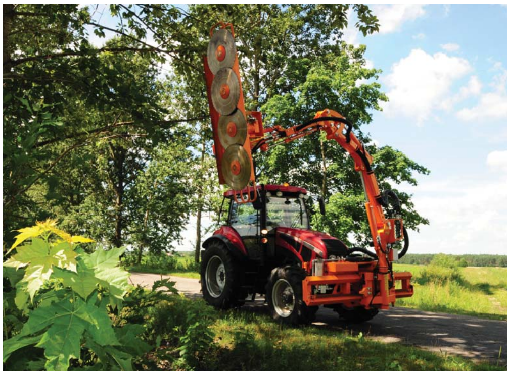
A multi-use PRONAR WWP500 extension arm with the PRONAR GP200 saw to cut hard-to-reach tree branches mounted on the PRONAR 5235 tractor
