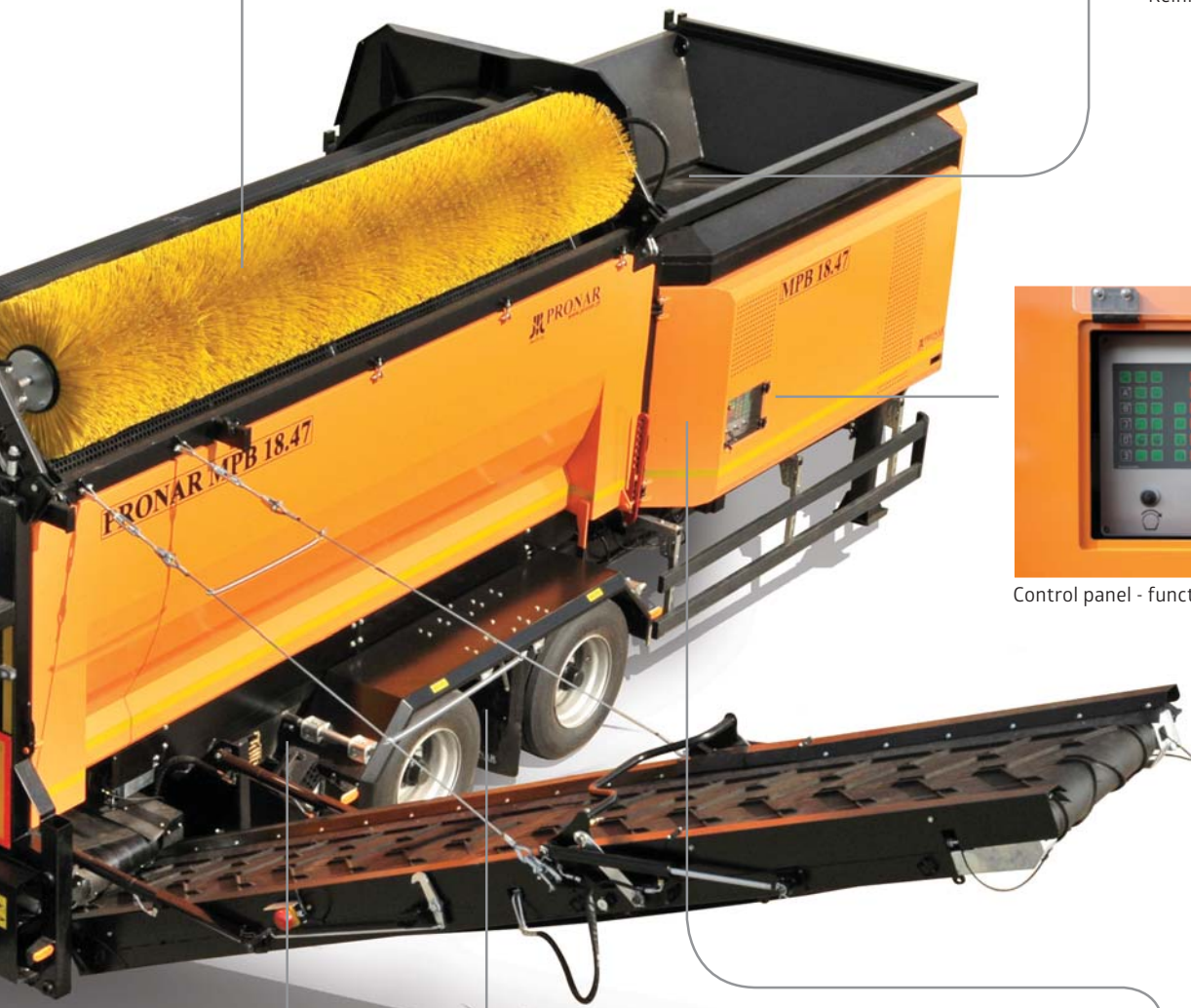
Drum cleaning brush - raised and lowered hydraulically
