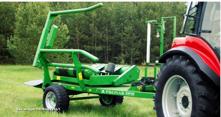
**Bale wrapper PRONAR Z245/1** has a functional system of loading arm by picking up the bale from the side (the wrapper follows the path of round baler). Loading arm allows loading a bale on the wrapping table without stopping. Standard version of bale wrapper is equipped with a hydraulic cutting mechanism what saves the time. Turntable allows unloading a bale in two ways: on its side or front surface what helps to easily load the bales onto the trailer.
