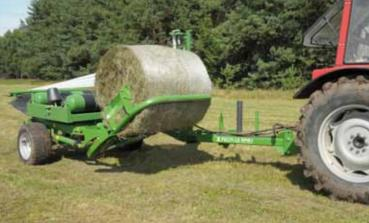
Unloading a bale either on its side or front surface
