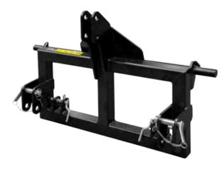
The rectangular frame is equipped on one side with a fixing eye on a three-point suspension system of the tractor. On the other side frame is equipped inholders for attaching tools for front loaders fromeuro type frame. Fastening the product to the tractor is done manually. Attaching the tool is taken from the position of the tractor operator, but bolted manually with bolts in the lower eye of the tool.
