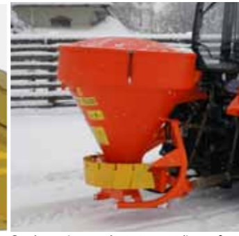
Sand container can be 250 or 500 litres of capacity
