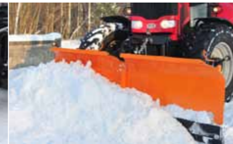
PUV 3300 working with 30 degree angle
