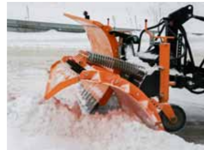
Segmented mouldboard with spring safeguard.
