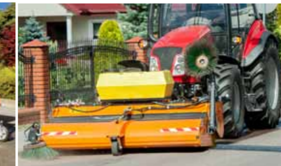
Tank with tiltable bottom allows for easy passage through e.g. speed bumps.
