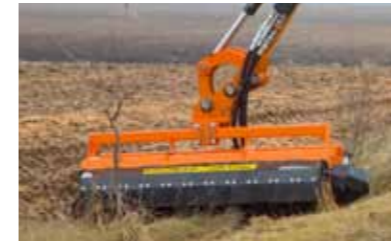
Light cutting head GK120L on arm WWT 600
