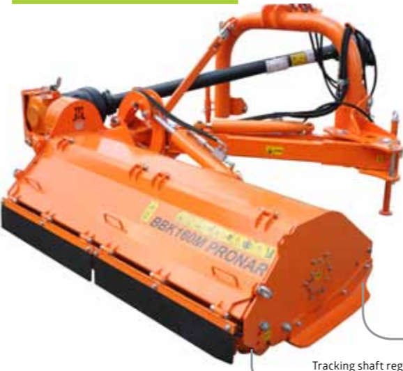
Tracking shaft regulates cutting height
