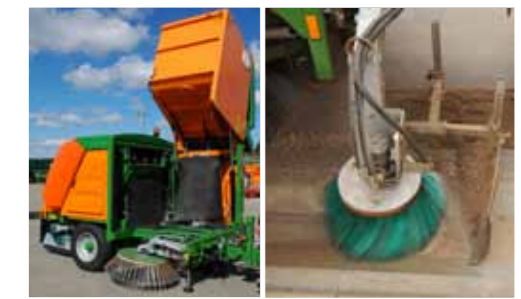
ZMC 3.0 - hydraulic hopper dumping system.
