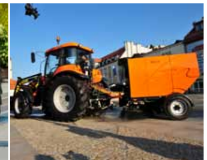
ZMC 2.0 - hydraulically articulated drawbar.
