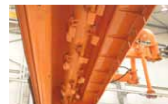
Flail shaft with flail hammers.
