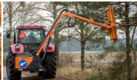
WWT700T, WWT800T - Long arm reach is provided thanks to hydraulic telescopic sliding
