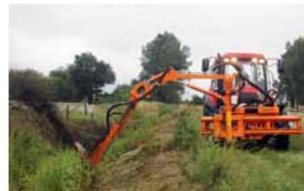
WWP600 with GO800 ditch digger. Long reach fits perfectly for desludging.
