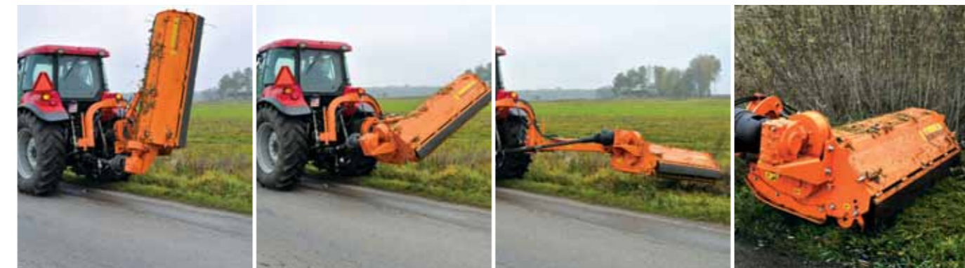
Mower works on right side of the tractor, vertical rest position
