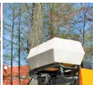
Additional water tank (200 l)
