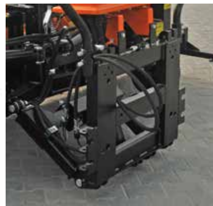
Mounting – DIN type A municipal plate
