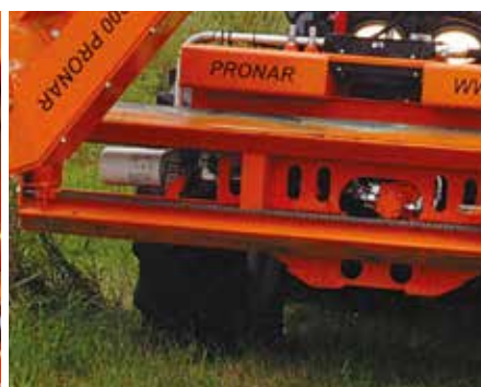
Hydraulic boom travel along the guide rail for selecting the appropriate working position
