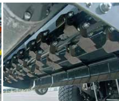
Cutting unit - cutting shaft with replaceable knives
