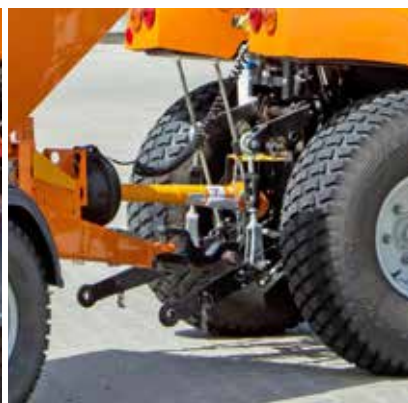
PTO drive for tractors without hydraulic system
