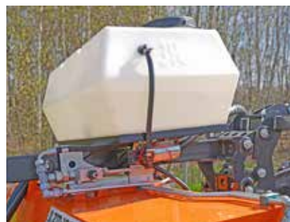
Additional water tank
