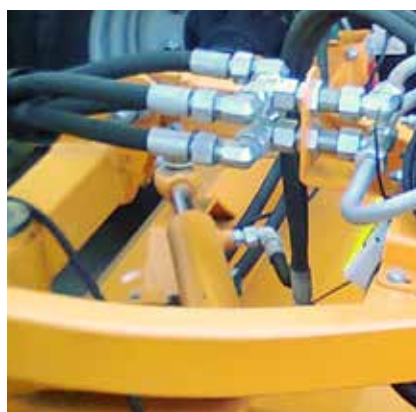
Hydraulic brush angle adjustment \pm 30^\circ
