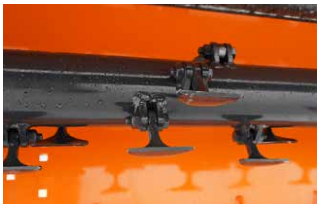
Cutting shaft with replaceable knives
