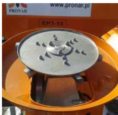
Stainless steel spreading disk
