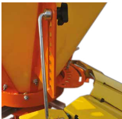
Adjustment of spreading width
