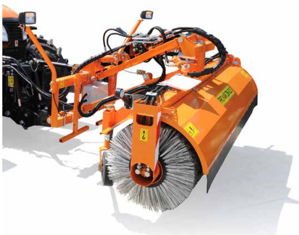
Hydraulic brush angle adjustment \pm 30^\circ
