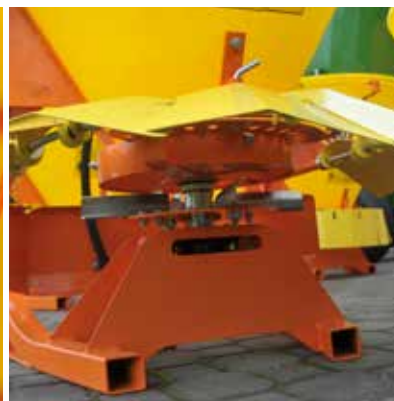
Stainless steel spreading disc
