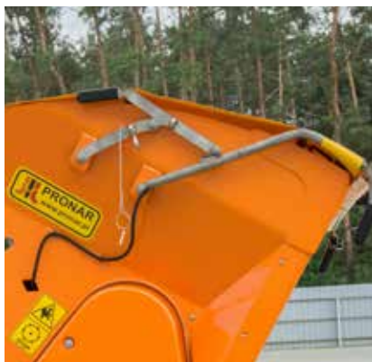
Canvas cover with frame protects the material from snow and rain
