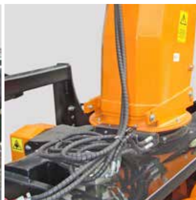
Hydraulic discharge chute rotation and adjustment of throwing distance
