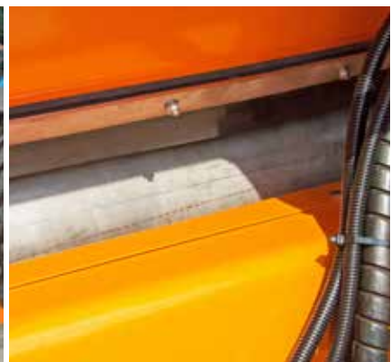
Working roller with slats dispense the material on the road
