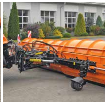
Mounting – DIN type A municipal plate
