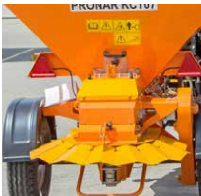
Covers for setting spreading width and limit scattering
