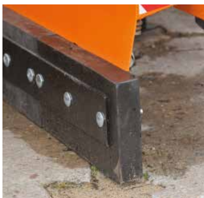
Rubber blades with shock absorption
