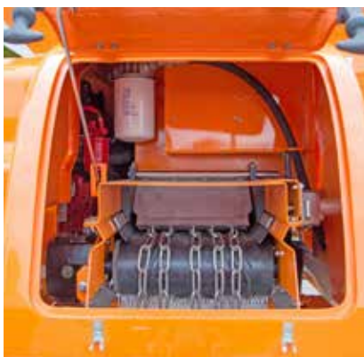
The material is transported by a belt conveyor to the charging system
