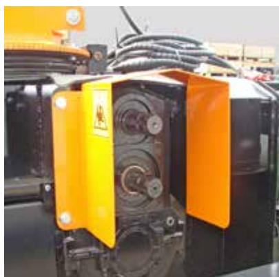
Transmission with two PTO outputs (rear-540 / front-1000 rpm)
