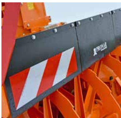
Rubber covers protect against dusting
