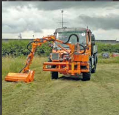
MULTIFUNCTION ARM WWP500U MOWING HEAD GK 110
