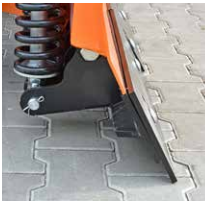
Blades with 30 degrees (perpendicular available)
