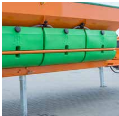
RORO (Roll-on / Roll-off) system for easier loading of PT70 spreader on the carrier platform
