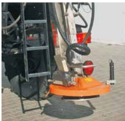
Adjustable spreader unit height
