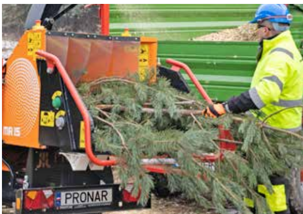
Loading ramp and safety bar
