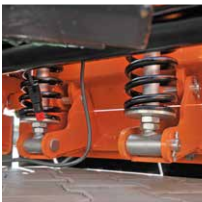
Spring shock absorption of the blade
