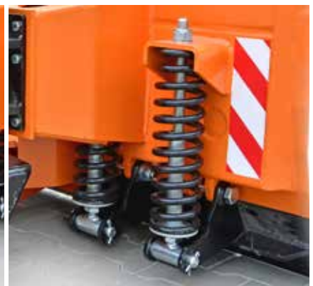
Blade spring protection
