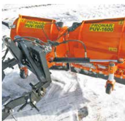
Electrohydraulic adjustment of the working angle
