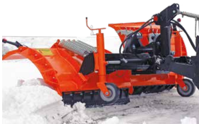
Segmented mouldboard with spring safeguard
