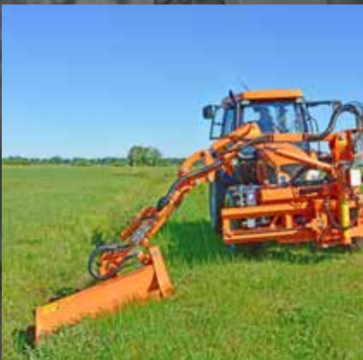
MULTIFUNCTION ARM WWP500 MOWING HEAD GK 140
