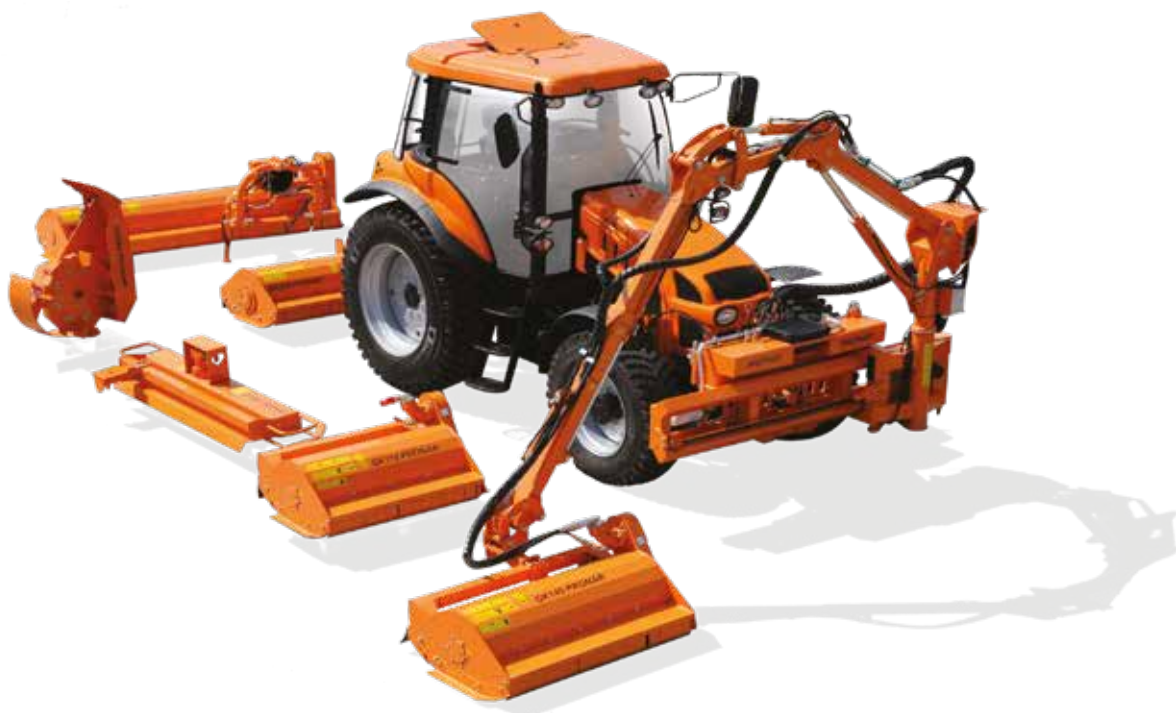
Hydraulic boom travel along the guide rail for selecting the appropriate working position
