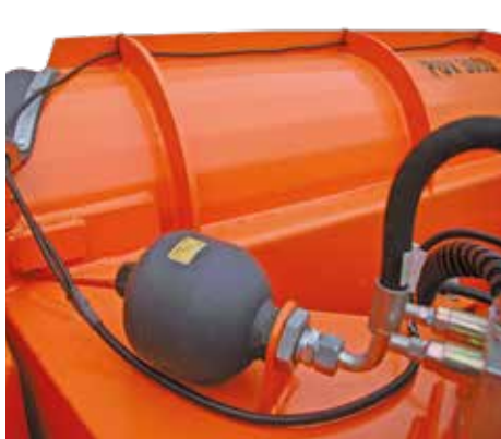
Hydraulic shock absorption
