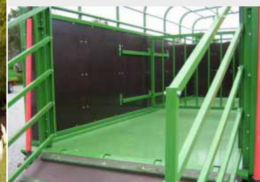
Platform with cattle separating inner barrier
