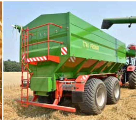
Operator's platform on rear side with foldable ladder
