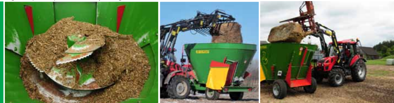
Auger with optimal shape increases efficiency of mixing
