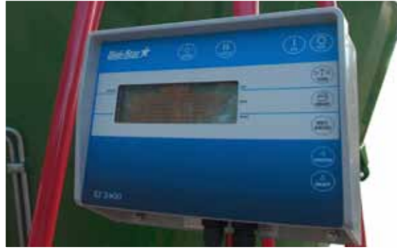
LCD display follows the weight of fodder and time of work
