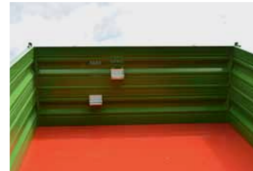
Loading box with reinforced floor suitable for euro pallet transport
