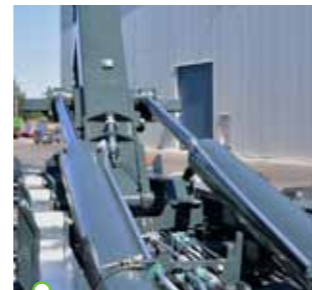
Two main cylinders increase strength and stability of the framework
