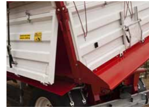
Chute over the entire width of the trailer
