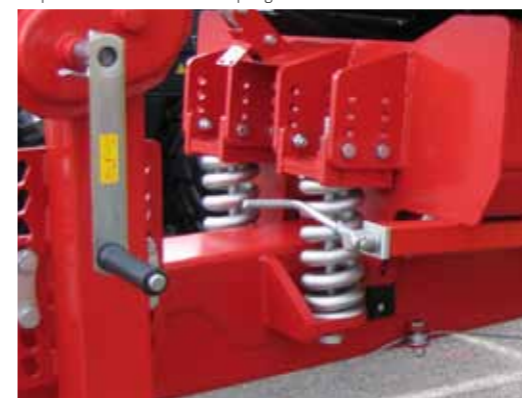
Suspended drawbar with steel springs
