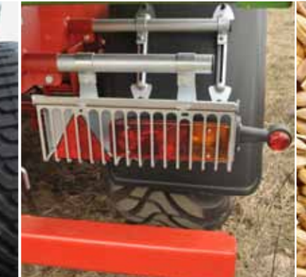
Rear lamps with protective grating
