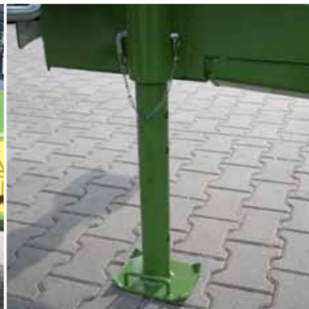
Drawbar support: straight, mechanic
