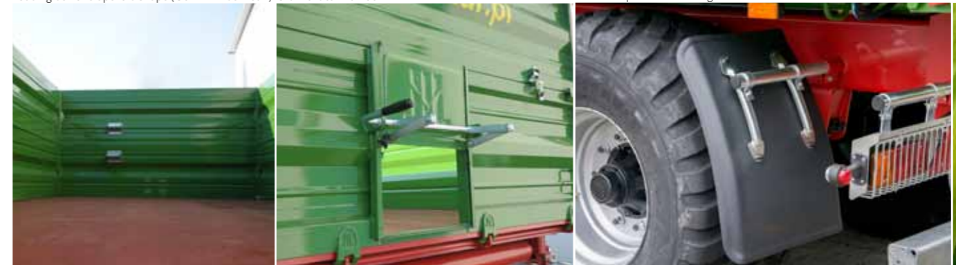
Loading box of trapezoid shape ( 50 mm wider rear ) Grain chute with lock
