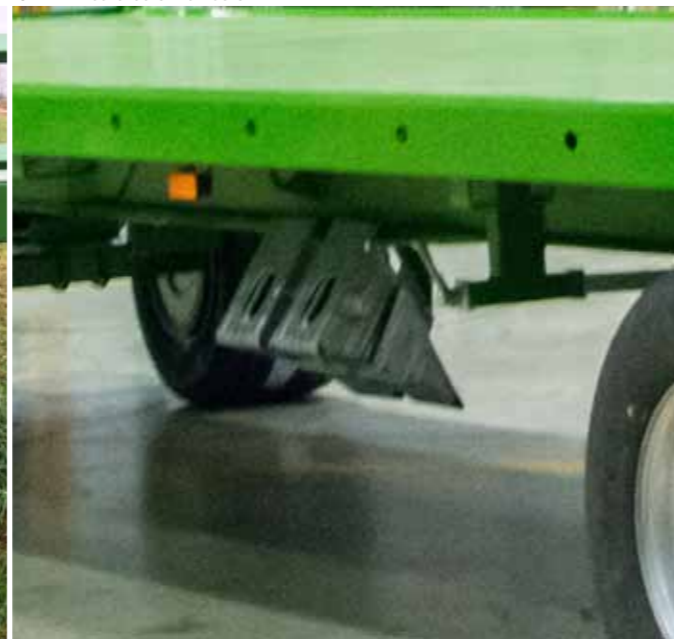
T027M - Wheel chocks with racks
