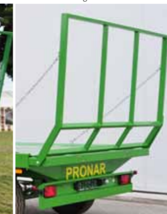
T022M rounded edges of side ladders
