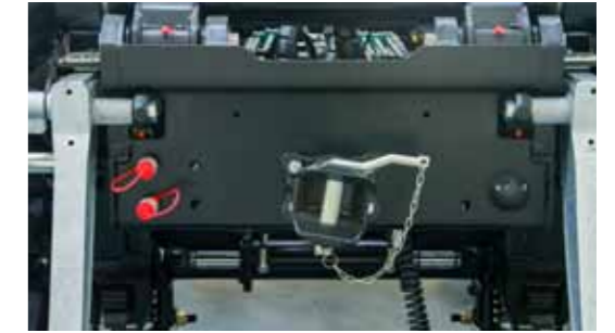
Pair of hydraulic sockets, electric socket and rear hitch at the back
