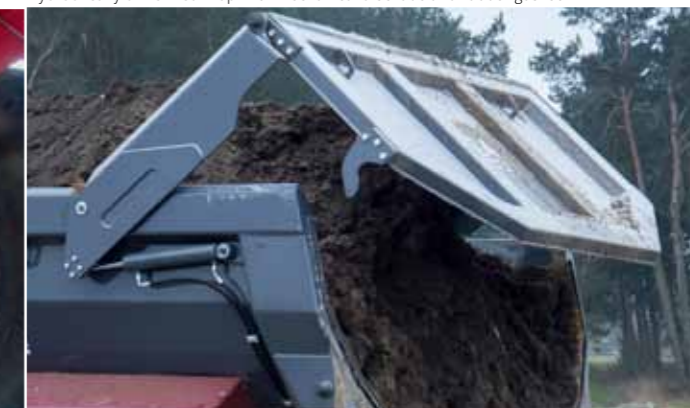
Hydraulically driven rear flap with mechanical blockade and rubber gasket
