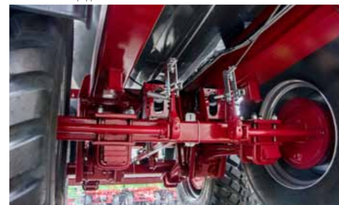
Bogie suspension on parabolic springs with 1600mm wheelbase with fixed axles with cross section 150x150 equipped in drum brakes 406x140
