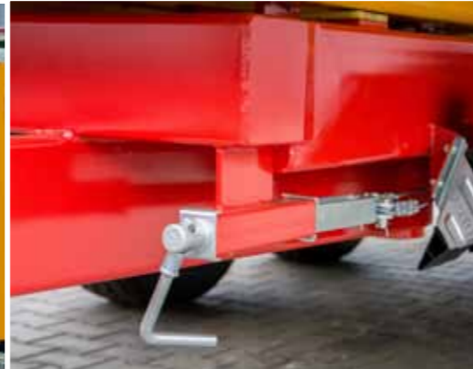
Crank hand brake
