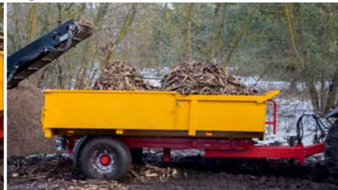
Universal and rigid drawbar to couple with lower or upper hitch of the tractor
