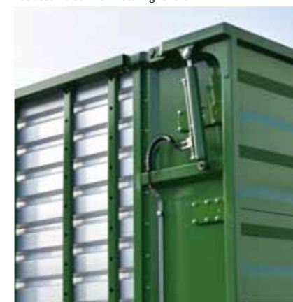
The rear wall lifted hydraulically, loading case adapted to be assembled with metering rollers.
