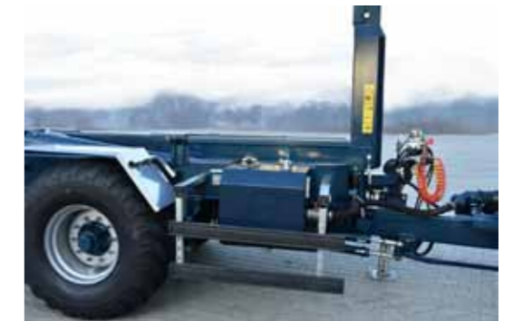
Central hydraulic system with own oil tank
