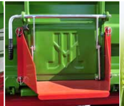
Rear grain hatch with a lever in a rear wall
