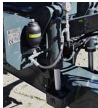
Hydraulic drawbar suspension with height adjustment
