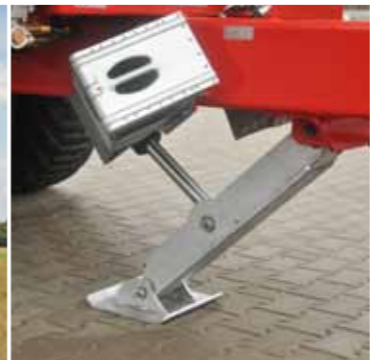
Hydraulic drawbar support
