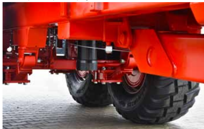
T669XL - Universal drawbar with steel springs and height adjustment. Possibility to connect with the tractor's lower or upper hitch (without approval)
