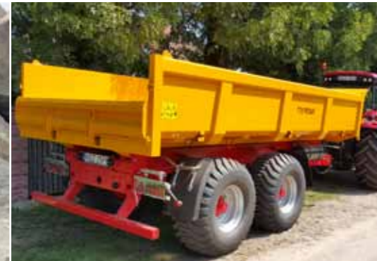
Hydraulically driven rear flap with height 370 mm, opened downwards (T701)
