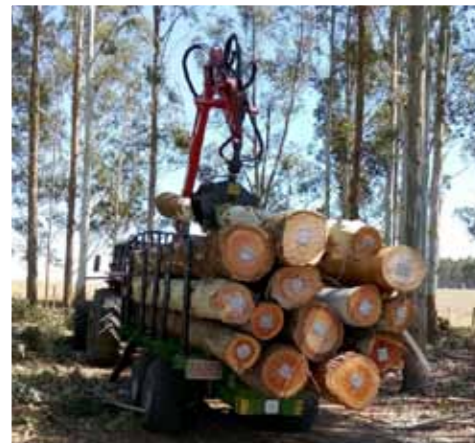
Crane with telescopic support legs and rotary grapple
