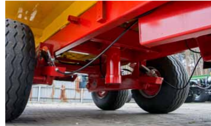
Tandem suspension with 2 trailing arms with fixed axle shafts equipped in drum brakes
