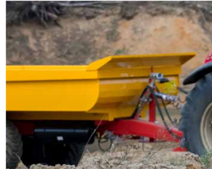
T679/4M - front wall curved facilitating unloading with the use of excavator bucket
