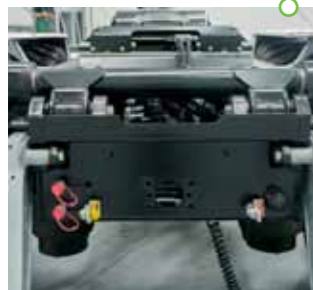
Pairs of hydraulic and pneumatic outlets at the back
