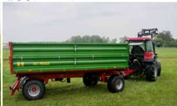
Tipping angle (backwards/sides) - 42/46°
