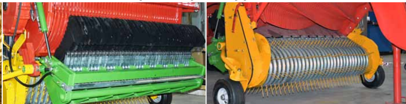
Pick-cam with eight rows of tines receiving roller and torsion aligning wheels
