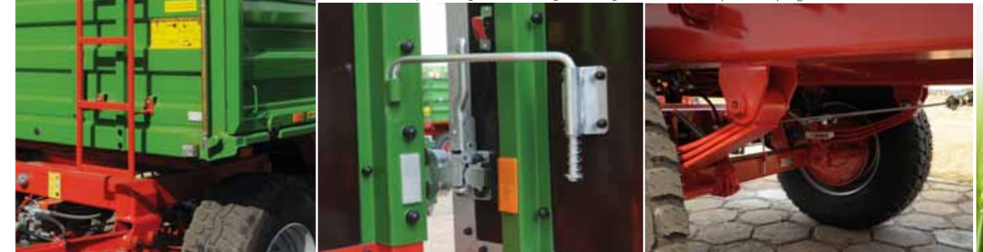
Sidewall blockade protects against self-closing and damage
