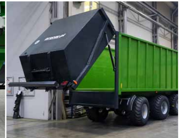
Hydraulically driven tailgate with automatic blocking system
