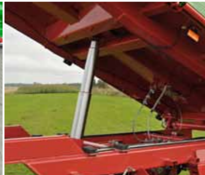
Chassis frame made of rectangular closed profiles of high strength steel
