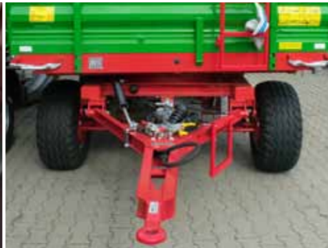
V or Y type drawbar with 40 towing eye
