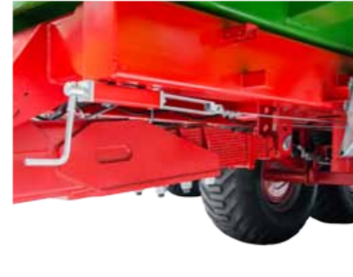
Sprung drawbar with steel spring
