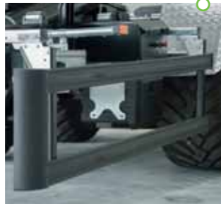
Side underrun protection
