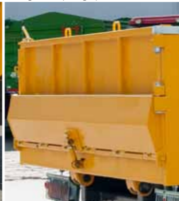
Hydraulically driven rear flap with height 325 mm, opened downwards and swinging tailgate with right side opening (optional)
