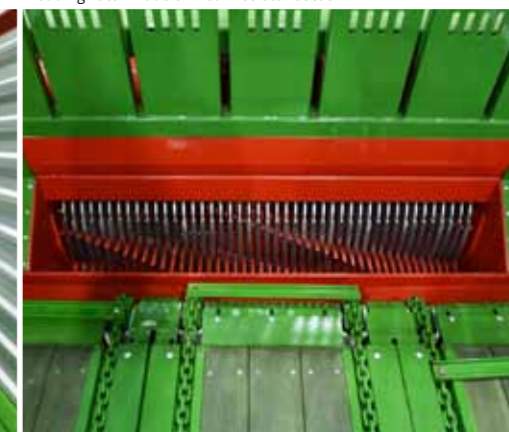
Loading rotor made of wear-resistant steel
