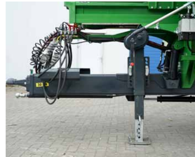
Fixed universal hitch hydraulically amortised
