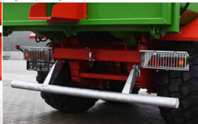
Rear lights with protective grille
