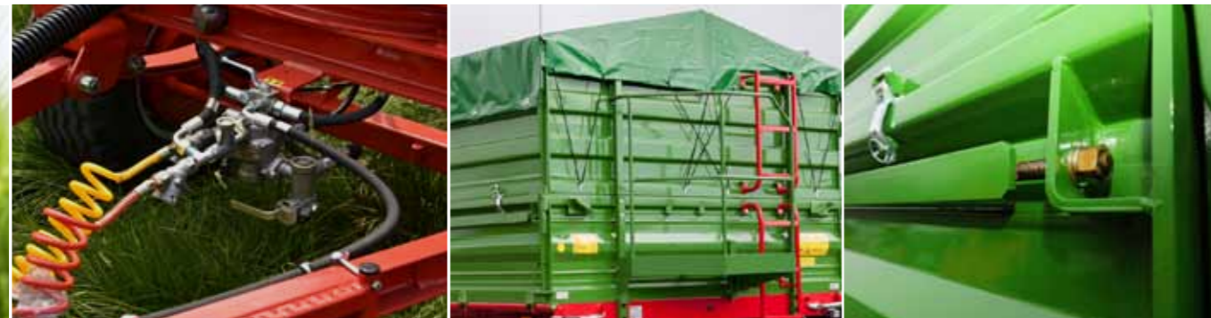
Braking system double line pneumatic with manual braking force controller
