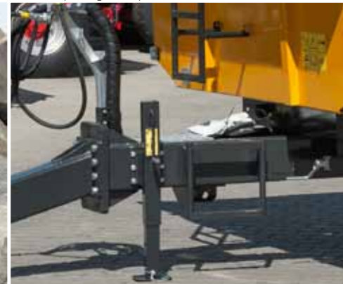
Drawbar support: telescopic supporting leg with fixed parking foot (optional)
