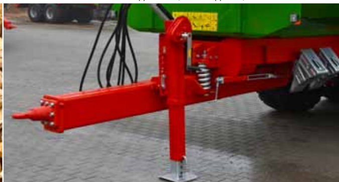
T669XL - Universal drawbar with steel springs and height adjustment. Possibility to connect with the tractor's lower or upper hitch (without approval)
