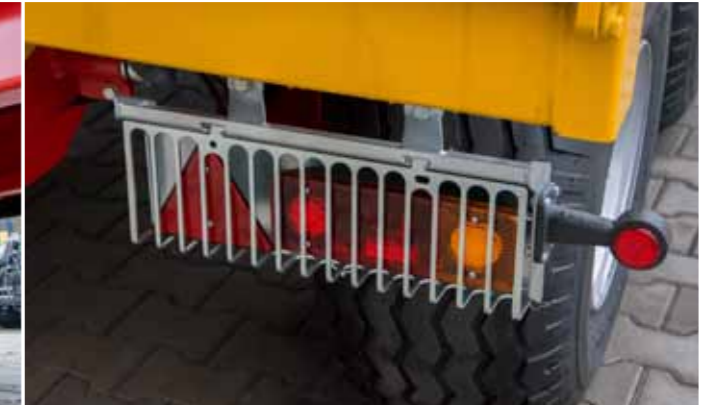
Rear lamps with protective grating
