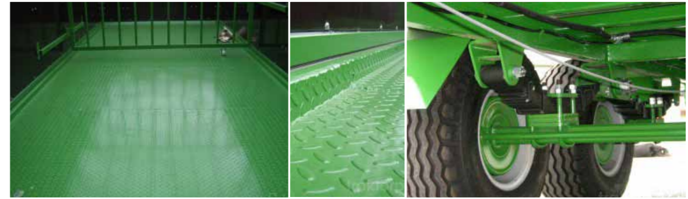
T046/1 checkered steel floor protect against slipping
