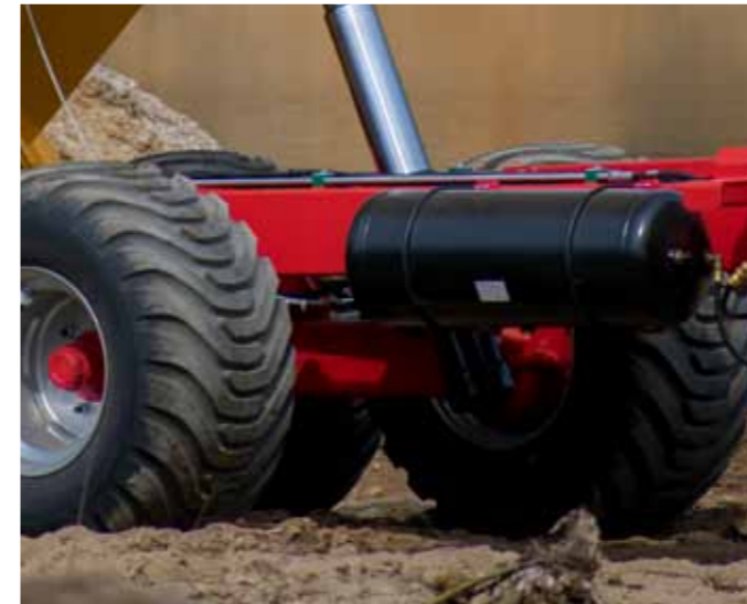
Tandem suspension with 2 trailing arms giving wide range of movement
