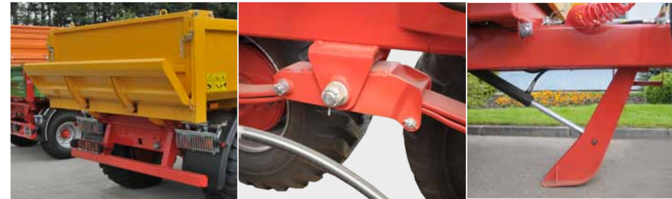
Hydraulically driven rear flap with height 450 mm (T679/2), opened downwards and swinging tailgate with right side opening (optional)
