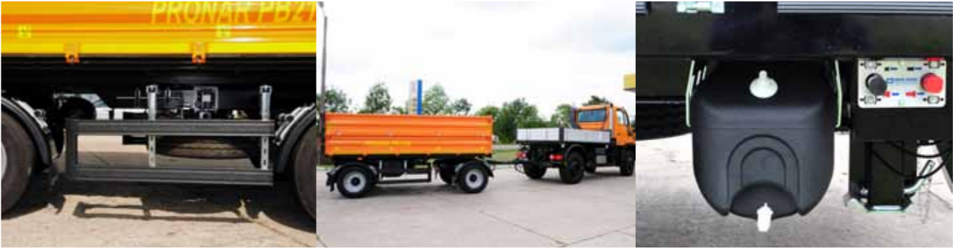
PB2100 – spare wheel, optionally equipped under chassis of the trailer PC2200 – pneumatic braking system with EBS Knorr-Bremse and water container PB2100 – an example of aggregation with two axles truck
