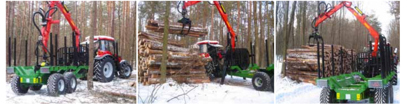
Strong stanchions and front protective barrier
