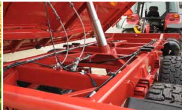
Chassis made of closed profiles
