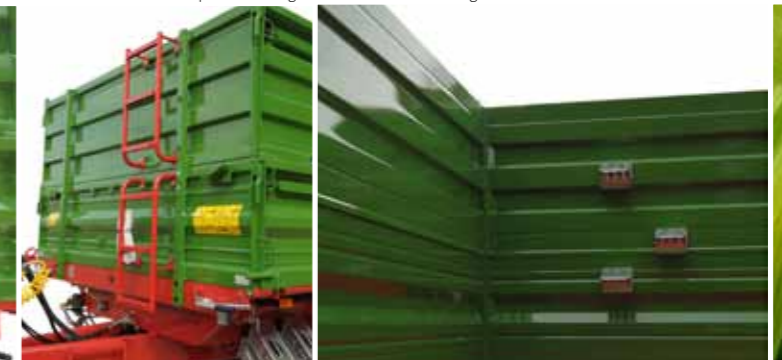
Ladder and steps facilitating the access to the loading case
