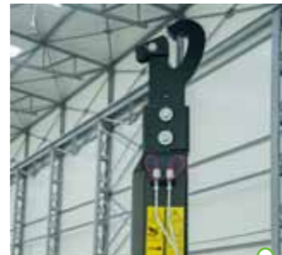
Pair of hydraulic sockets on the hook
