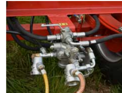
Braking system double line pneumatic with manual speed force controller
