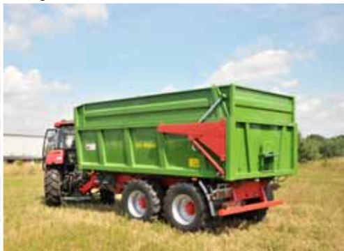
Loading box with vertical reinforced ribs (T679)
