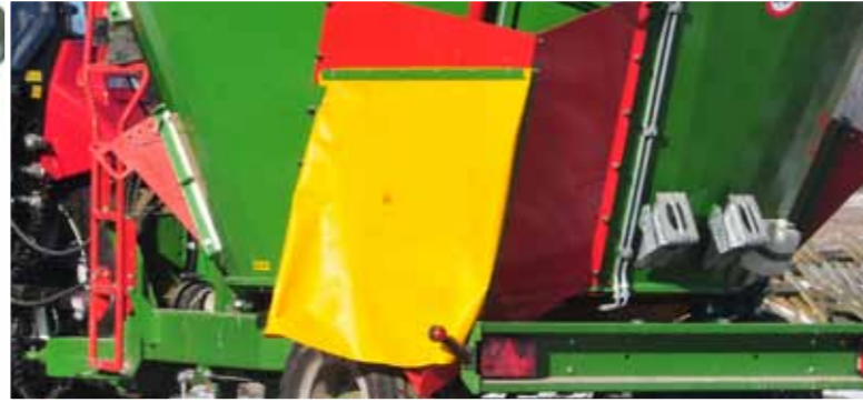
VMP-10S - discharge windows with gutters and covers
