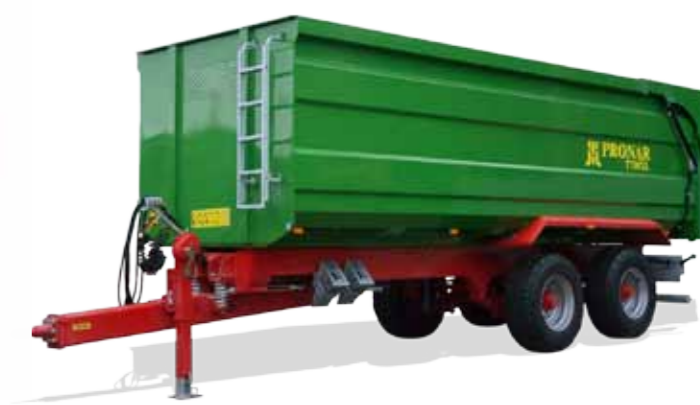
T700 - Universal rigid drawbar suspended with springsteel feather and height adjustment. Possibility to connect with the lower or upper hitch of the tractor
