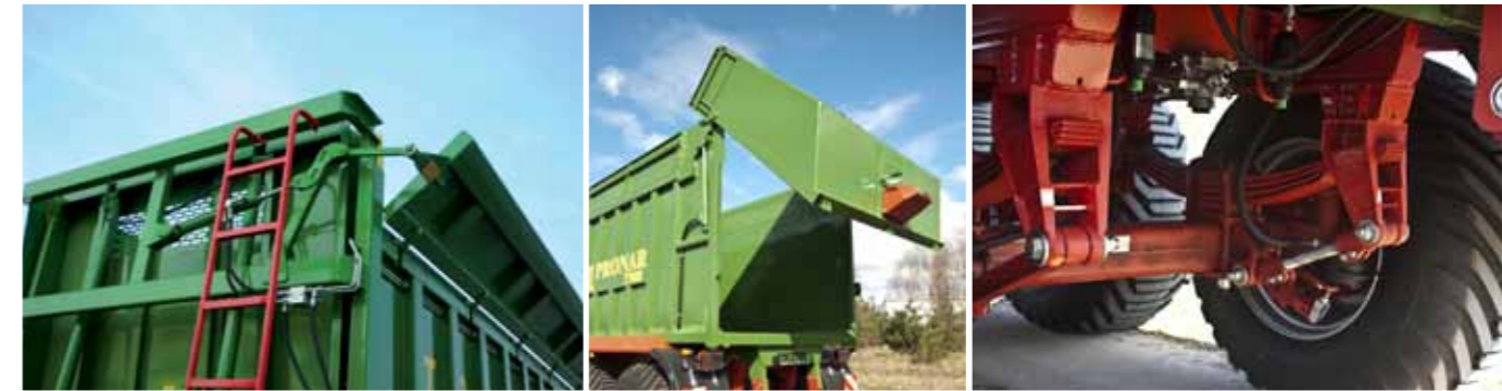
Hydraulically driven side flap with automatic locking system
