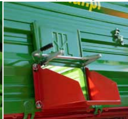
Grain chute with lock for precise unloading
