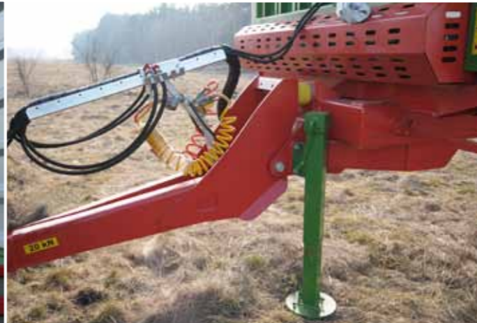
Drawbar support telescopic mechanical straight leg
