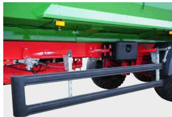
T700M - Side underrun protection
