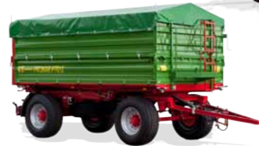
Loading box with reinforced floor suitable for euro pallet transport
