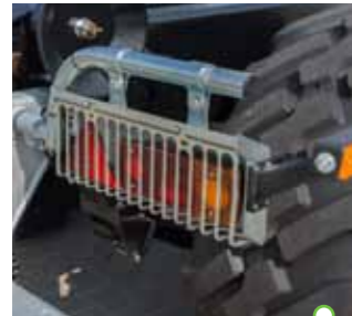
Rear lamps with protective grating
