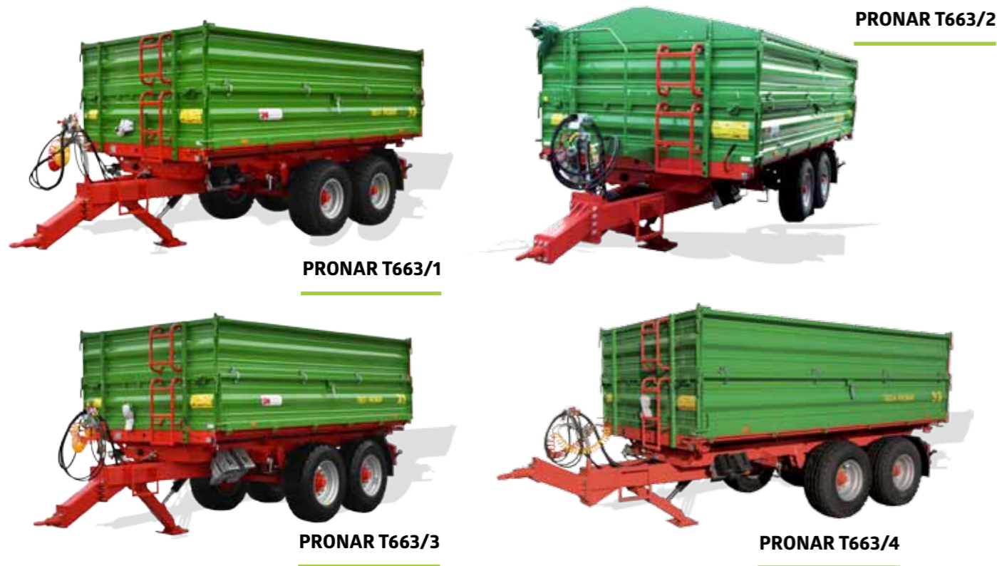
Universal rigid drawbar to connect with the lower or the upper hitch of the tractor
