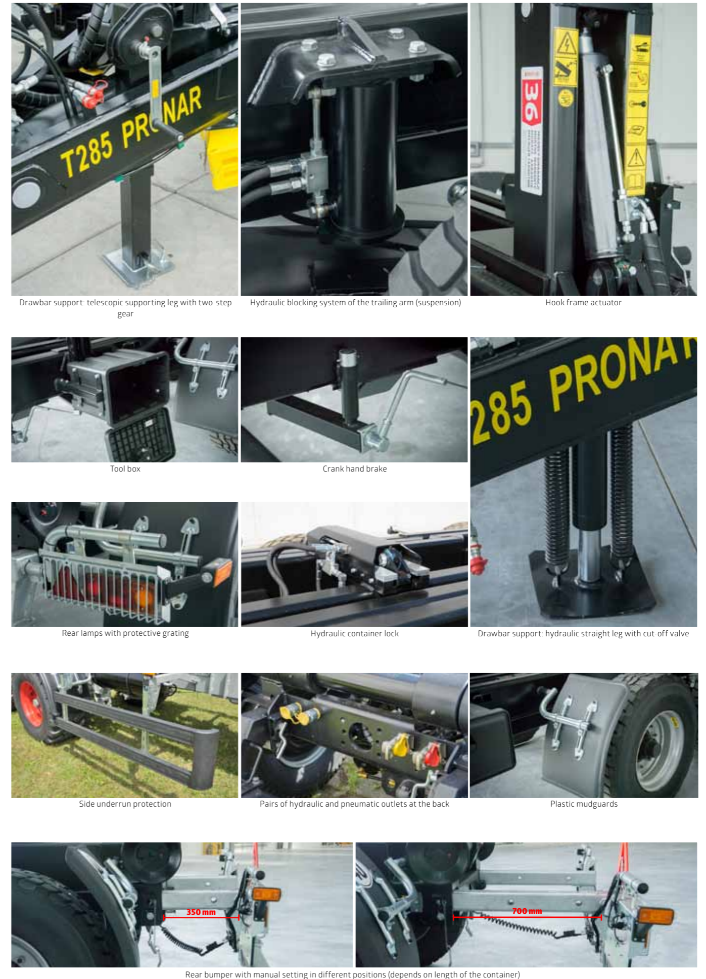
Rear bumper with manual setting in different positions (depends on length of the container)
