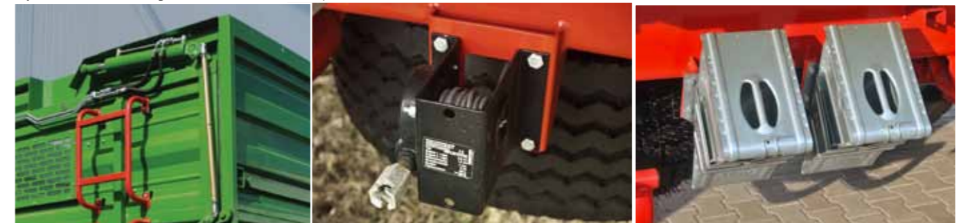
Hydraulic control and locking of the sidewall lift (T680H)
