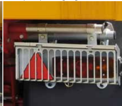
Rear lamps with protective grating
