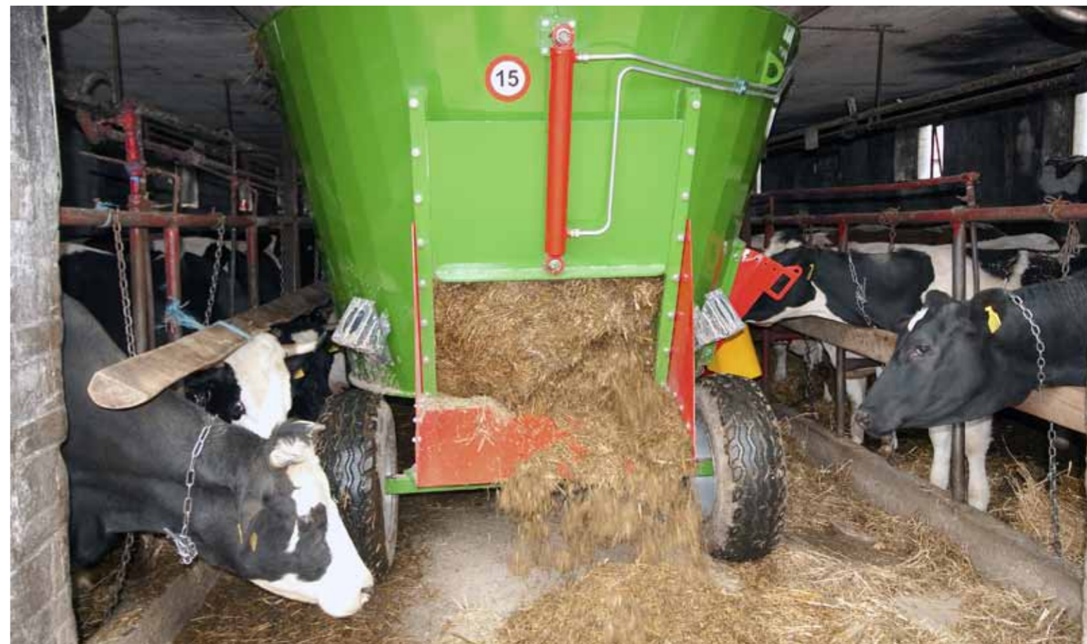
PRONAR VMP-5ST – Two discharge windows: rear side and right side at the front.
