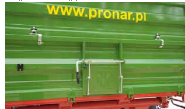
Rear grain chute with locking system
