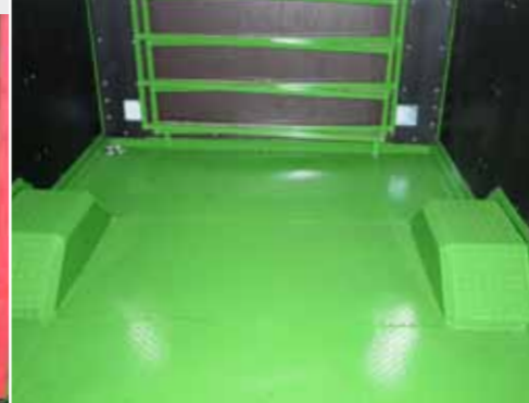
T046 - Floor made of checkered steel
