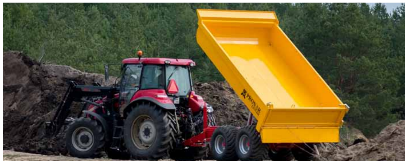
T679/4M - monocoque type of loading case, side wall and half floor made of one piece of steel, 90° angle between floor and wall
