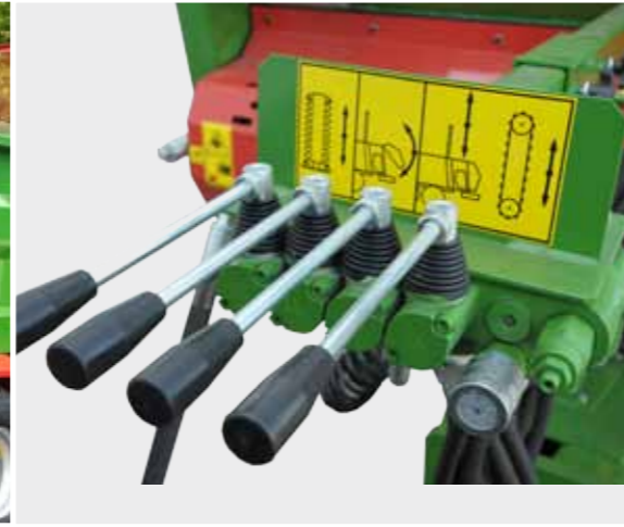
Spreader N262/1- hydraulic conveyor drive
