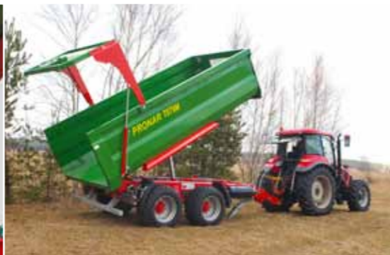
Loading box with profiled walls and reinforced upper rim (T679M)
