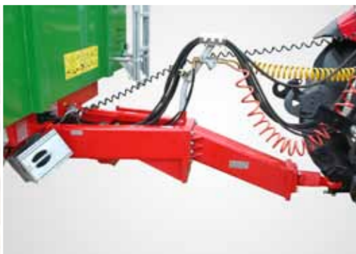
Universal drawbar to connect with upper and lower hitch of the tractor
