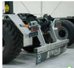
Hydraulically extendable, galvanized under-run protections. Cylinder skip - 70 cm.
