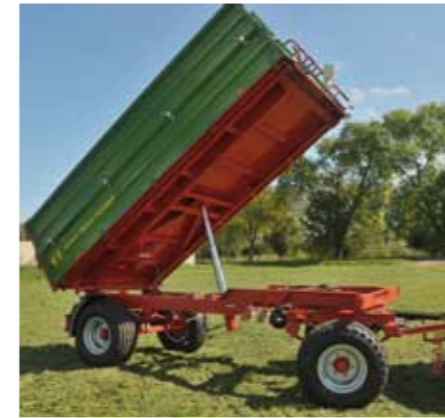
Loading case with universal system of sidewall opening and trapezoid shape of the loading box ( rear 50 mm wider than front)
