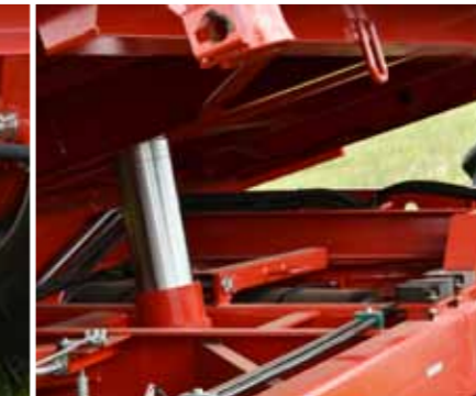
Three side tipping system with cradle
