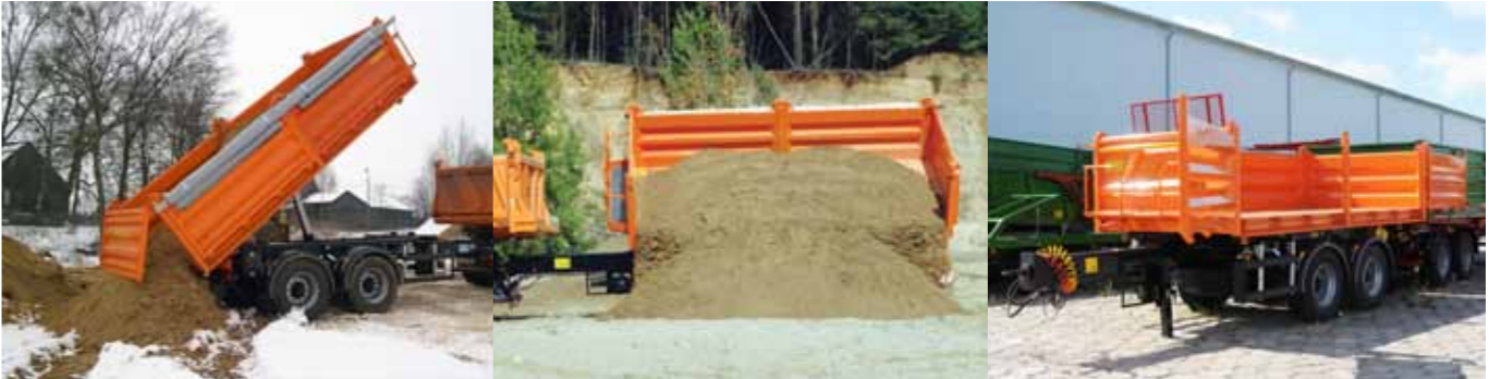
PC2100 – unloading of the trailer. Rear raised wall opened automatically when tipping PC2100/1 - unloading of the trailer. Left side Wall opened and closed with hydraulic cylinders PC2100 – left sidewall raised and side-opened
