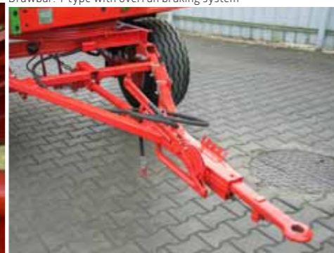
Drawbar: Y type with overrun braking system
