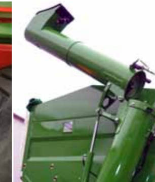
Two-segment front conveyer hydraulically folded with hydraulic safety lock
