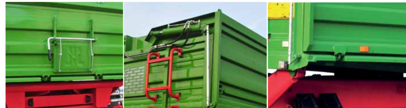
Rear grain chute with locking system
