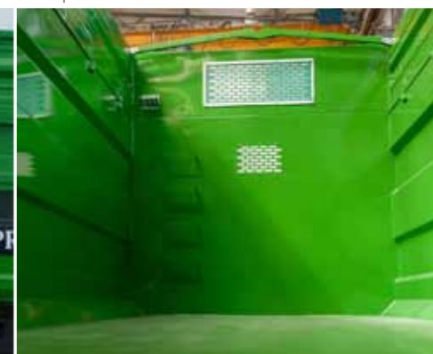
Window with PLEXI on the front wall of the load case and side steps to facilitate access to the load case
