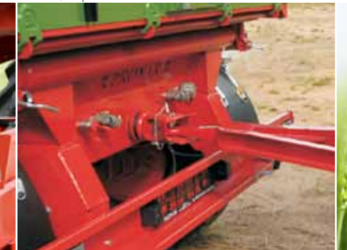
Manual, suspended rear hitch
