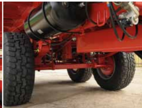
Tandem suspension on parabolic springs
