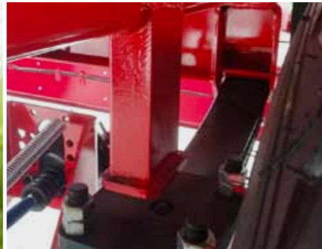
Parabolic spring suspension with steel buffer
