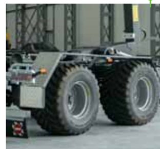
Rigid front axle and passively steered rear axle with hydraulic turning blockade
