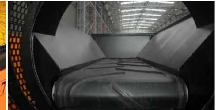
Reinforced belt on in-feed hopper conveyor
