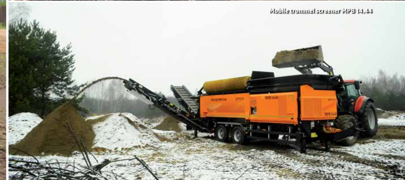
The PRONAR MPB 18.47 TROMMEL SCREEN sieving waste after biological stabilisation.
