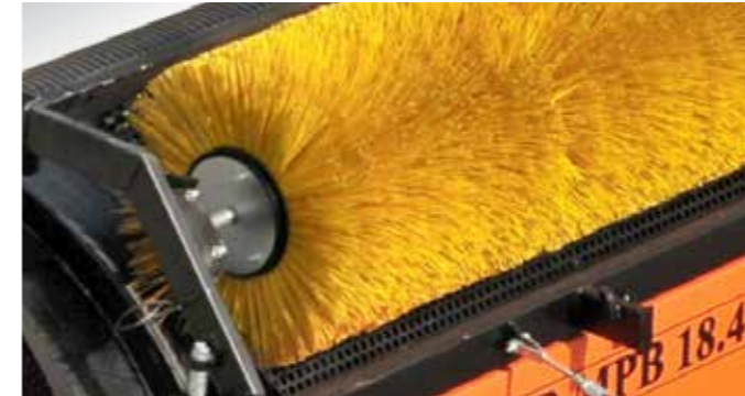
Hydraulically raised and lowered trommel cleaning brush.
