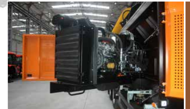
The engine and hydraulic system are mounted on a pull-out frame which provides easy access for maintenance requirements.
