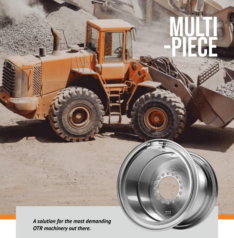
The biggest machines used in construction and mining sectors usually use multi-piece wheels which allows the highest load capacity and durability on the market.
