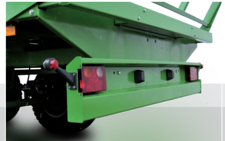
Rear under-ride guard integrated with rear lights
