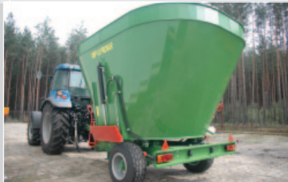
VMP-10 - two symmetrical feeding windows on both sides of the wagon.
