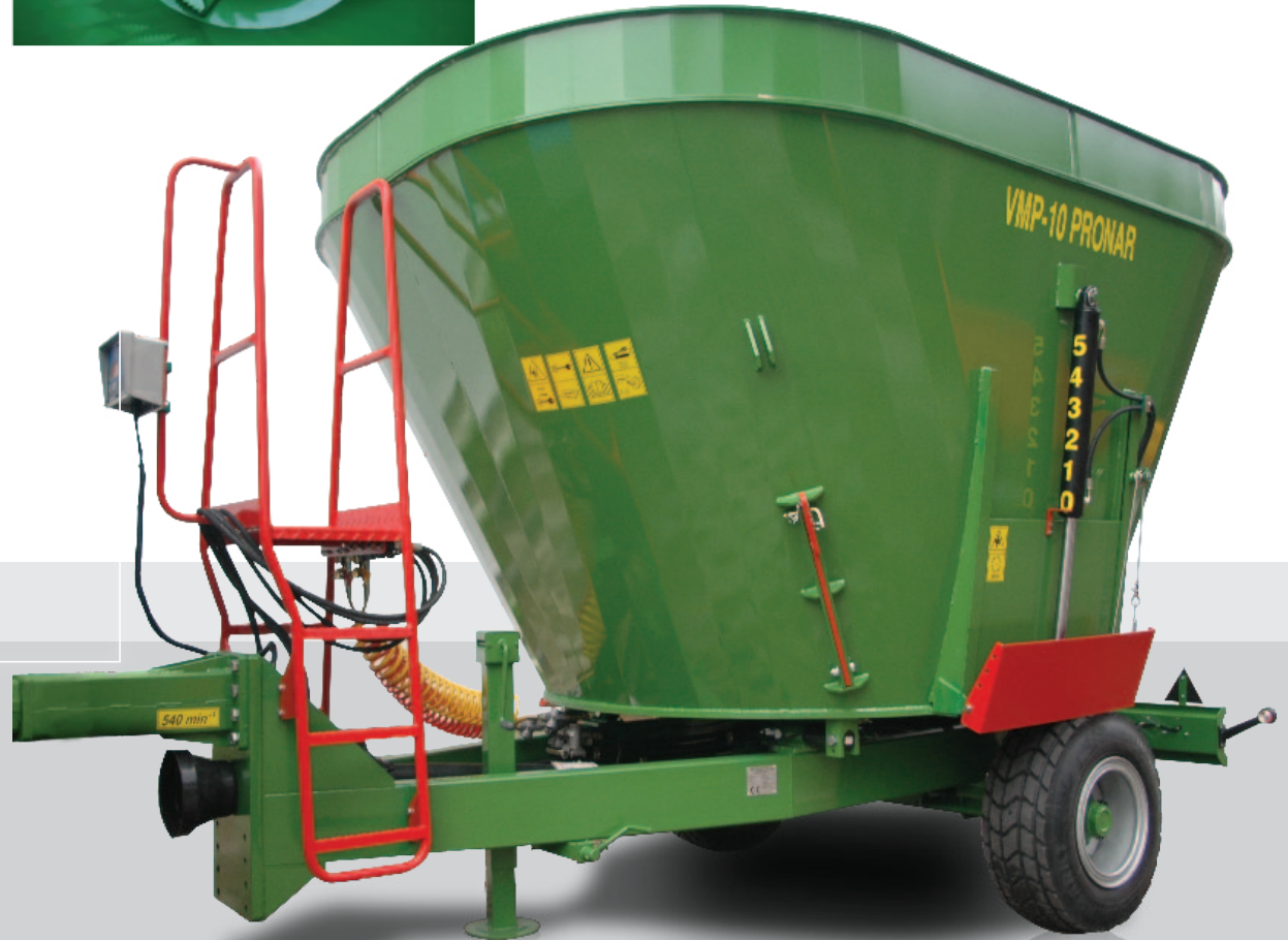
VMP-10 - two symmetrical feeding windows on both sides of the wagon.
