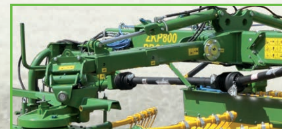
Hydraulic and synchronized raising and lowering of rotors
