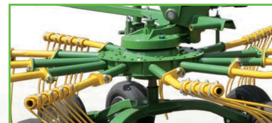
Dry rotor transmissions of our own design
