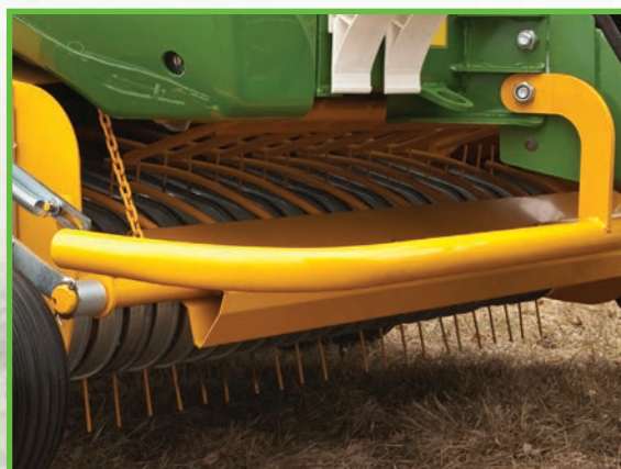
Dosing rake – adjustment of thickness of fed material layer
