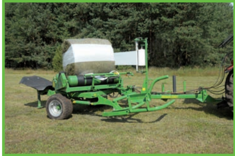
Front loading when the wrapper is positioned next to the side of the bale
