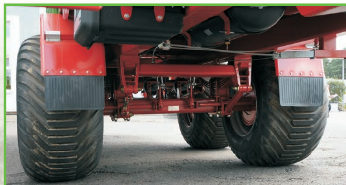
Tandem parabolic leaf spring suspension with passive turning system
