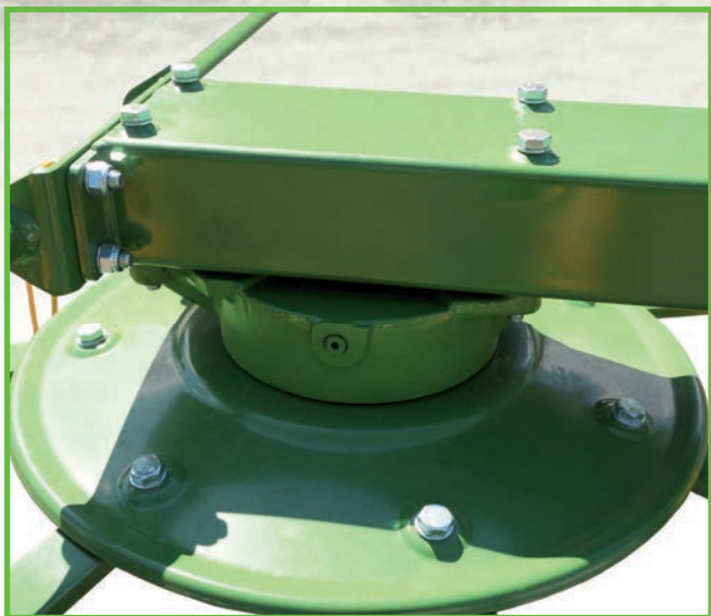
Dry lubrication and maintenance-free gear rotors
