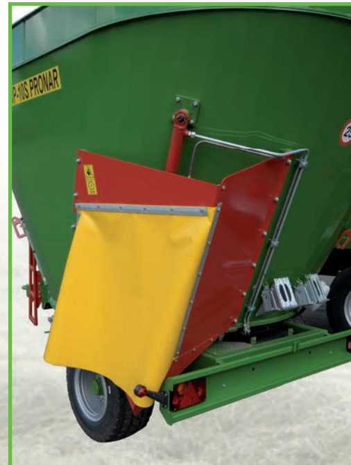
Slant arrangement of discharge openings
