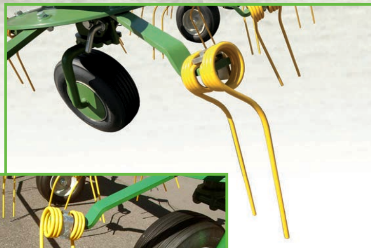
Innovative method of fixing the tedder spring tines
