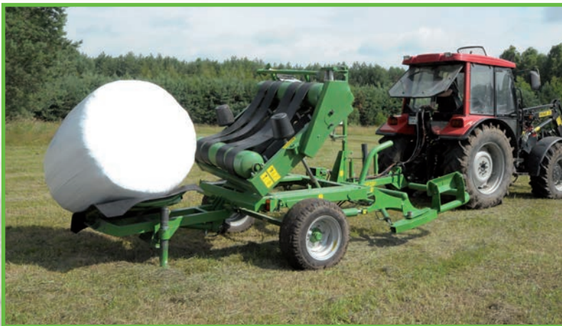
Bales can be unloaded on their side or front surface
