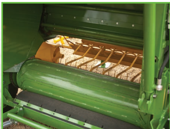
Dosing rake – adjustment of thickness of fed material layer
