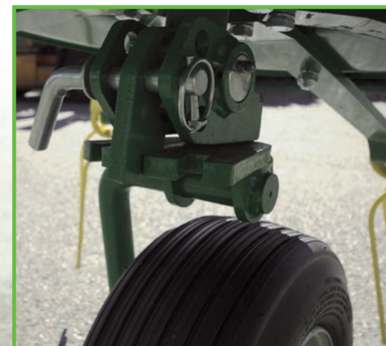
Adjusting the angle of ejection - inclination 13°, 16°, 19°
