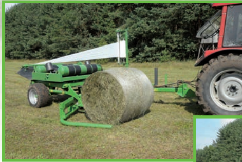
Front loading when the wrapper is positioned next to the side of the bale
