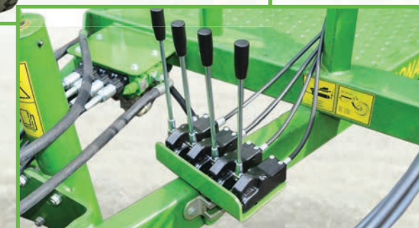
Hydraulic manifold controlled by means of strings
