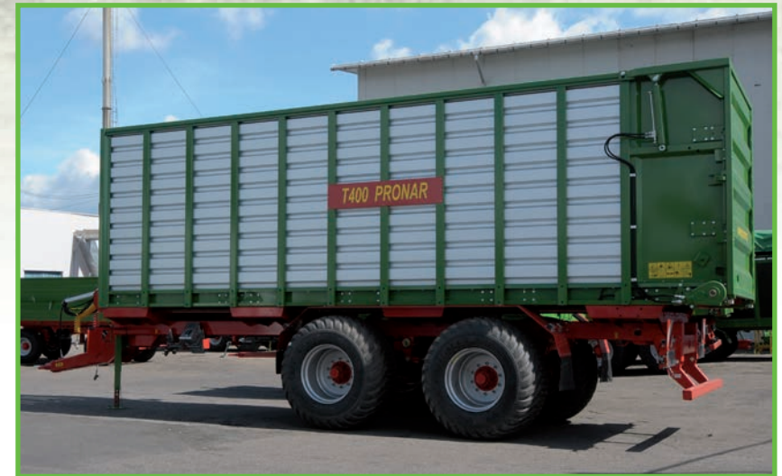
The trailer walls are made of trapezoid profiles covered with aluminium-zinc coating
