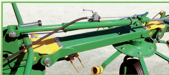
Synchronous folding and unfolding of rotors - hydraulic system
