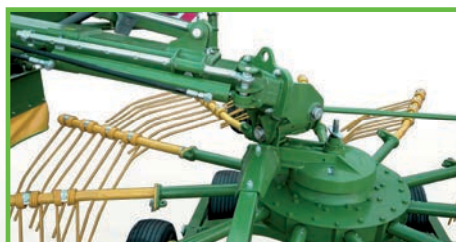
Hydraulic cylinders adjust working width of the machine – 7-8 m
