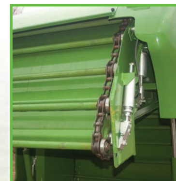
Rolling chain makes it possible to collect over-dried material as well as moist material
