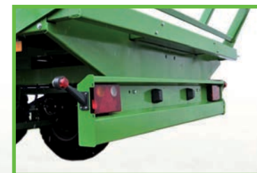
Rear under-run protection integrated with rear lights
