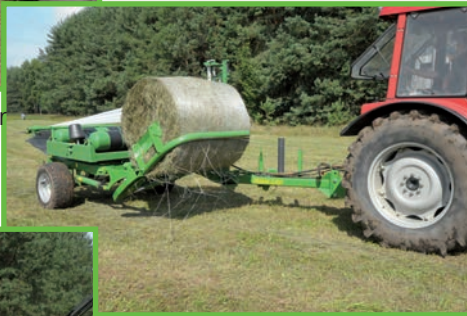
Front loading when the wrapper is positioned next to the side of the bale
