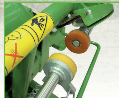
Hydraulic cutting and grabbing system cuts and holds the film in the position for wrapping the next bale,
