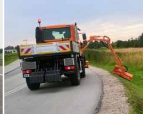
Mowing of a hard-to-reach roadside using a WWP500U multifunction arm and GK 110 head.
