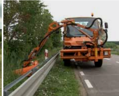
Mowing of a hard-to-reach roadside using a WWP500U multifunction arm and GK 110 head.
