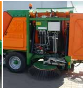
Tilting service hatch.
