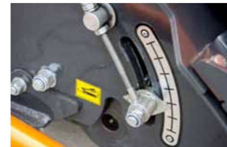
Stepless mowing height adjustment
