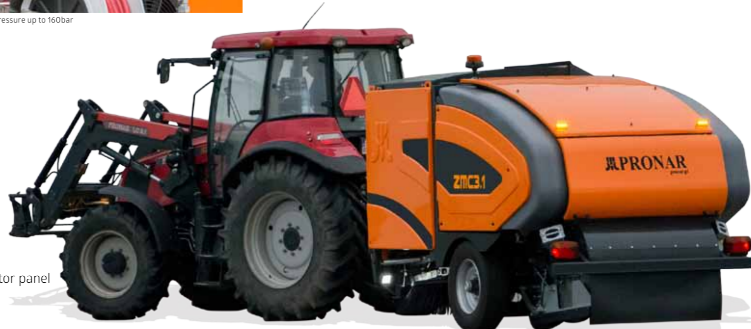
Warning lights - mounted on top cover
