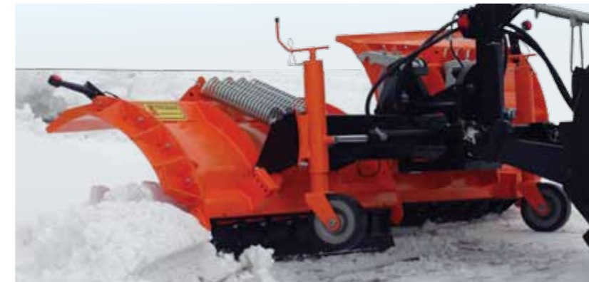
Segmented mouldboard with spring safeguard.
