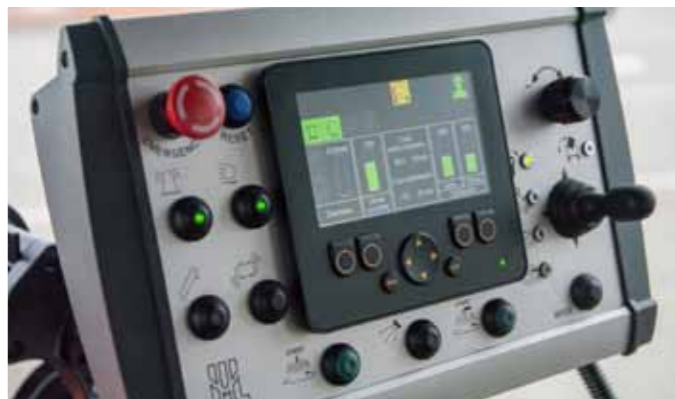
Control panel – all sweeper functions are controlled using a panel located in the tractor cab
