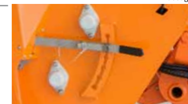
Aperture adjustment to set the spreading dosage.
