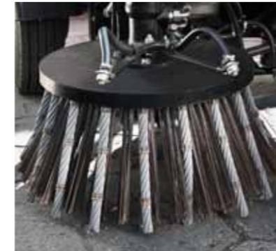
Special brush for removing plants from carriageway edges.
