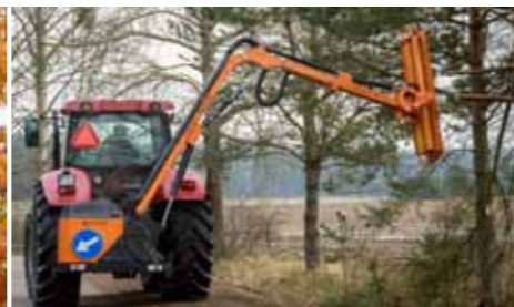
WWT700T, WWT800T – Long arm reach is provided thanks to hydraulic telescopic sliding
