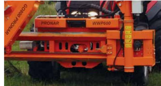
WWP600 multifunction arm — hydraulic movement of working arm over guide rail.
