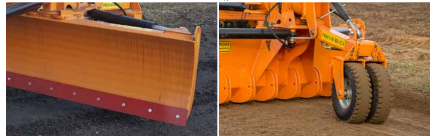
The mouldboard is equipped with a steel blade made of wear-resistant steel
