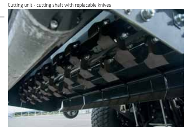
Cutting unit - cutting shaft with replaceable knives
