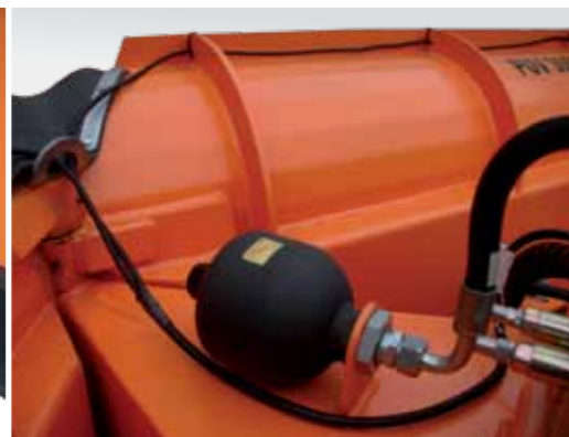
Hydraulic shock absorption
