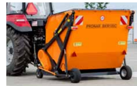
Container with 2 m³ volume for collecting shredded material
