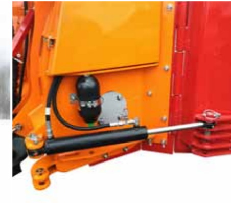
Hydraulic control of the widening
