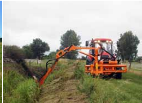
WWP600 with G0800 ditch digger. Long reach fits perfectly for desludging.
