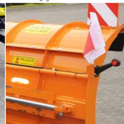
Position marking lights
