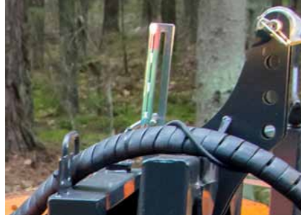
The work position indicator helps to set the optimum height of the carrier suspension
