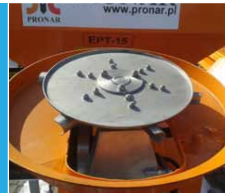
Stainless steel spreading disk.
