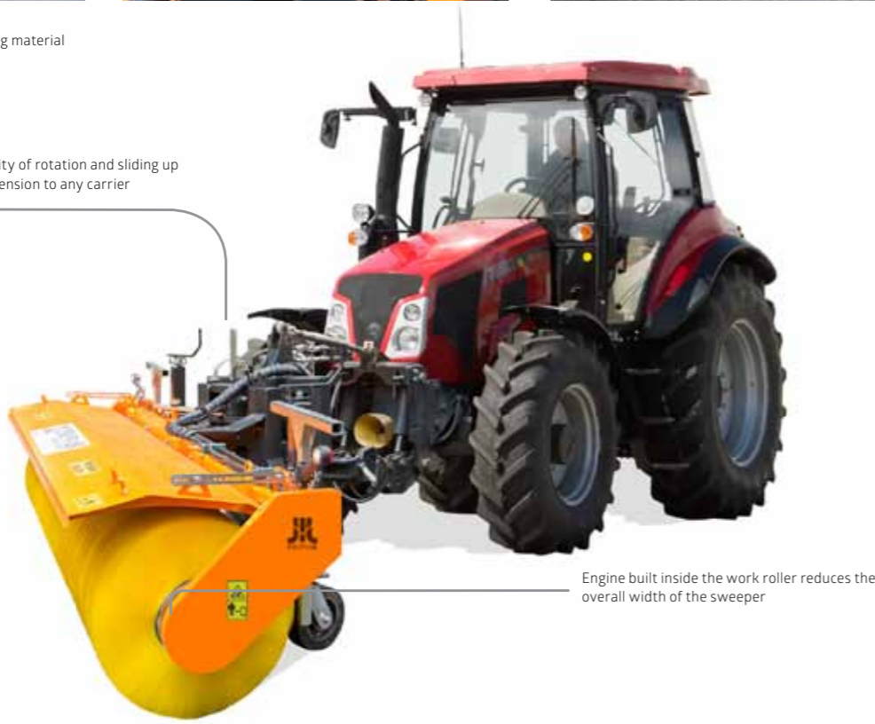
8 types of roller brush available (4 hardness levels of bristles of the brush and 2 types of rings flat or „honeycomb“)
