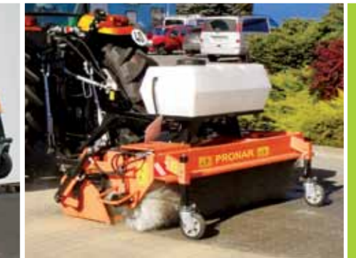
Sprinkler system reduces dust and particulate emissions.
