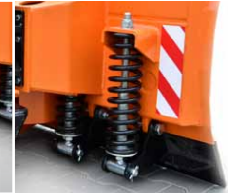
Blade spring protection
