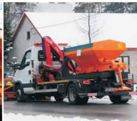
Capability of aggregation with a hook loader.
