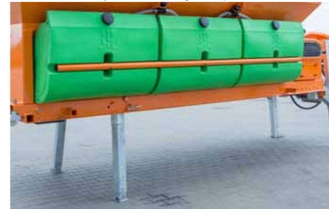
RORO (Roll-on / Roll-off) system for easier loading of PT70 spreader on the carrier bed
