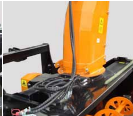
Hydraulic discharge chute rotation and adjustment of throwing distance.
