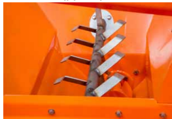
Additional mixer facilitates aggregate breaking
