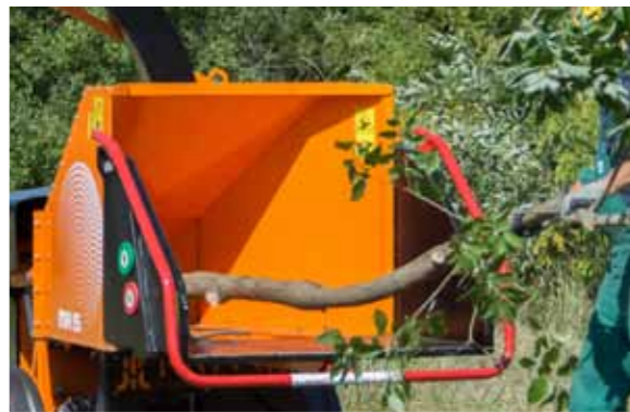
The branches are picked up automatically by means of hydraulically driven feed rollers.
