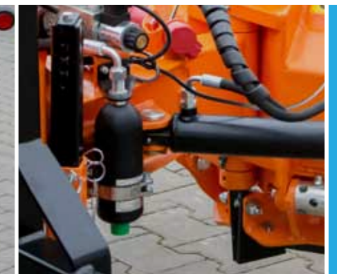
Hydraulic shock absorption
