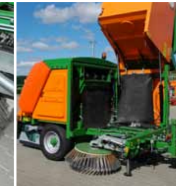
Hydraulic hopper dumping system.
