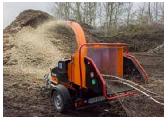
Loading ramp and safety bar.
