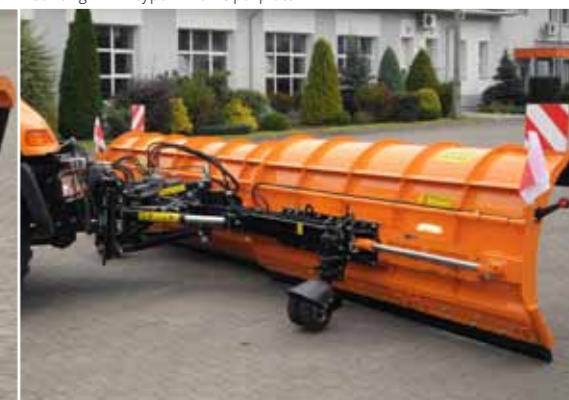
Mounting – DIN type A municipal plate
