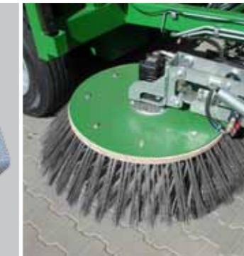
Hydraulic adjustment of rotary disc brush position.
