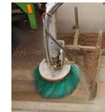
Hydraulic brush for gutter cleaning
