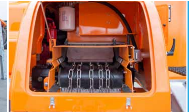
The material is transported by a belt conveyor to the charging system
