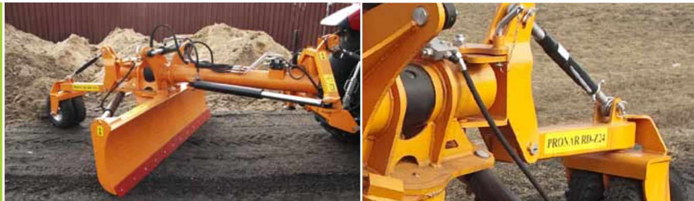
The turnbuckle is used to set the working depth
