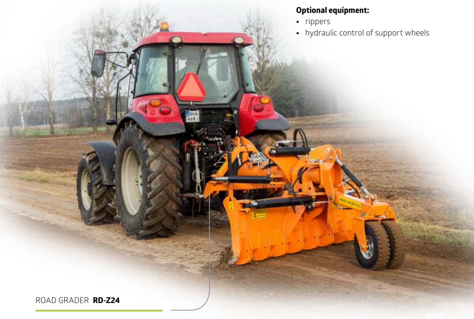
The turnbuckle is used to set the working depth
