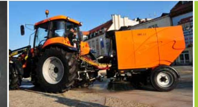
Hydraulically articulated drawbar.
