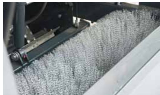
Roller brush made from segment discs
