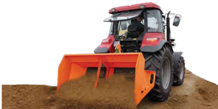
Additional mixer facilitates aggregate breaking
