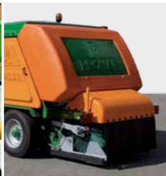
1150 litre water tank and roller brush.
