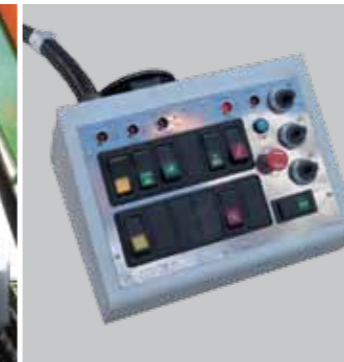
Control panel in the operator's cabin.
