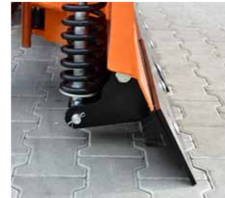
Blades with 30 degrees (perpendicular available)
