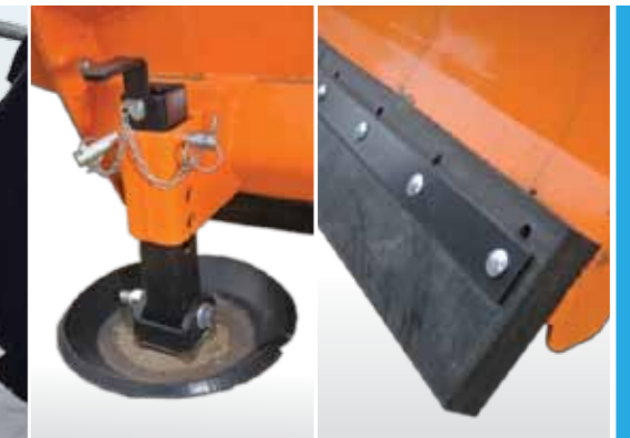
Slides made of abrasion-resistant steel. Rubber blade
