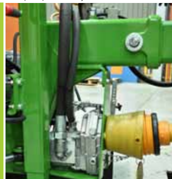
Multiplier powered by tractor PTO
