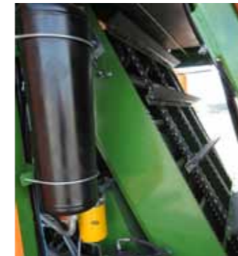
Scraper conveyor transporting waste to the hopper.
