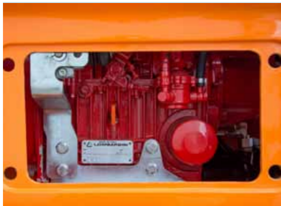
Diesel engine with power 16,2kW - SPT70)
