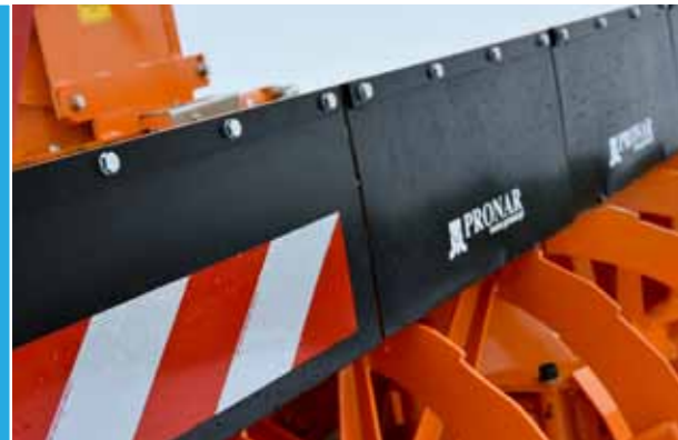
Rubber covers protect against dusting.
