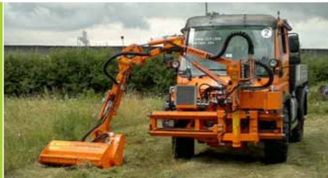
WWP500U multifunction arm with GK10 mowing head on Unimog U500
