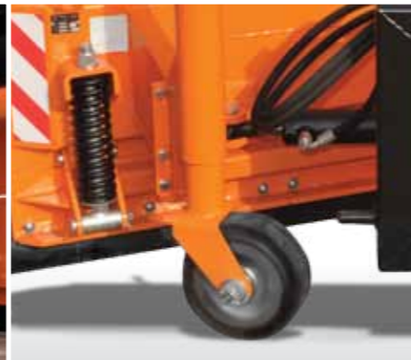
Spring safeguard (extendable blades)
