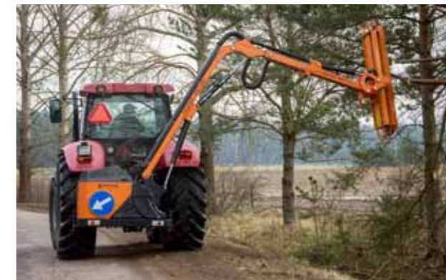
WWT700T, WWT800T- The large range is achieved due to the arm that extends by a telescopic actuator.
