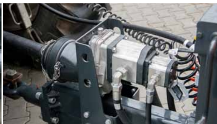
Hydraulic - Hydraulics with two hydraulic pumps and oil cooler
