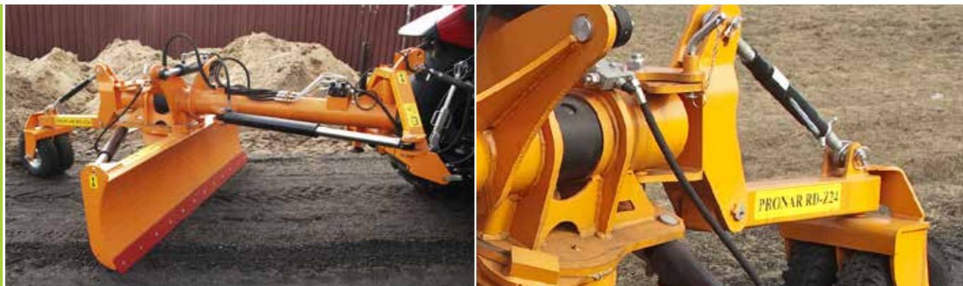
The turnbuckle is used to set the working depth
