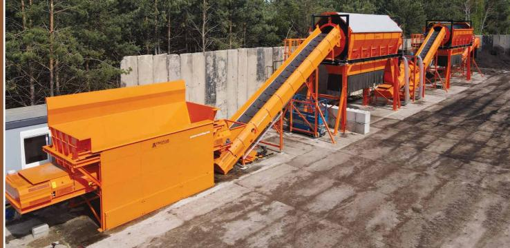
Depending on specific features, the stationary trommel screen is used for the mechanical separation of the waste into fractions of different size. The size-based separation process produces individual material streams for further processing, which improves efficiency.
