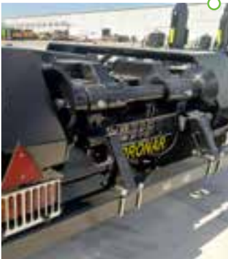
Rear bumper with setting in one position (no slid lights) 500 mm
