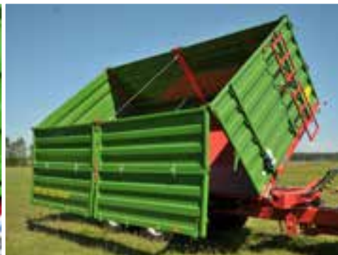
Loading case with universal system of walls opening (T683)
