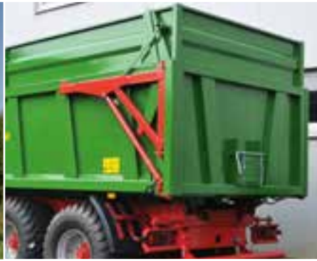
Hydraulic tailgate lifting system.
