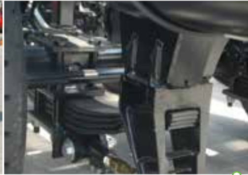
Tandem suspension with 4 parabolic Springs
