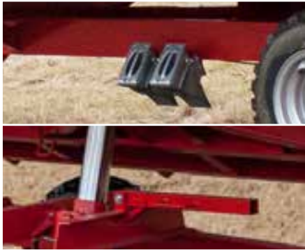
Wheel chocks with pockets as standard equipment and service support for loading case
