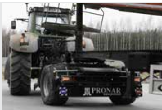
Single-axle TD111 during aggregation with a semi-trailer.
