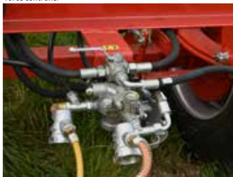
Braking system double line pneumatic with manual speed force controller
