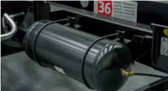
Air tank for pneumatic braking system
