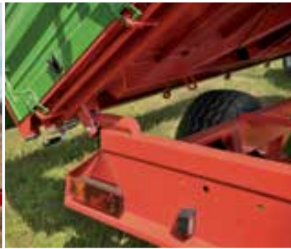
Tipping system with ball joints at the rear
