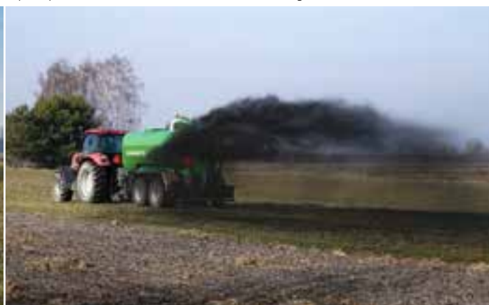
Impact spiller (stream directed downward to reduce nitrogen loss)
