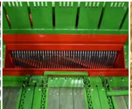
Loading rotor made of wear-resistant steel
