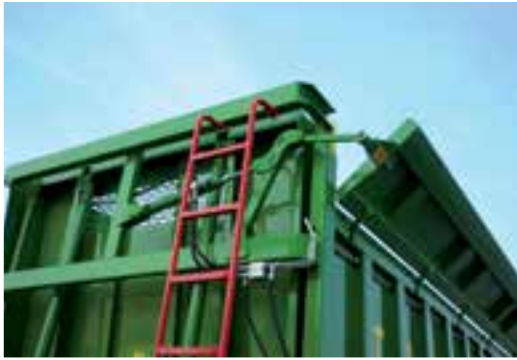
Hydraulically driven side flap with automatic locking system
