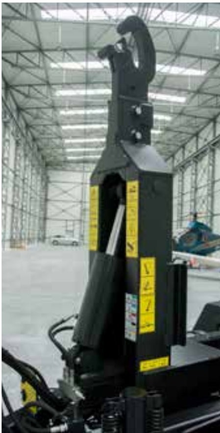
Hook frame with actuator
