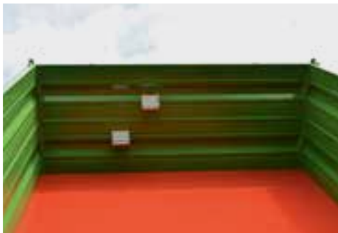
Loading box with reinforced floor suitable for euro pallet transport Parabolic springs
