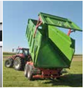
Tipping backwards at an angle of 50 degrees.
