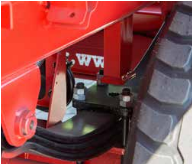
Tandem suspension with 4 parabolic springs with 1325 mm wheelbase with fixed axles equipped in drum brakes 406x120
