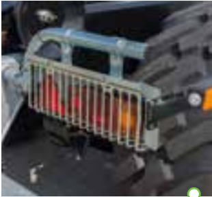
Rear lamps with protective grating
