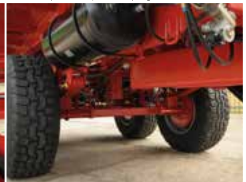
Tandem suspension on parabolic springs
