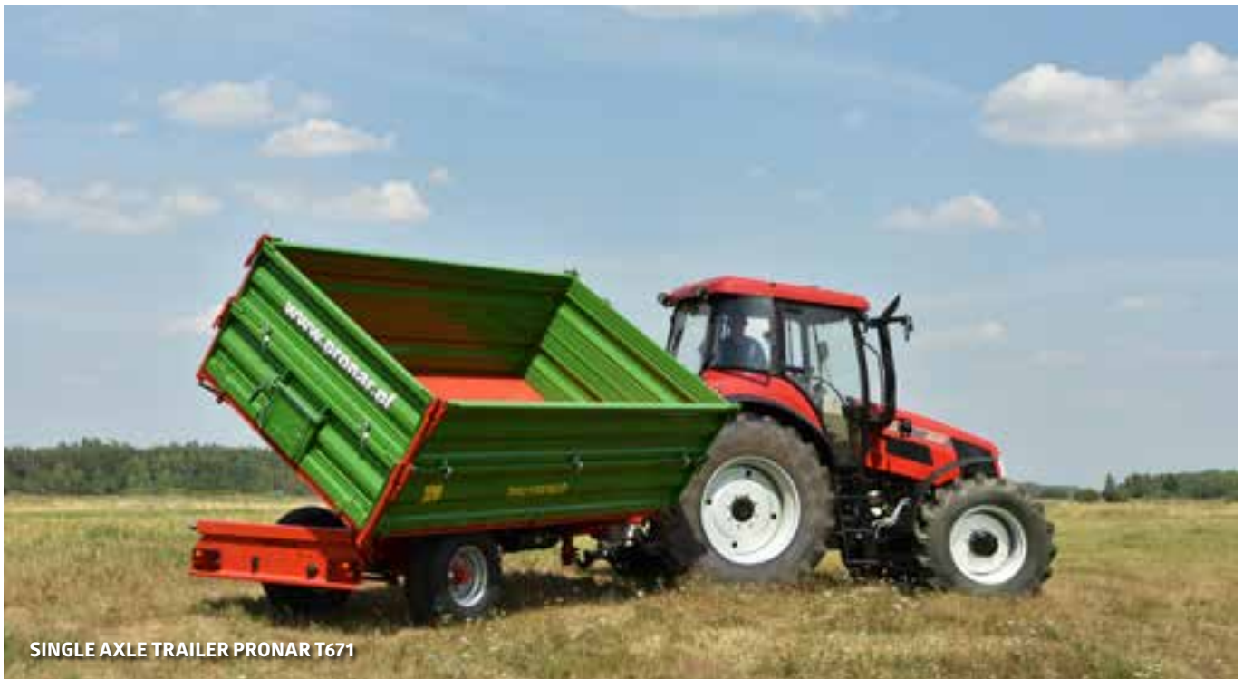
Three way tipping system with telescopic cylinder and hinged suspension
