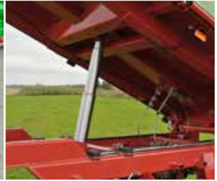
Chassis frame made of rectangular closed profiles of high strength steel
