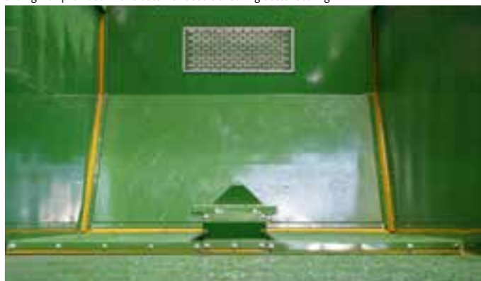
Sliding wall provided with elastomeric seals ensuring better sealing
