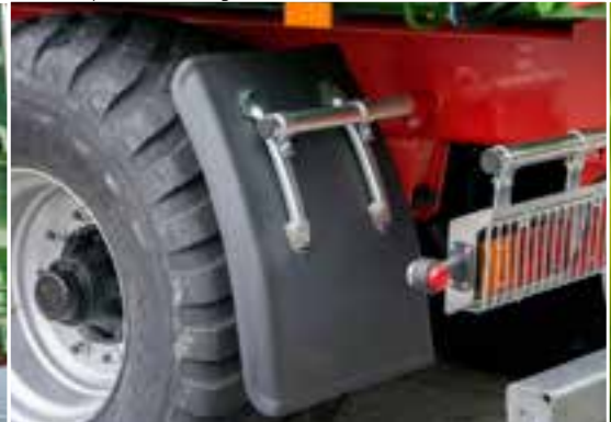
Additional plastic front mudguards - the wheels of a wheelset tandem
