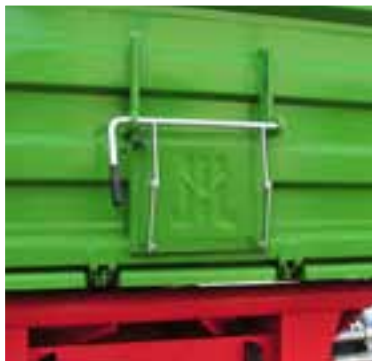
Rear grain chute with locking system
