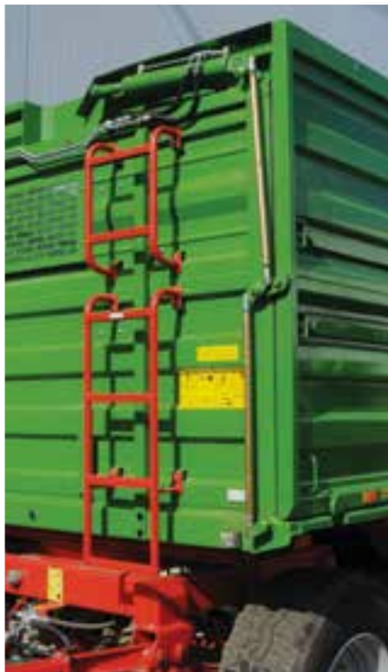
Hydraulic control and locking of the sidewall lift (T680H)
