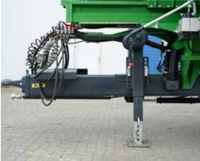
Fixed universal hitch hydraulically amortised
