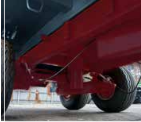
Tandem suspension with 4 parabolic springs (T679/2 and T701)
