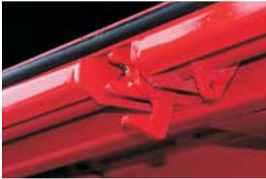
Robust wall locking near the floor
