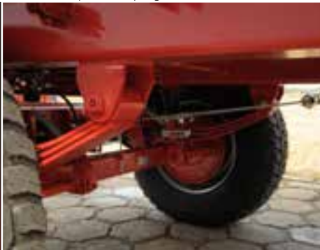
Solid axles on parabolic springs
