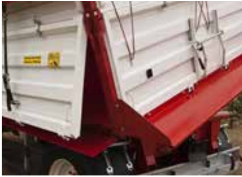
Chute over the entire width of the trailer
