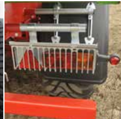
Rear lamps with protective grating
