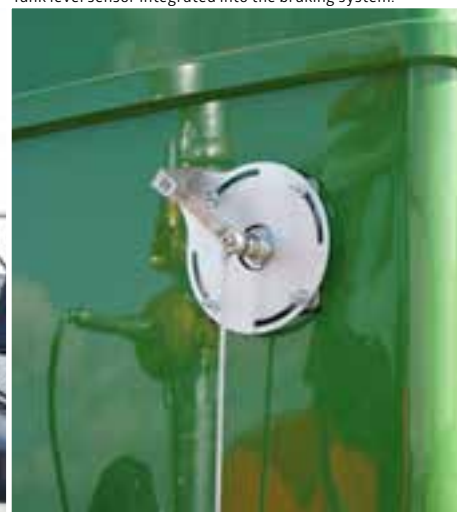
Tank level sensor integrated into the braking system.
