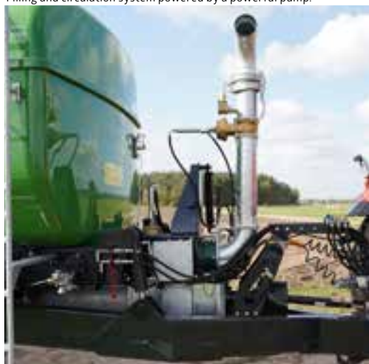
Filling and circulation system powered by a powerful pump.
