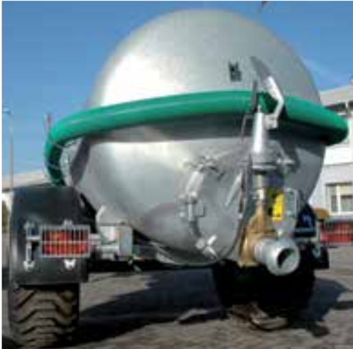
Drain port at the lowest point of the tank
