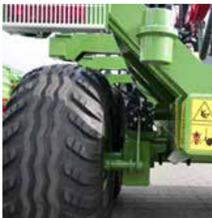
Tandem type suspension with 2 trailing arms and fixed axle shafts equipped with drum brakes
