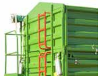
Ladders and operator's platform on the front sidewall for easy access to loading box and rolled canvas cover. Two cylinders for three side tipping system- rear 470, on the sides 450
