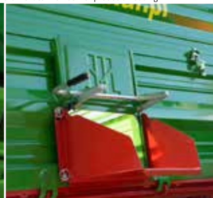
Grain chute with lock for precise unloading
