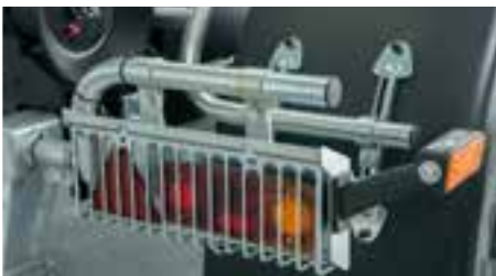
Rear lamps with protective grating
