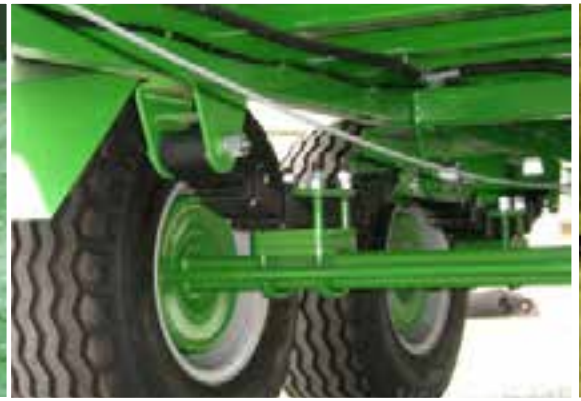
Tandem suspension on leaf springs
