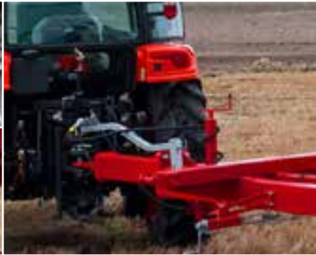
T654/2 - Rigid drawbar to connect to the upper hitch of the tractor
