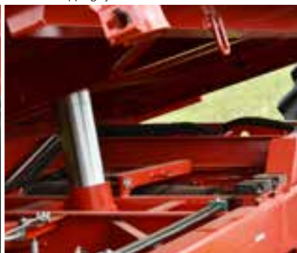
Three side tipping system with cradle
