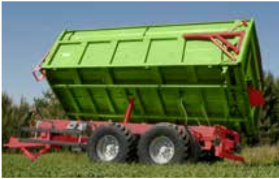
Tipping to the right side at an angle of 45 degrees on T669/1 trailer.
