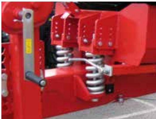
Suspended drawbar with steel springs
