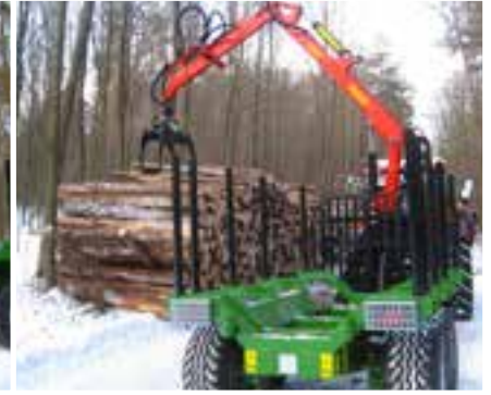
Hydraulically sliding rear frame with columns
