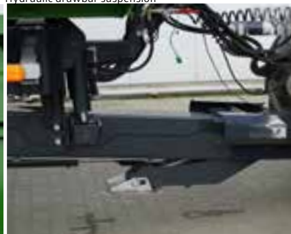
Hydraulic drawbar suspension
