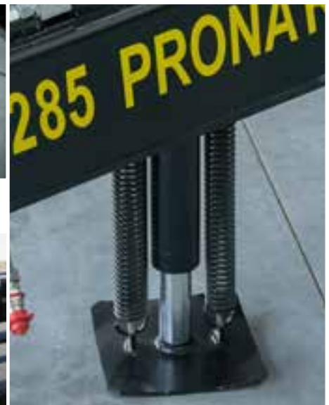
Drawbar support: hydraulic straight leg with cut-off valve
