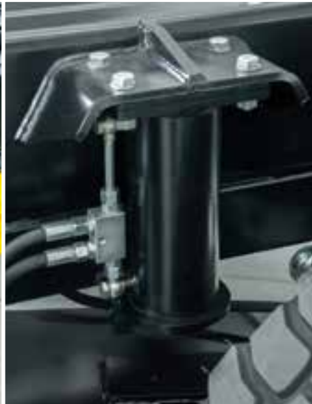
Hydraulic blocking system of the trailing arm (suspension)
