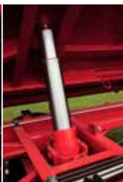
Telescopic servo-motor of 3 side tipping system
