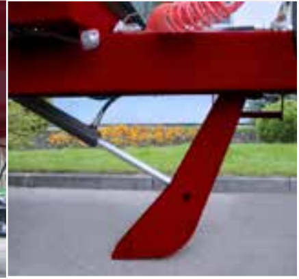
Drawbar support: hydraulic scissor - type leg (T679/2)
