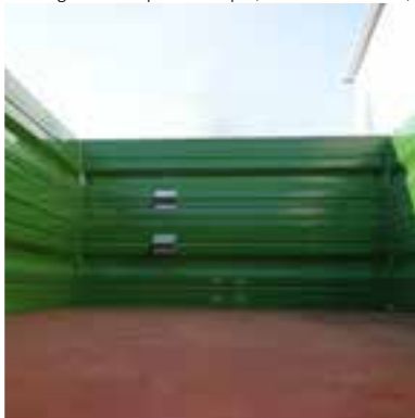
Loading box of trapezoid shape ( 50 mm wider rear ) Grain chute with lock
