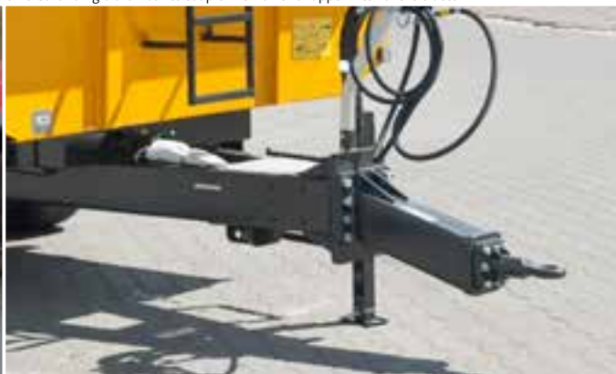
Universal and rigid drawbar to couple with lower or upper hitch of the tractor
