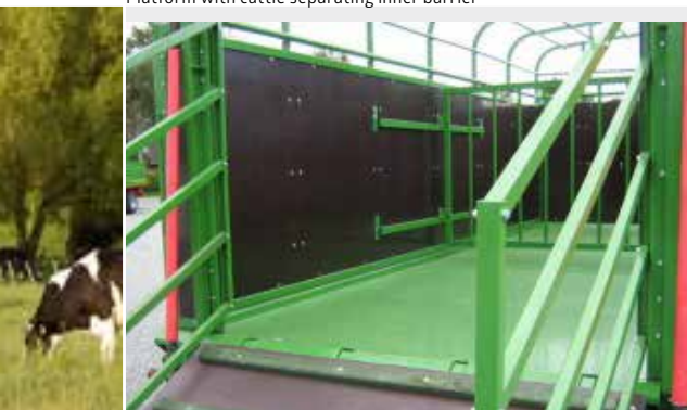
Platform with cattle separating inner barrier
