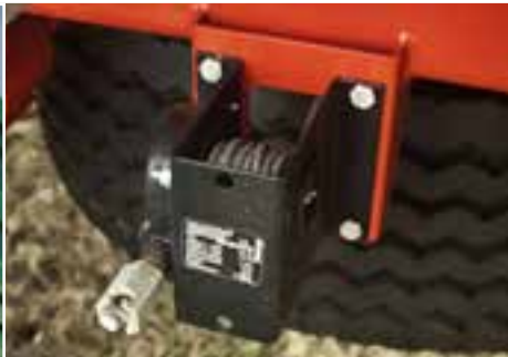
Spare wheel winch under the chassis
