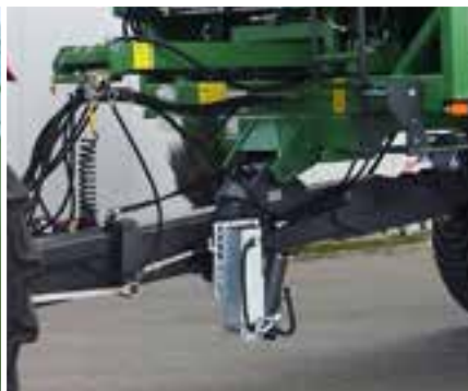
Axles with active steering
