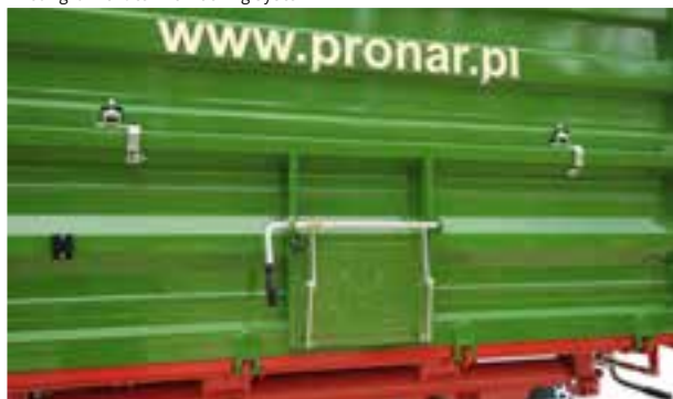
Rear grain chute with locking system
