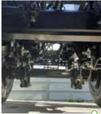
Tandem suspension with 4 parabolic springs
