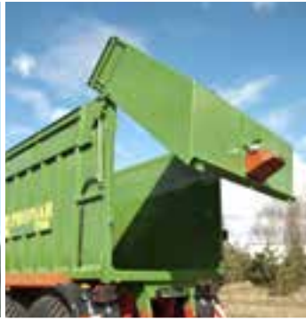
Hydraulic tailgate with automatic blocking system
