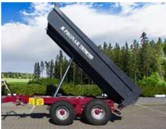
Hydraulically driven rear flap opened downwards
