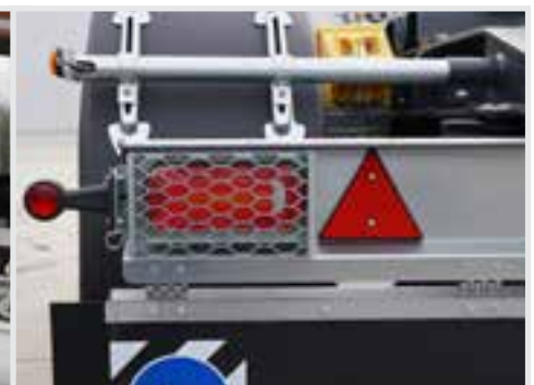
Rear lighting counter - (metal mesh cover).
