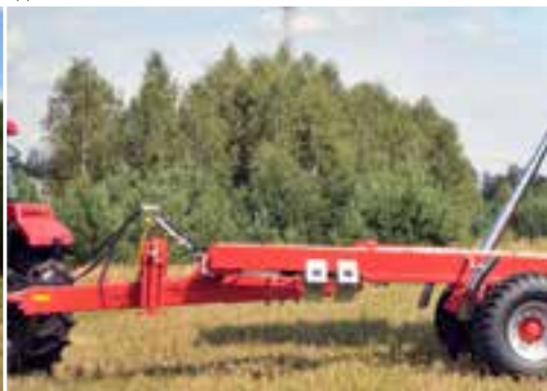
T700 - Universal rigid drawbar suspended with springsteel feather and height adjustment. Possibility to connect with the lower or upper hitch of the tractor
