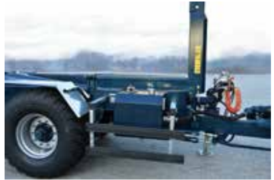
Central hydraulic system with own oil tank
