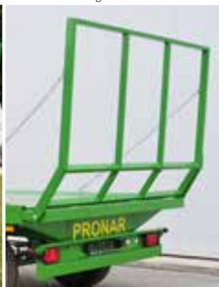
T022M rounded edges of side ladders
