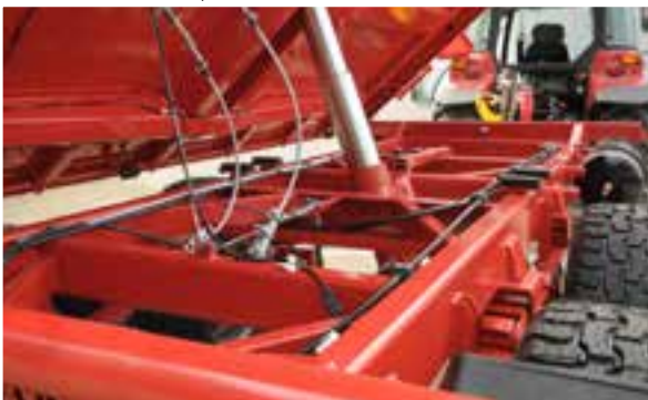
Chassis made of closed profiles
