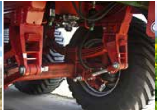
Tridem suspension on 6 parabolic springs
