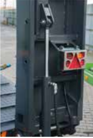
Mechanically lowered ramps
