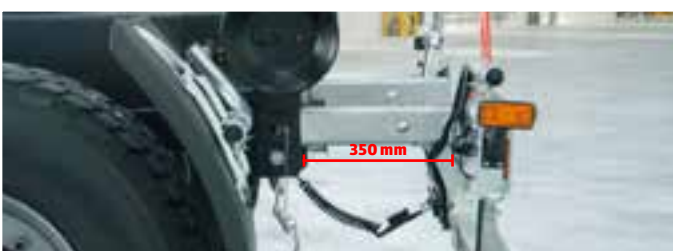
Rear bumper with manual setting in different positions (depends on length of the container)
