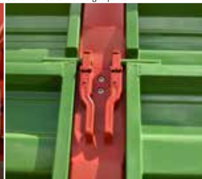
Solid wall locks with forged parts
