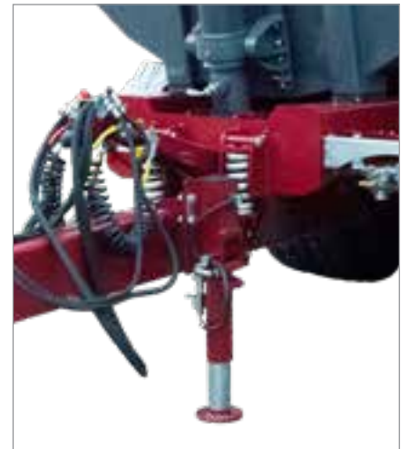
Hydraulic foldable drawbar support with cut off valve (optional)
