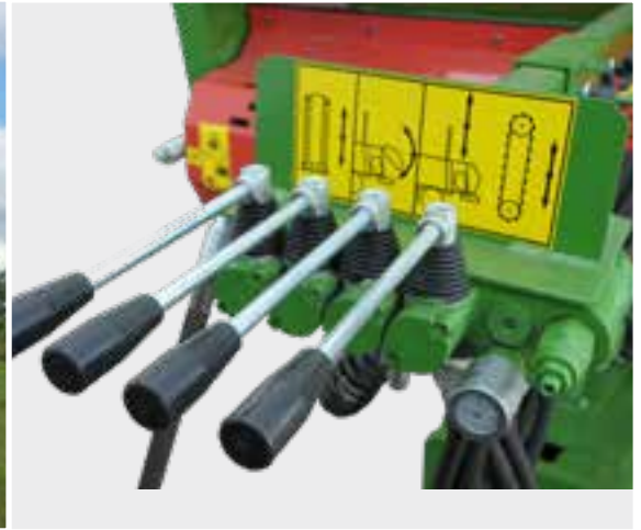
Spreader N262/1- hydraulic conveyor drive
