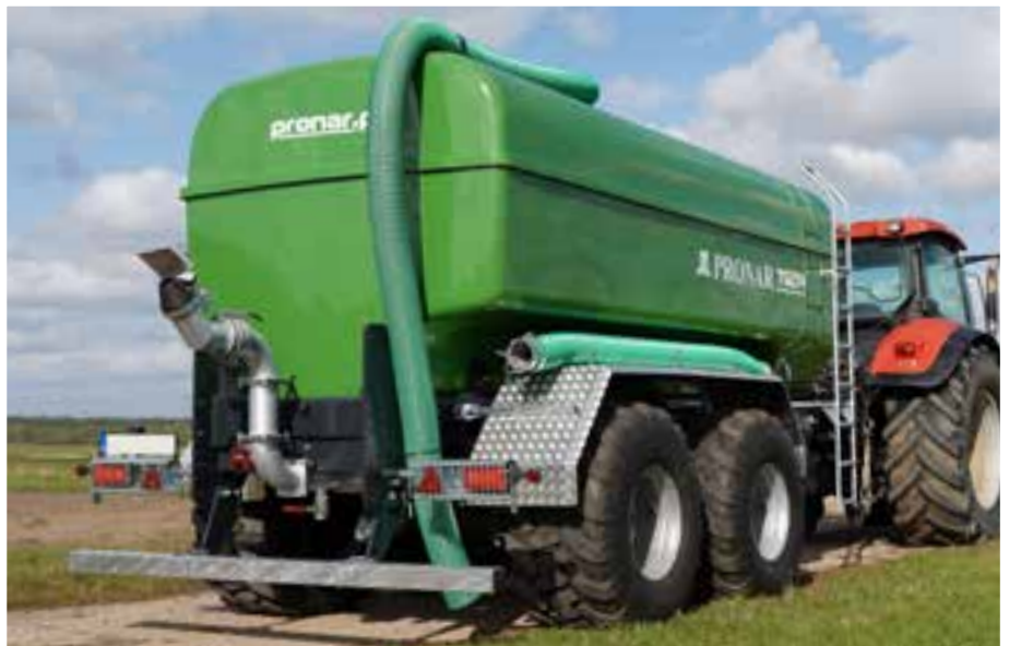
Lower Center of gravity compared to slurry tankers made of steel, which results in higher stability of the tank.
