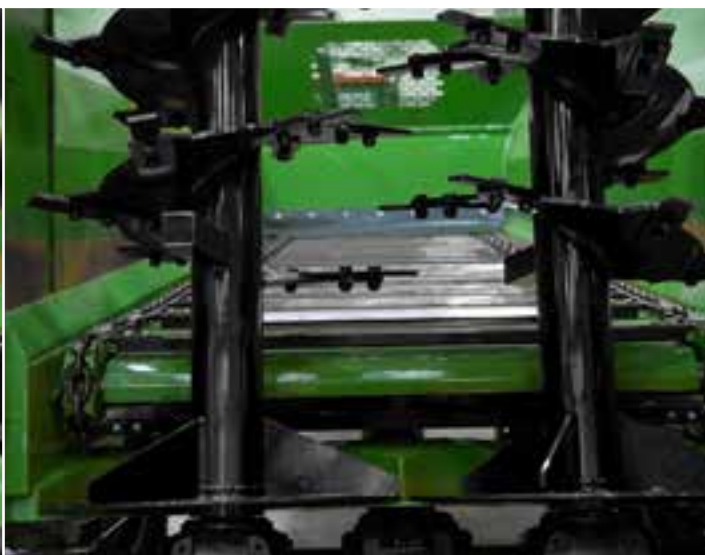
Spreading adapter with 2 vertical beaters of 1600 mm height
