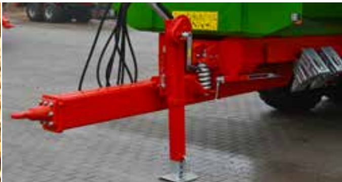
T669XL - Universal drawbar with steel springs and height adjustment. Possibility to connect with the tractor's lower or upper hitch (without approval)
