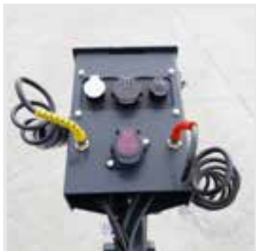
Junction box for electrical and pneumatic systems.
