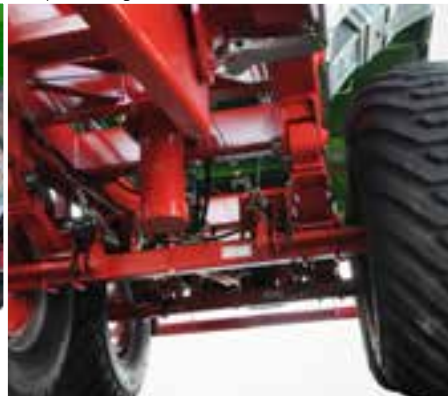
Strong and robust chassis on parabolic springs facilitates transport in rough terrain
