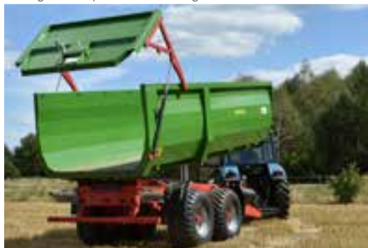
Loading box with profiled sides, strengthened with ribs
