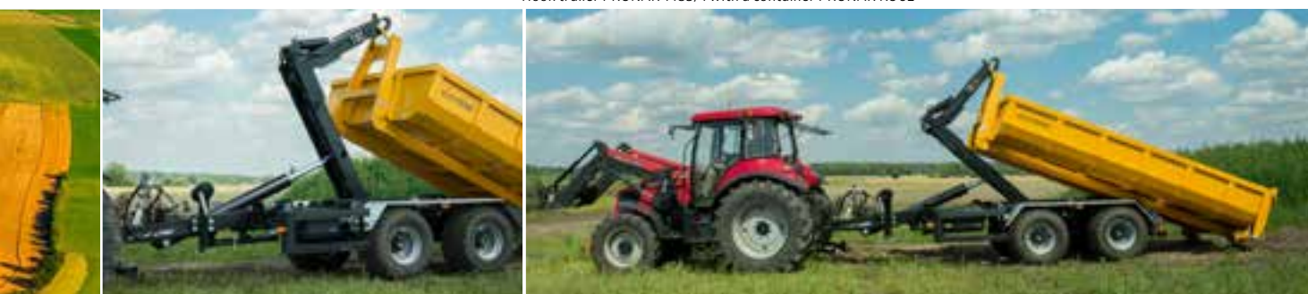
Hook trailer PRONAR T185/1 with a container PRONAR K002
