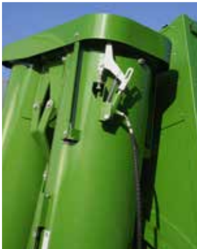
Transport cover for the interior of the 2 segment auger
