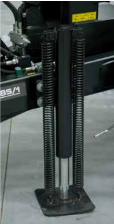
Drawbar support: hydraulic straight leg with cut-off valve
