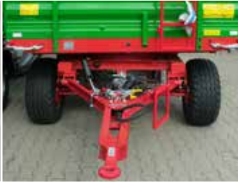
V or Y type drawbar with 40 towing eye
