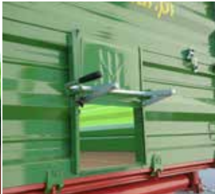
Loading box of trapezoid shape ( 50 mm wider rear ) Grain chute with lock
