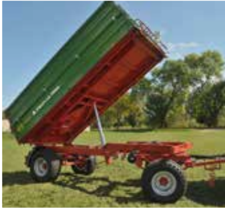
Loading case with universal system of sidewall opening and trapezoid shape of the loading box ( rear 50 mm wider than front)
