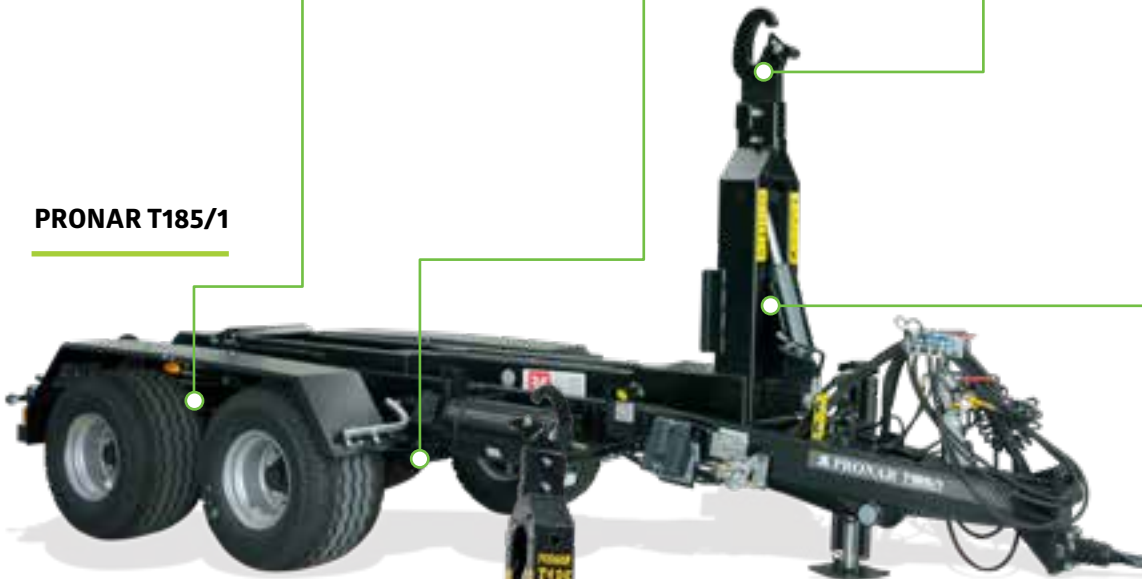
Rear bumper with setting in two positions (slid lights) 340 mm and 680 mm
