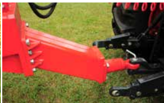
Universal rigid drawbar to connect with the lower or the upper hitch of the tractor
