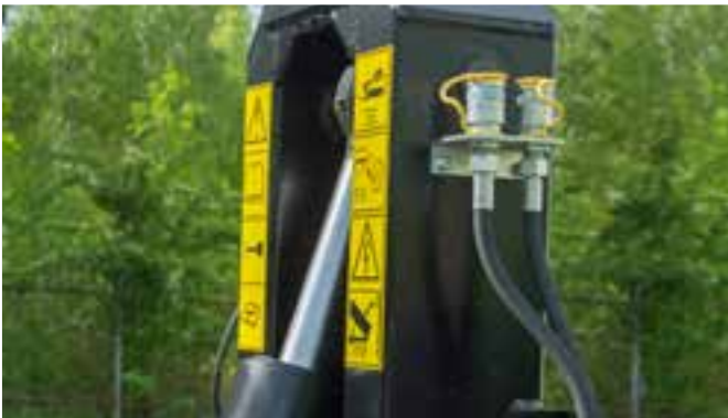
Additional pair of hydraulic outlets located on the hook
