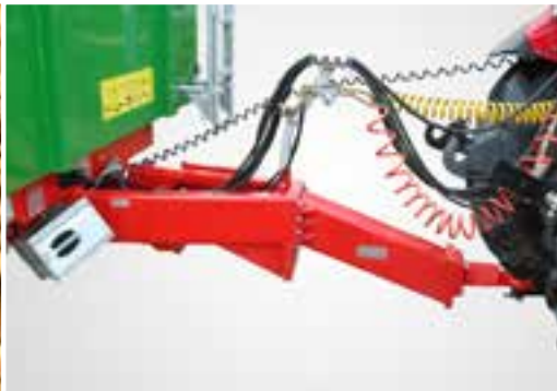
Universal drawbar to connect with upper and lower hitch of the tractor
