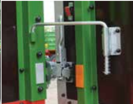
Sidewall blockade protects against self-closing and damage
