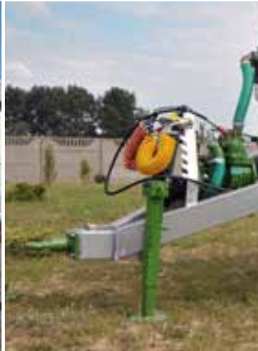
Drawbar support- simple telescopic
