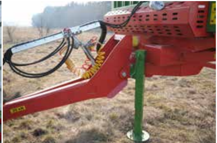
Drawbar support telescopic mechanical straight leg
