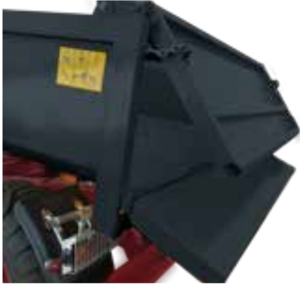
Hydraulically driven rear flap with height 450 mm (T679/2), opened downwards and swinging tailgate with right side opening (optional)
