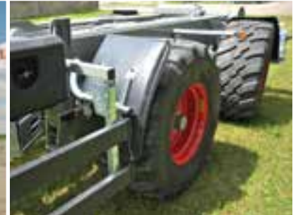
Passively steered rear axle on T285/1
