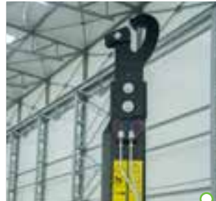
Pair of hydraulic sockets on the hook
