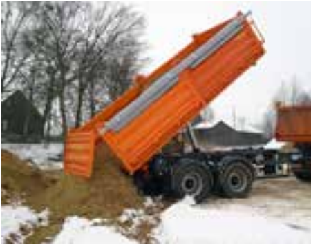
PC2100 – unloading of the trailer. Rear raised wall opened automatically when tipping
