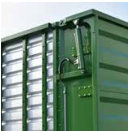
The rear wall lifted hydraulically, loading case adapted to be assembled with metering rollers.
