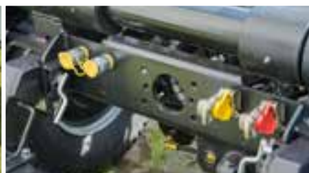
Pairs of hydraulic and pneumatic outlets at the back
