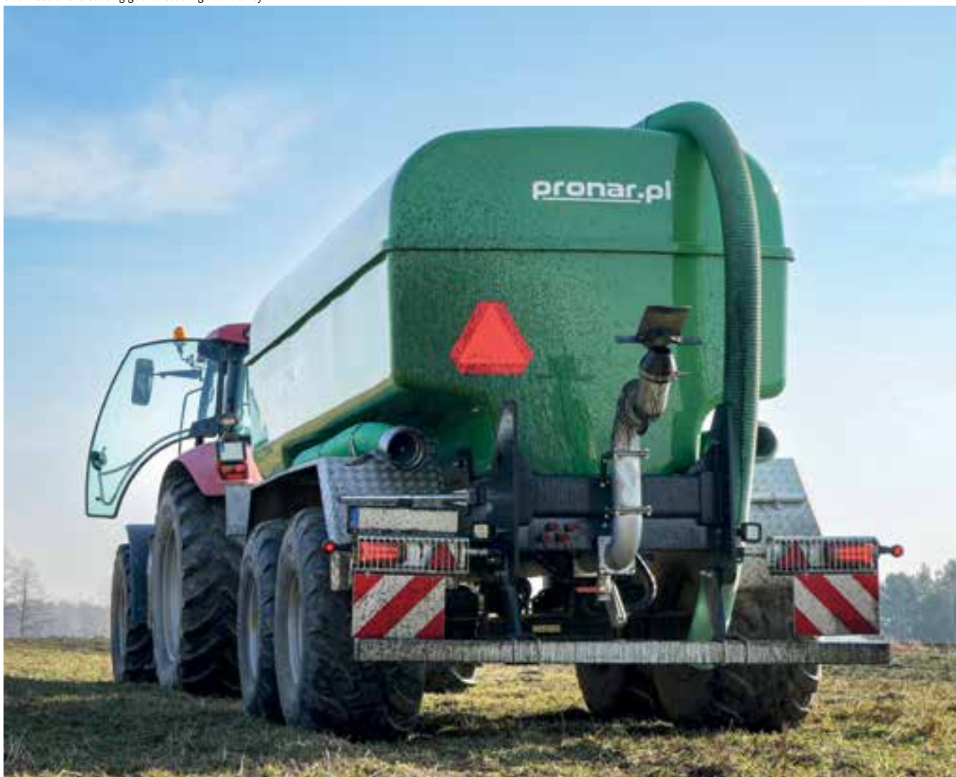
Two suction pipes 6" (Perrot quick couplings) each 5 m long and a 6" vent pipe
