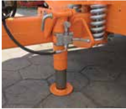
Sprung drawbar and hydraulic support leg
