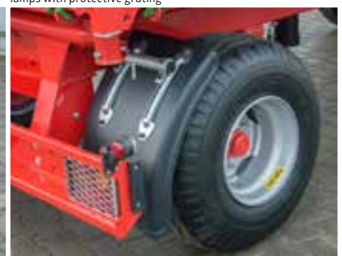
T672 eco - Plastic mudguards - rear mudguards and rear lamps with protective grating
