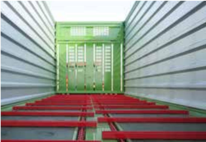
Wooden floor board with metal rails of conveyor's chains
