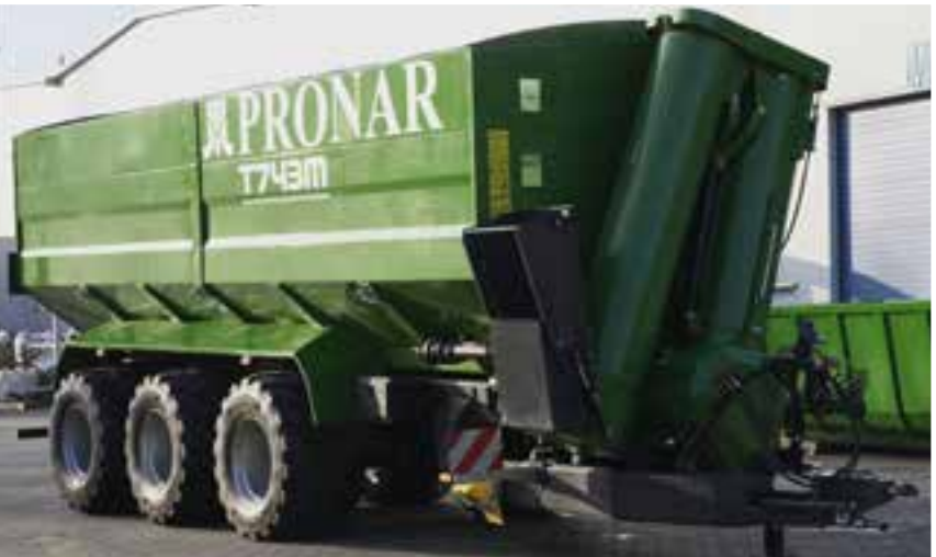
Shell cargo box with profiled walls, with additional vertical stiffeners and bolt-on extensions
