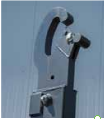
Trailer hook with automatic container lock
