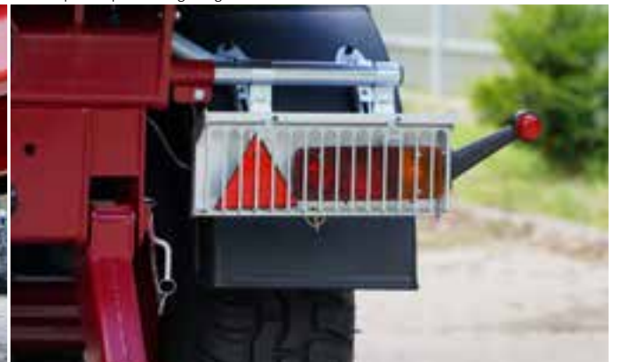
Rear lamps with protective grating
