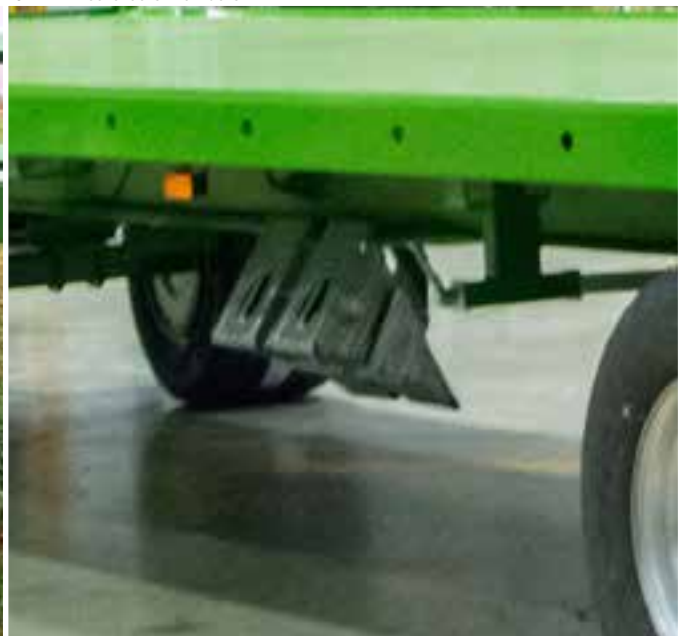
T027M - Wheel chocks with racks
