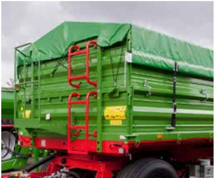
Tarpaulin with frame. Operator's platform to handle tarpaulin
