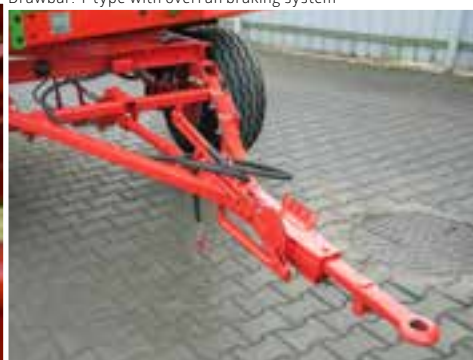
Drawbar: Y type with overrun braking system
