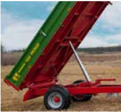
Three way tipping system with telescopic cylinder and hinged suspension
