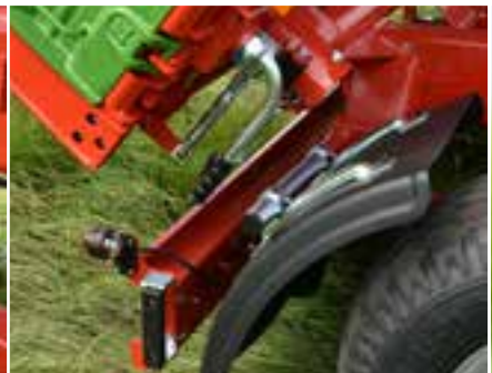
Three side tipping system of loading box
