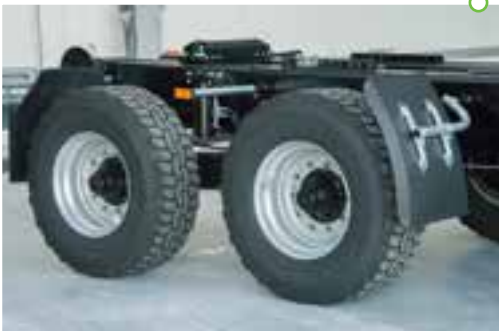
Trailing arms (rigid suspension)
