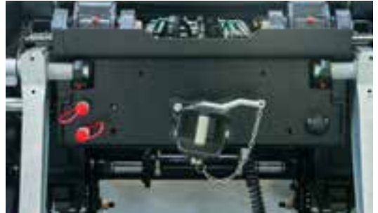
Pair of hydraulic sockets, electric socket and rear hitch at the back
