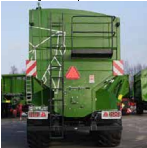
Folding ladder on the rear wall and ladder inside the cargo box, balcony
