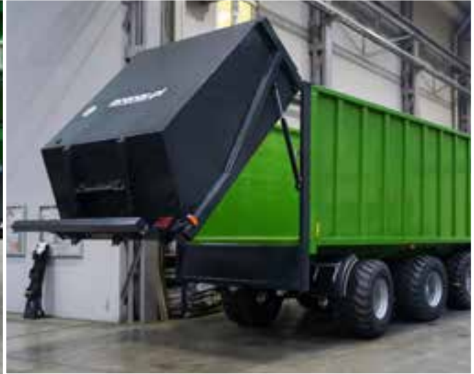
Hydraulically driven tailgate with automatic blocking system
