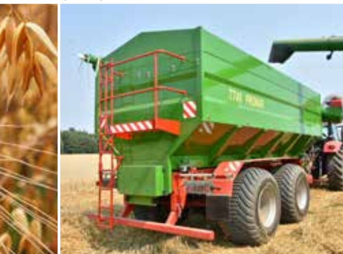
Operator's platform on rear side with foldable ladder
