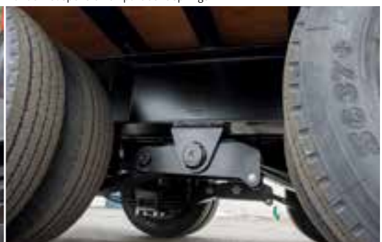
Tandem suspension on parabolic springs
