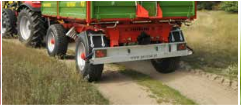
Strong rear bumper with LED lights with bars protecting against damage
