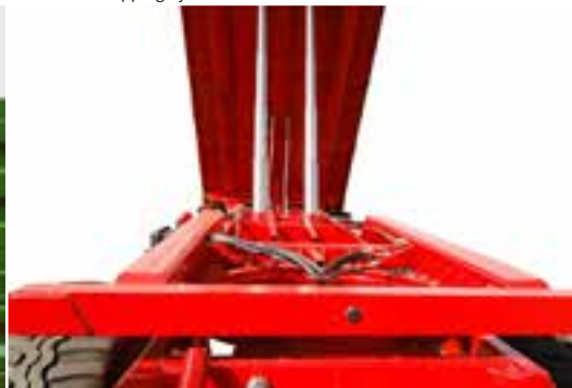
Three side tipping cylinders - rear 470, 450 on the sides
