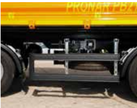
PB2100 – spare wheel, optionally equipped under chassis of the trailer
