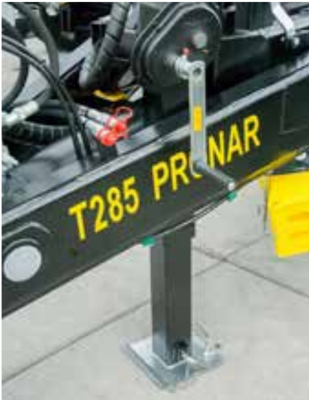
Drawbar support: telescopic supporting leg with two-step gear
