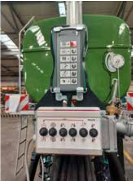
Remote control for slurry tank operations. Steering box for external adapter functions
