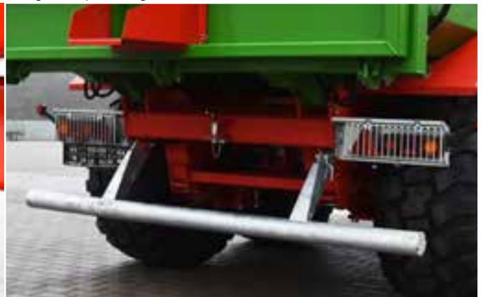
Rear lights with protective grille
