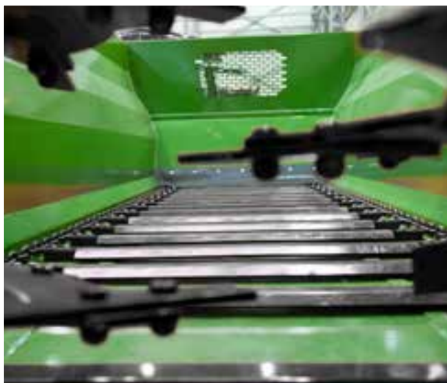
Chain conveyor with two 14mm chains of high quality steel, with hydraulic drive and stepless speed regulation
