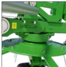
● maintenance-free gearbox, lubricating grease
