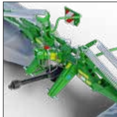
• central suspension bilateral terrain copying range +18°-16°
