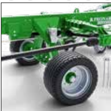
• 2 wheels on the axle braked
