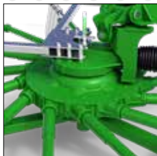
• carousel gearbox - greased
