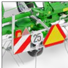
• warning signs with road lighting
