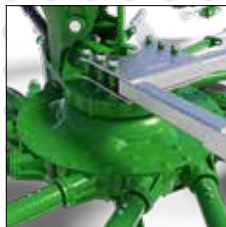
● carousel gearbox - greased
