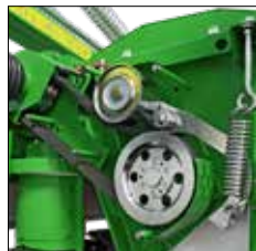
• belt drive conditioner, automatic winding
