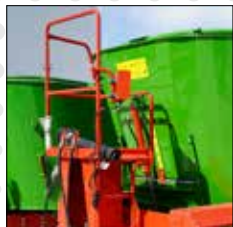
• platform with steps and a protective barrier
