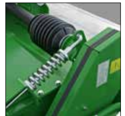
● automatic tension of the conditioner shaft drive
