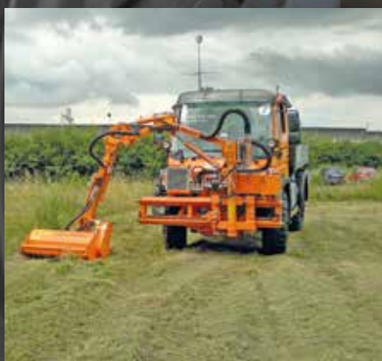
MULTIFUNCTION ARM WWP500U MOWING HEAD GK110
