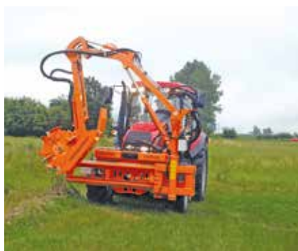
WWP600 with GO800 ditch digger. Long reach fits perfectly for desludging
