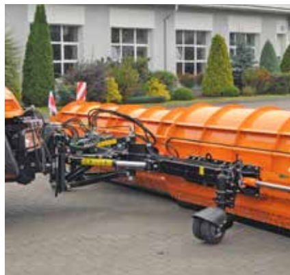
Mounting – DIN type A municipal plate
