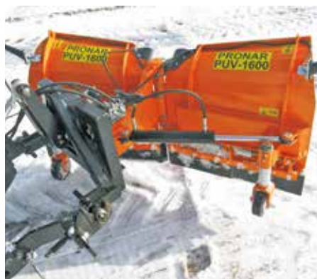
Electrohydraulic adjustment of the working angle
