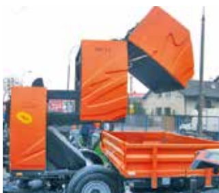
Hydraulic hopper dumping system
