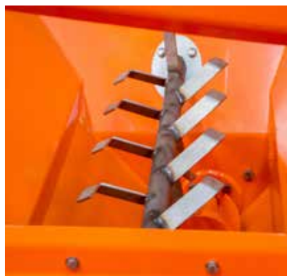
Additional mixer facilitates aggregate breaking
