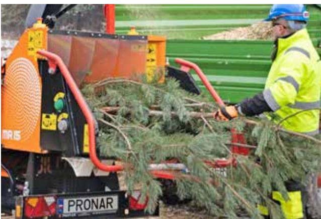
Loading ramp and safety bar
