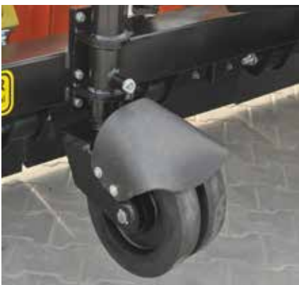
Optional adjustable support wheel
