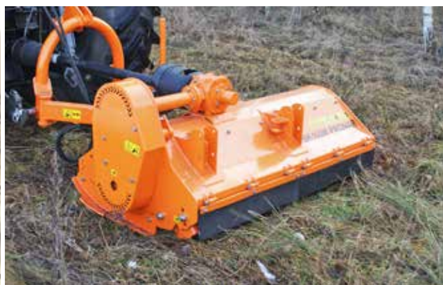
Intersecting gear and belt drive - overload protection of the mower
