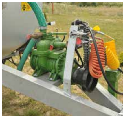
Rotary vane vacuum pump
