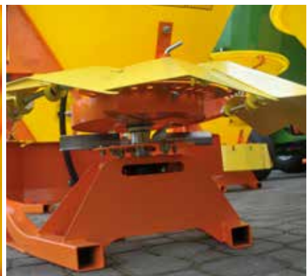
Stainless steel spreading disc
