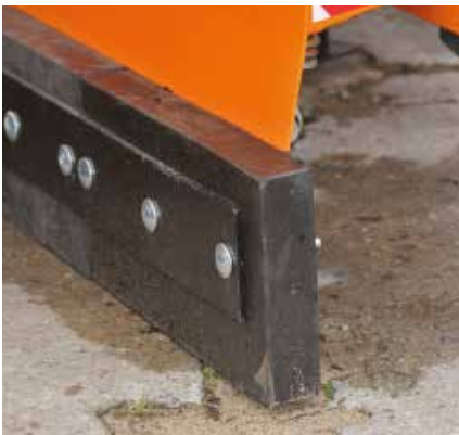
Rubber blades with shock absorption
