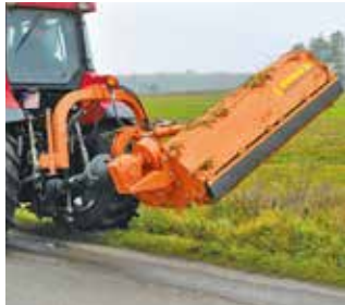
Hydraulic adjustment of the working angle
