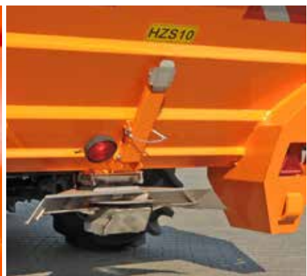
Stainless steel spreading disc
