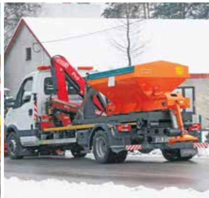
Capability of aggregation with a hook loader
