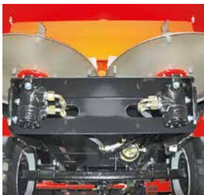
2 stainless steel spreading discs
