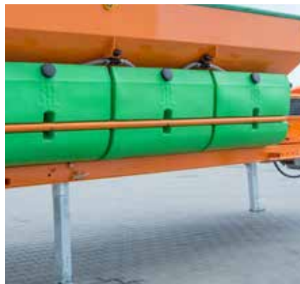
RORO (Roll-on / Roll-off ) system for easier loading of PT70 spreader on the carrier platform
