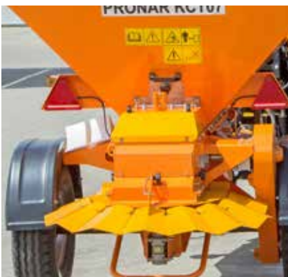
Covers for setting spreading width and limit scattering
