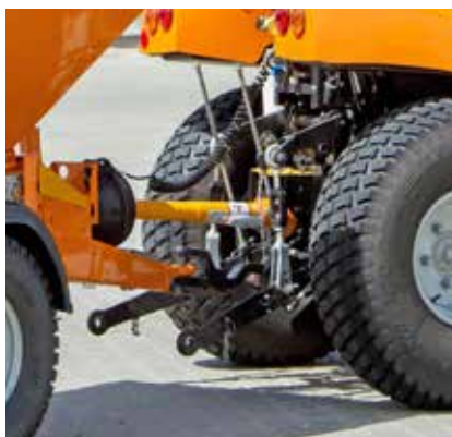
PTO drive for tractors without hydraulic system
