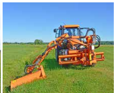
WWP600 boom with GK mowing head
