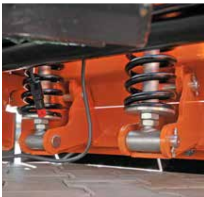
Spring shock absorption of the blade
