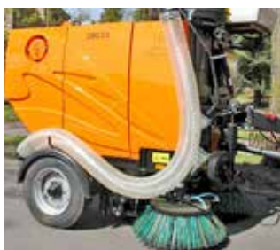
Side attachment for collecting leaves
