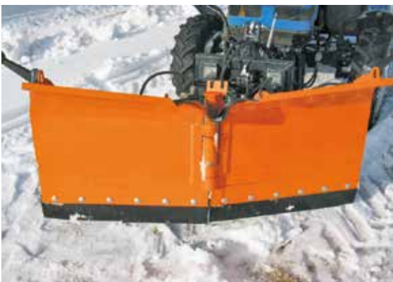
Working at an angle of 30°
