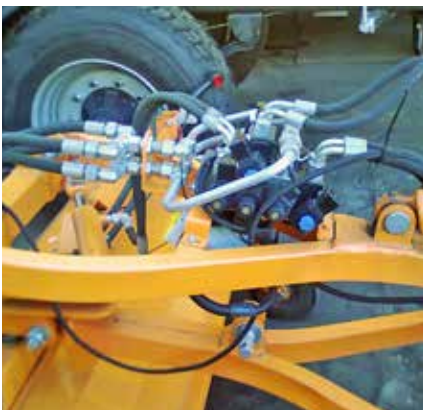
Hydraulic brush rotation \pm 30^\circ
