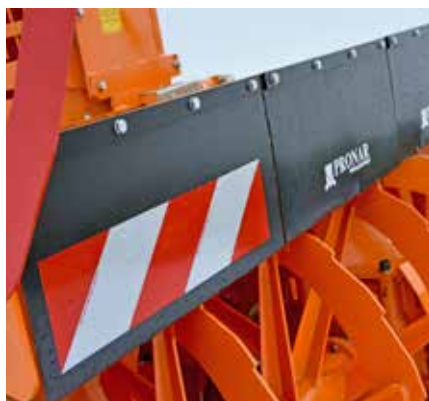
Rubber covers protect against dusting
