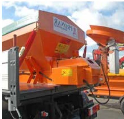
Tiltable spreader unit
