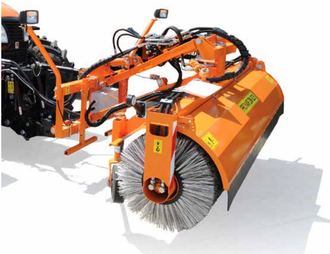
Hydraulic brush rotation \pm 30^\circ
